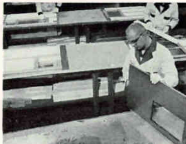
Foam and structural parts being assembled on panel skins
