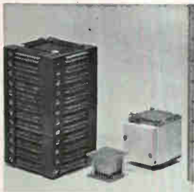
Storage capacity of conventional stack (left) is provided by MICROSTACK unit (center). Complete unit, surrounded by temperature-controlled circuit and insulation is at right.
