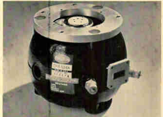
FIG. 7—Injected-beam backward-wave electronically tunable oscillator type QK 634A
