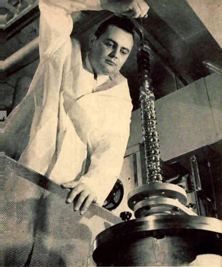
Engineer lowers shish-kebab of approximately 100 Nuvistors into an exhausting and heat-sealing machine. Tubes are subjected to 1,800 F during this operation
