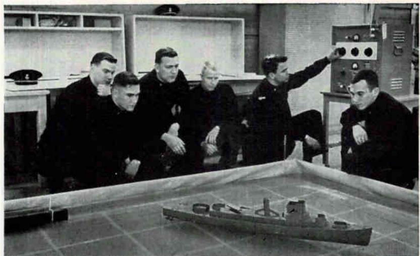
Transistorized radio receiver built into ship model hull allows naval reserve officer trainees at Cornell to study ship-handling problems. Models are controlled by equipment (right). Scaled-down vessels cost $2,000 each
