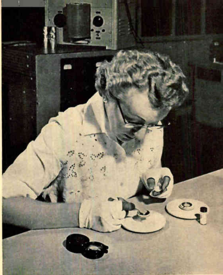
FIG. 1—High vacuum thermionic converters having an output of one watt at \frac{1}{2} to \frac{3}{4} volt direct potential
