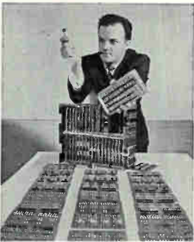
Cube of electronics in engineer's right hand fits on modular card that does as much work as all 23 conventional printed circuit boards spread out on table
