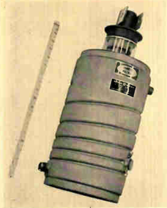
FIG. 8—Ignitron 7151 con switch 4,800 Kva (two tubes in inverse parallel) at potentials of 250 to 600 v
