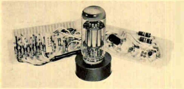
FIG. 6—Burroughs Beam-X decimal electronic switch and one of its transistorized circuit modules
