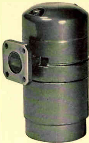
FIG. 7—Reflex klystron for 34,000 to 37,000 Mc
