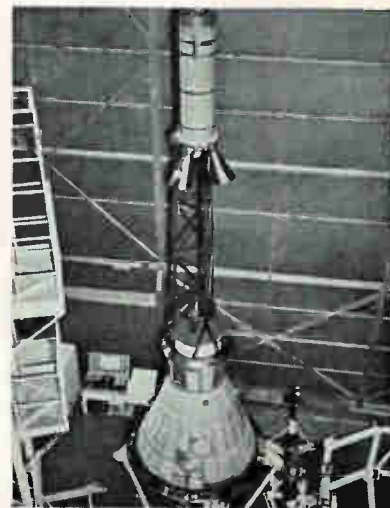
First Project Mercury man-in-space capsule to be delivered to NASA at Wallops Island, Va., is shown here before it was shipped from the St. Louis plant of McDonnell Aircraft. Pylon atop capsule incorporates escape system
