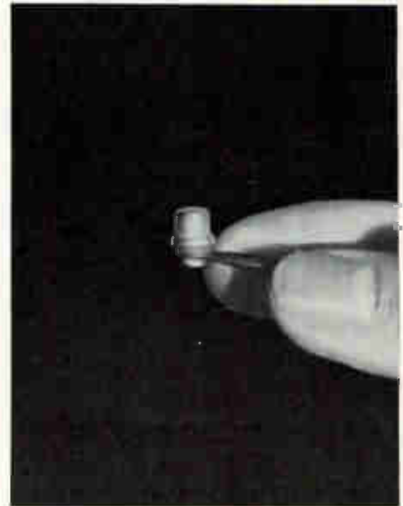
First practical diode for amplifier, shown here held by tweezers, was jointly developed by A. E. Bakanowski and A. Uhlir.
