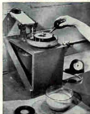
Base-plating equipment, showing arrangement of plating chambers (foreground) and frequency scanning monitor
