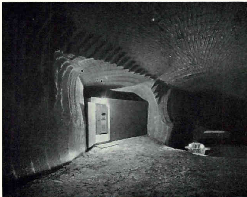
Subsurface propagation of electromagnetic waves is being studied by Space Electronics Corp., Glendale, Calif., with the aid of this experimental station buried in a mine shaft in the Mojave desert. Company recently received USAF contract (ELECTRONICS, p 11, Mar. 4) to study feasibility of burying components of a communications system deep within the earth's crust
