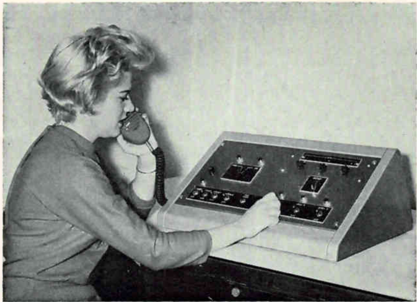
Operator sets digit switches to identify zones and then determines type of signal
