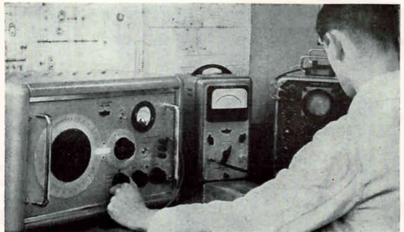
Precision oscillator being used for alignment of filters with sharp resonance curves
