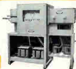
LINDBERG SOLID DIFFUSION FURNACE: Preheat chamber 21" long with two zones of control—maximum temperature 900°C. (1652°F.). High heat chamber 16" long with two zones of control, maximum operating temperature 1300°C. (2372°F.).
