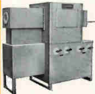
LINDBERG SOLID DIFFUSION FURNACE: Preheat chamber 21" long with two zones of control—maximum temperature 900°C. (1652°F.). High heat chamber 16" long with two zones of control, maximum operating temperature 1300°C. (2372°F.).
