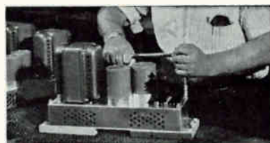
Nuts are run down on prethreaded studs
