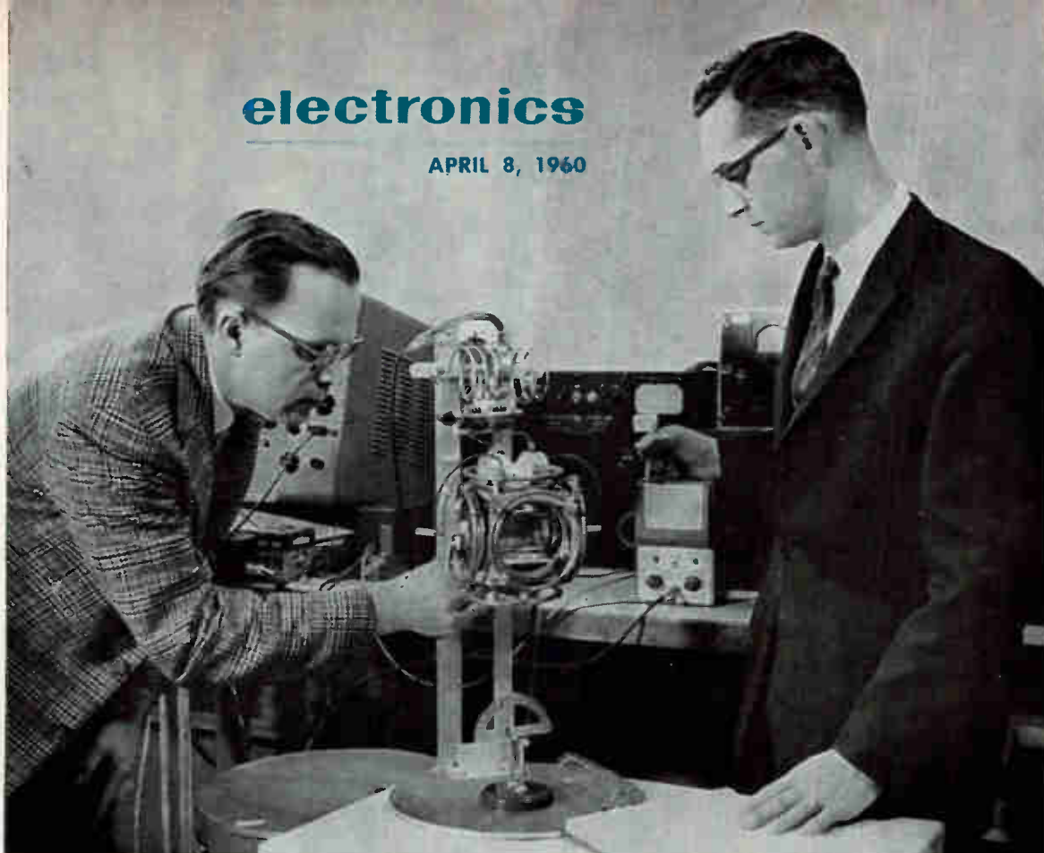
During a test run, the lamp-cell rig is enclosed by container at lower left. Spectral lamp is mounted above absorption cell. Although coil pairs can produce two mutually perpendicular fields, only one pair is used in Fig. 1 setup
