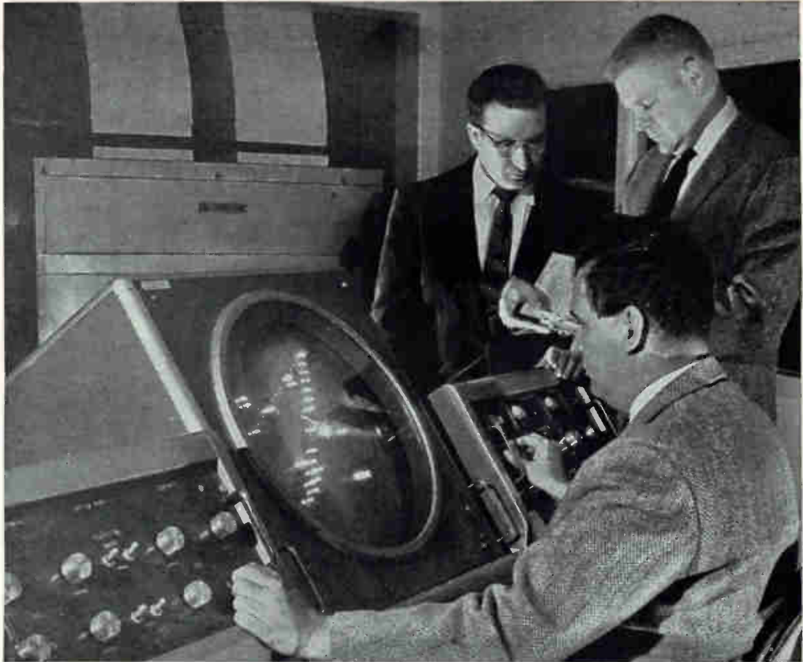
Charactron display in NAFEC's computer laboratory shows movements of 50 simulated aircraft
