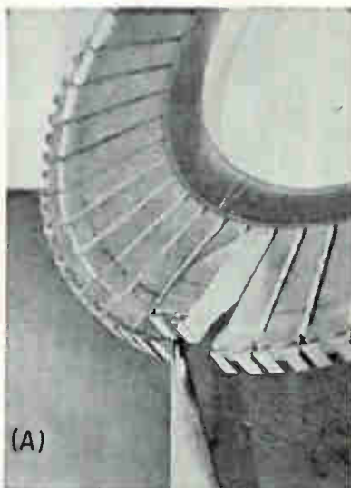
Pantographic element greatly extended (A). Cathode-filament support ring with one of the 96 filamentary cathode strands in place (B)
