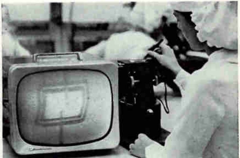
Closed circuit television system is used to monitor quality during the production of mesa transistors at Motorola's Semiconductor Products Division, Phoenix, Ariz. The system enables operators to view the operating area (less in diameter than a human hair) of the devices at about 200 times actual size
