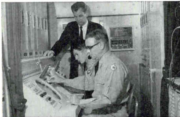
"Vest Pocket Air Defense System" —Hughes mobile digital computer and display unit, linked to a Hughes 3-D scanning radar antenna, assigns enemy targets to missile batteries.
