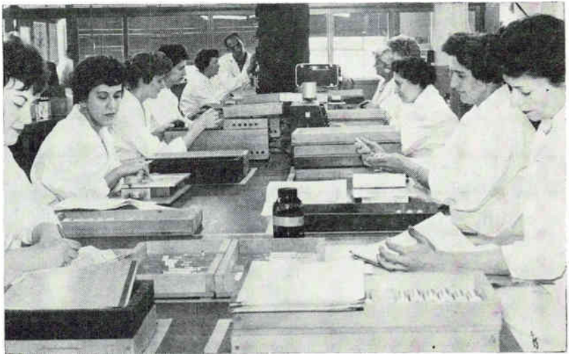
Component inspection line. Each operator performs a separate test. Parts are passed on in corrugated tote trays
