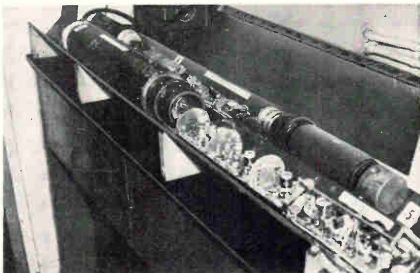
Telemetering hydrophone, such as this one aboard a U. S. oceanographic vessel, is typical of new electronic devices designed for oceanic research
