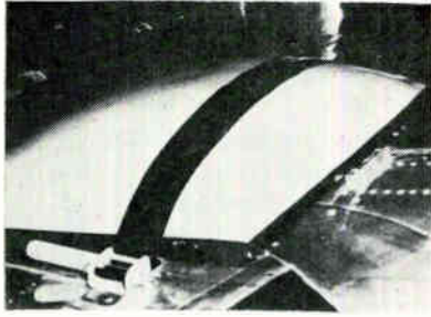
FIG. 2—Crash position indicator is held on aircraft tail by a slim metal ribbon passing through a spring-loaded knife. Extreme tension in trigger wire operates knife
