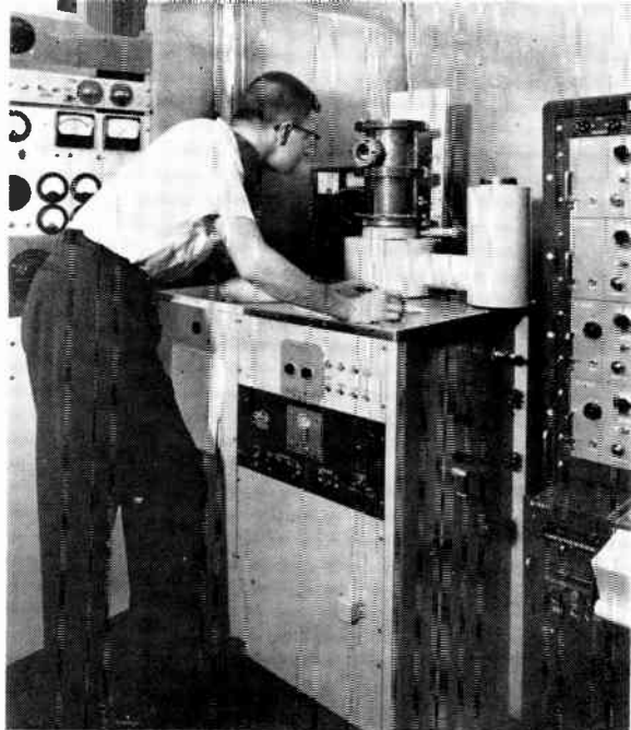
Operator leaning on vacuum portion of a deposition system used in fabricating Microcircuits
