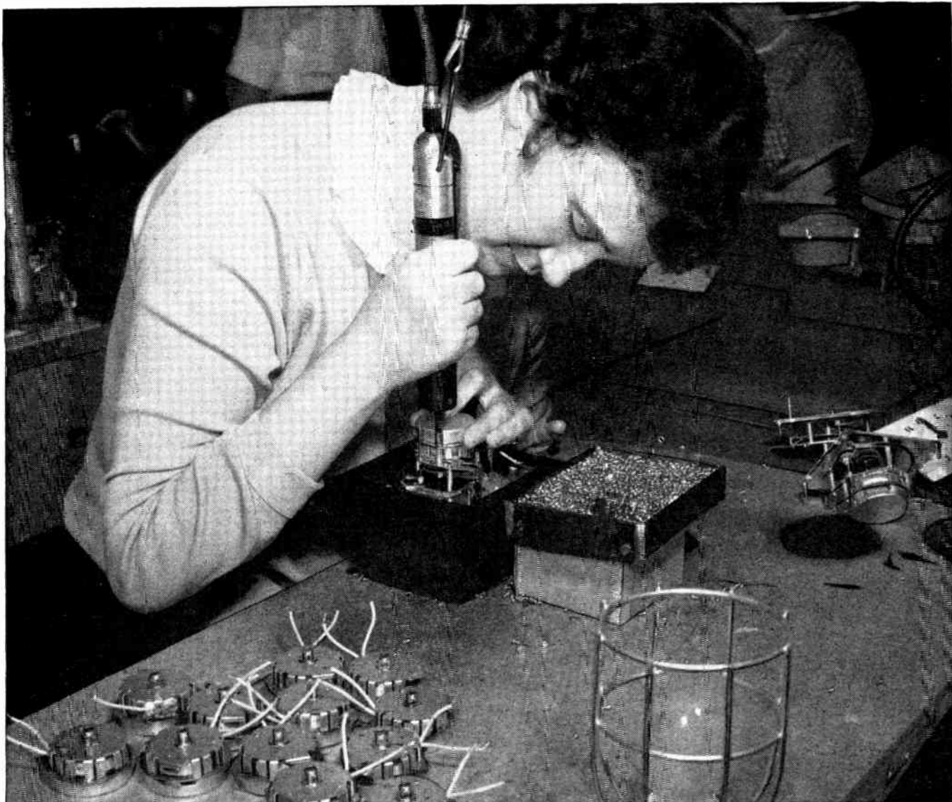
Clock assembly work steps along quickly with Gardner-Denver 12E air screw driver.
