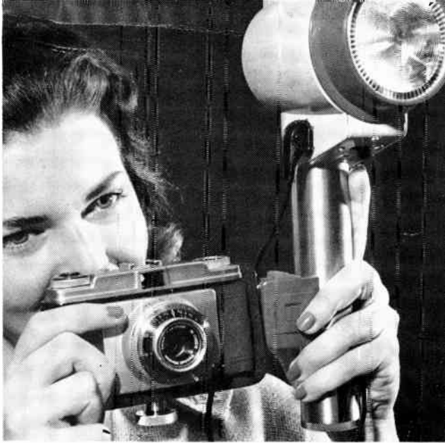
Power for this electronic flash unit is provided by transistorized circuits in lamp head and handle. Device made by Heiland Div. of Minneapolis-Honeywell works off batteries or household current
