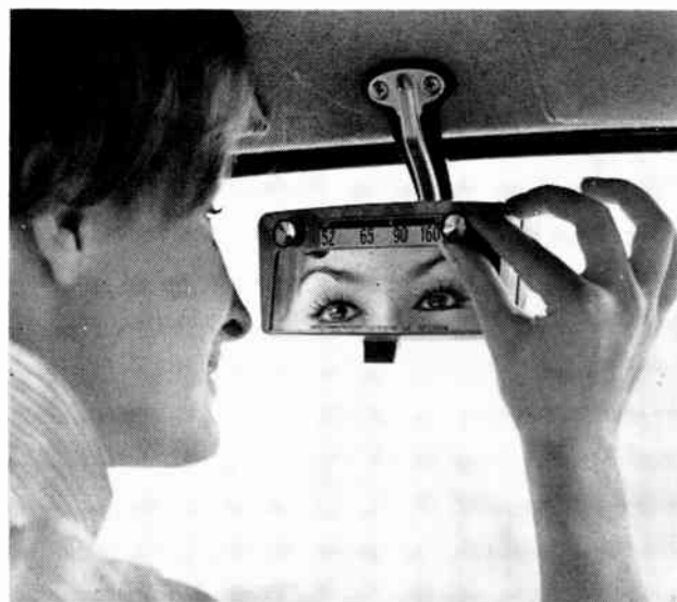
All receiving circuits of the Voxson Vanguard automobile radio are enclosed behind mirror. Transistorized unit is manufactured by Fabbrica Apparecchi Radio E Televisione of Rome
