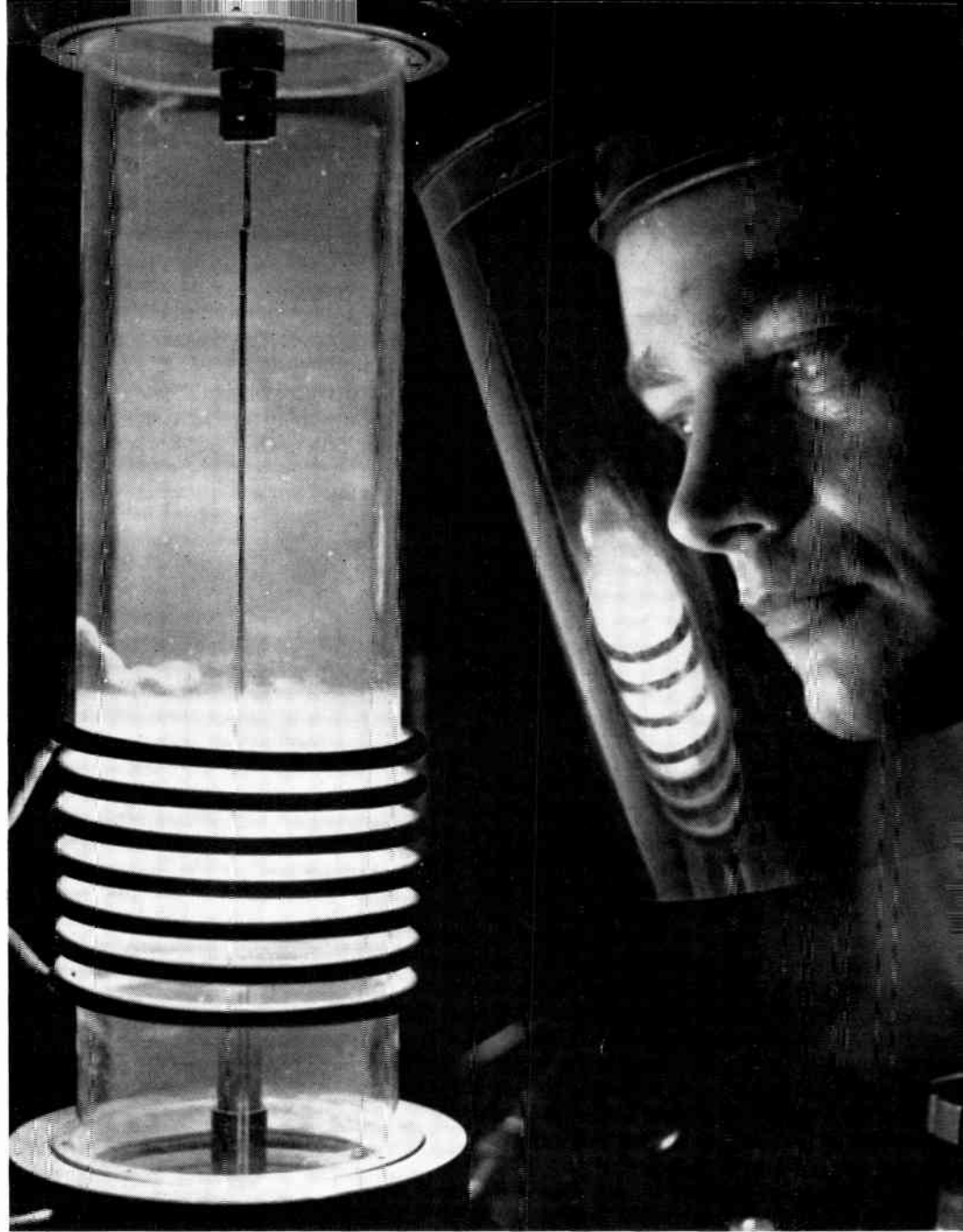
Growing of germanium crystal in ribbon form at Westinghouse Research Laboratories
