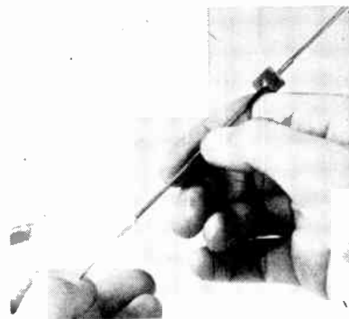
The tool's tube is slid between shielding and wire for about 1 inch
