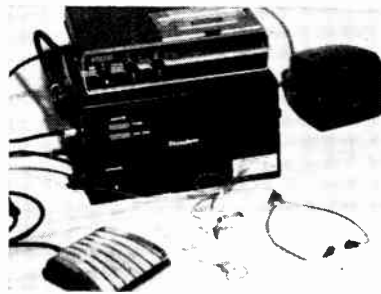
Parts used with transcriber include foot pedal, hearing-aid type receiver, headpiece and loudspeaker
