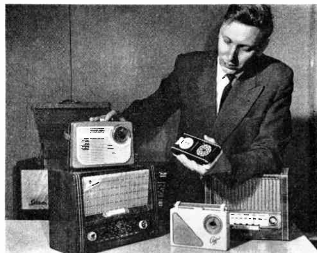
FIG. 5—Portable radios use transistors. Unit in foreground is powered by solar battery on top of case
