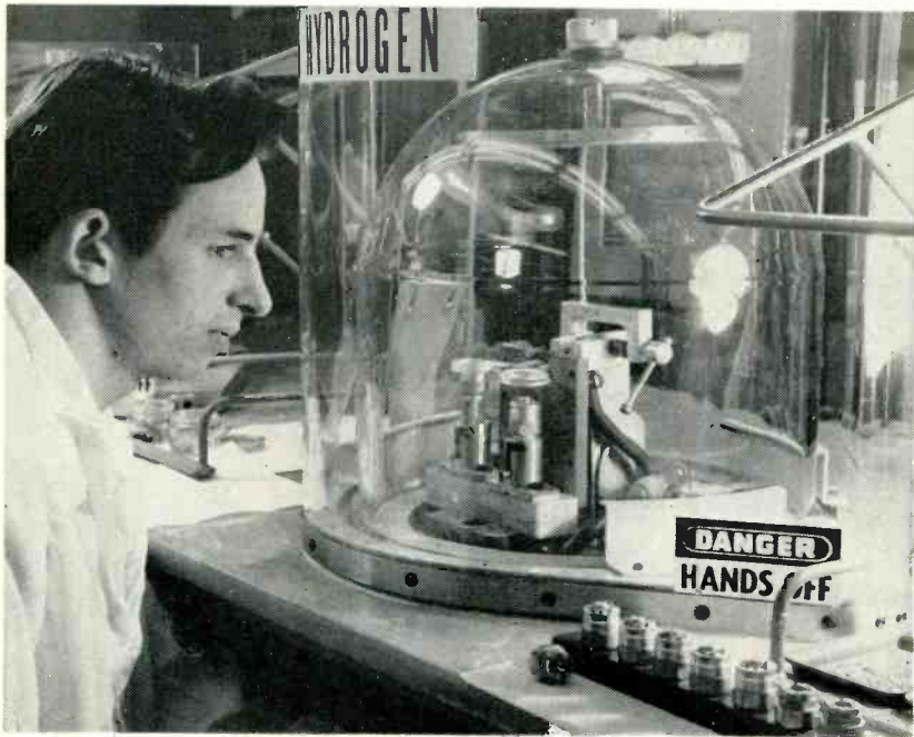
Terminals are soldered into 2 gyroscope pickoff and null adjustment housings. Operation takes 10 seconds at temperature of 400 F
