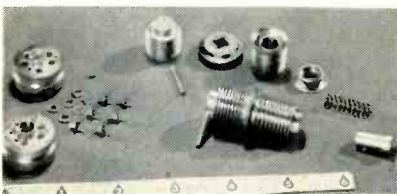
Typical components brazed and soldered in bell jar setup. Parts are shown above assemblies at lower left and right
