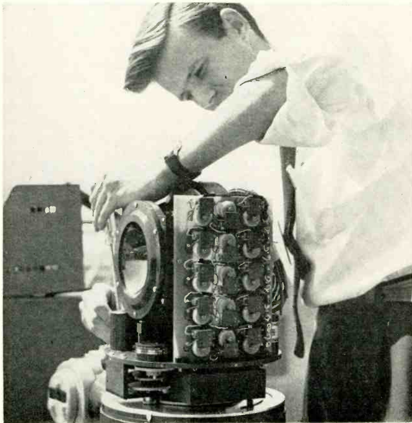
THE FRONT COVER—Closeup of CODES shows some of the parallel-tuned tank circuits
