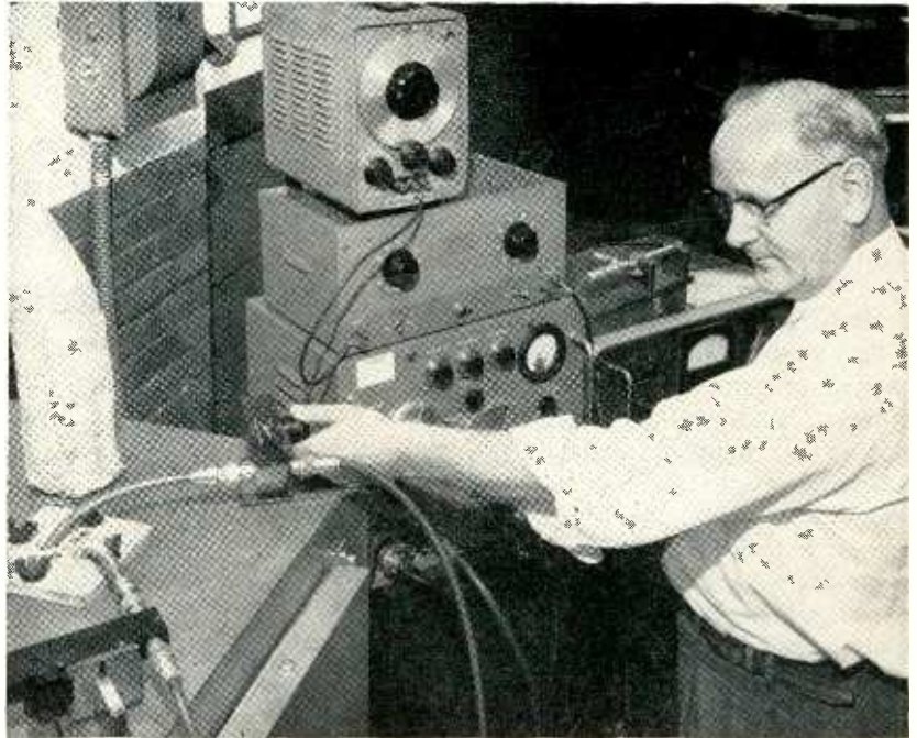
Attenuation values of cable system are being determined at 1,000 F. Cable system has been inserted in oven at left. Impedance transformers are shown at each end of the assembly
