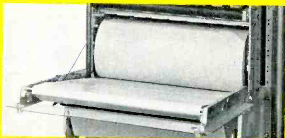
The 504A paper drive gives speeds of from 1 to 250 mm/sec. Electrical speed shift 1 to 250 mm per minute available. Zero weave high precision drive, 850 ft. capacity (heat or electric) 1500 ft. (ink). Front loading, with record fully visible from front.
