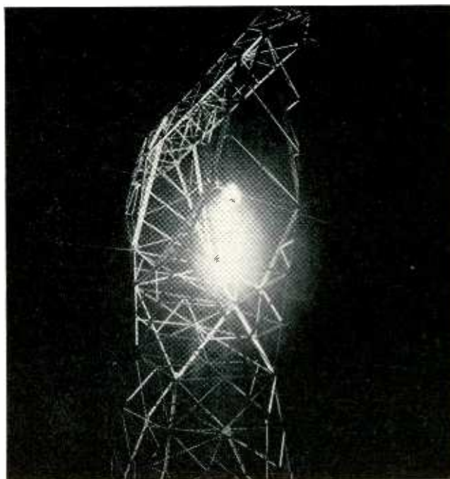
Arcing fault initiated on 345-kv single-phase line at Bonneville Power Administration installation tests operation of frequency-shift power-line carrier used in transfer trip relaying system
