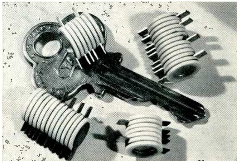
Cathode follower (upper left); plate clamped, flip-flop stage, grid-driven, grounded cathode, bistable multivibrator (upper right); triple in-and gate (lower left) and a second cathode follower (lower right). These correspond to building blocks shown in Fig. 3
