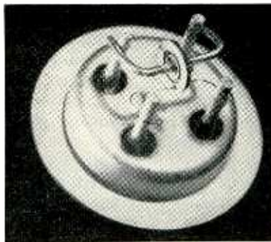
Tetrode with leads applied is bonded to a header
