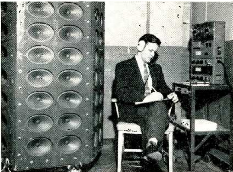
Ear defenders are evaluated at Stromberg-Carlson division of General Dynamics. Under study is the subject's ability to recognize information transmitted to the receivers in various types of ear defenders while working where noise is 122 db. About 100 speakers in single array are used to provide sound for test for U.S. Army Signal Equipment Support Agency. Work is being carried out under subcontract with Lehigh Engineering Associates
