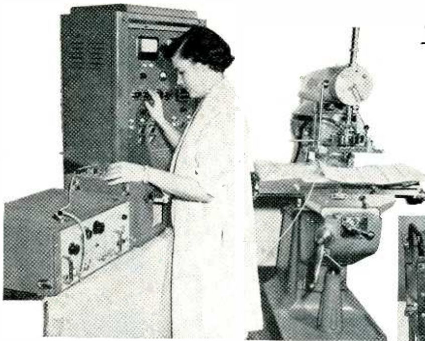
Operator adjusts ultrasonic generator. Transducer is mounted on modified milling machine (right) to give rigid support and to provide accurate positioning. Calibration of focal size and ultrasound intensity is done with precision thermocouple probe. Inset shows typical plug-in coil for low-frequency operation
