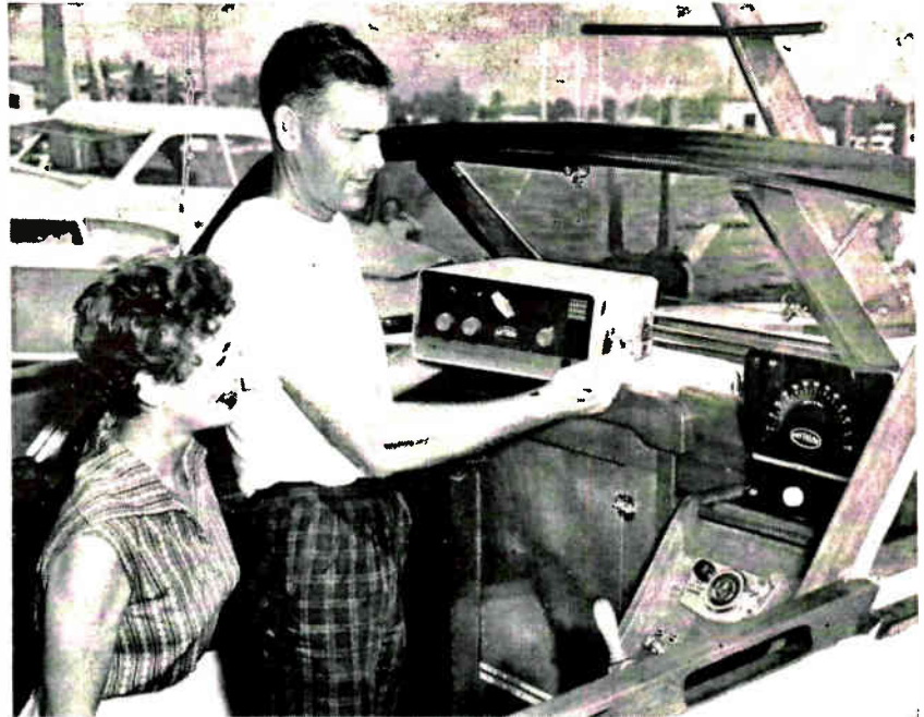
Transistorized 20-w unit is Raytheon's radiotelephone. Depth sounder is on right
