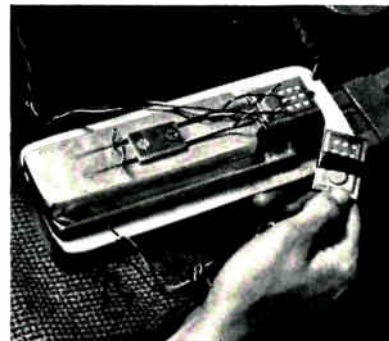
Spring clip replaces tape, speeding welding
