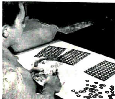
Finished parts are cut from sheet with shears
