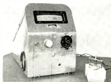
Front-panel view of watch timer showing test watch mounted on hollow block
