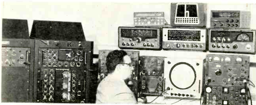
Radar communications countermeasures simulation equipment in operation. Multitarget generator producing large targets with antenna pattern simulator controlling basic i-f signal of high power
