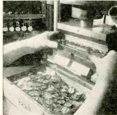
Disks hang in soldering machine (left) as excess wire is cut off in clipping machine
