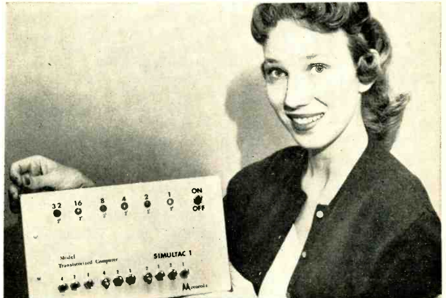
Model computer performs simultaneous binary addition in 7\mu\text{sec} . Only active circuit elements used are 178 transistors
