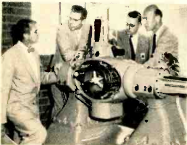
Discussing operation of Bendix Computer's three-dimensional flight simulator. Unit holds model of missile or aircraft undergoing test
