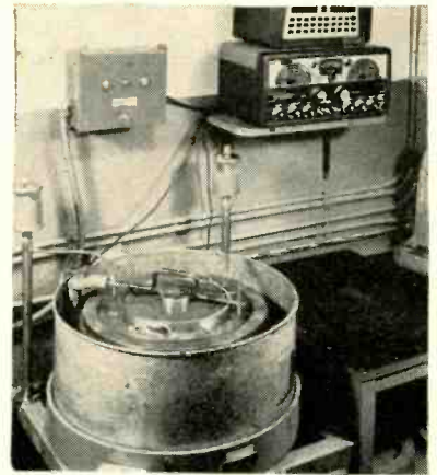
The front cover—planetary lap with automatic cut-off
