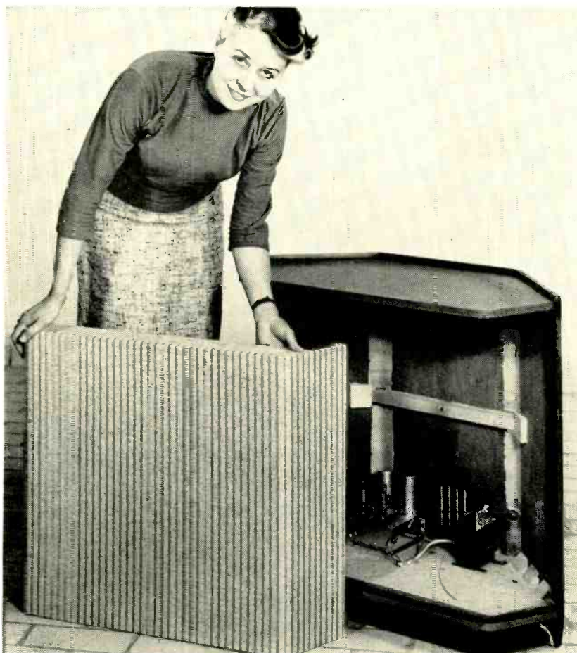
Young lady removes front piece to show amplifier within speaker enclosure
