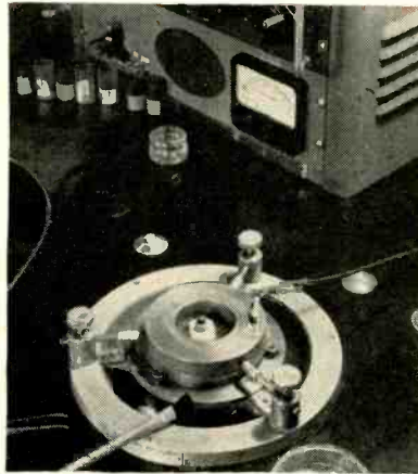
Impedance matching coaxial cable is connected to alligator clip
