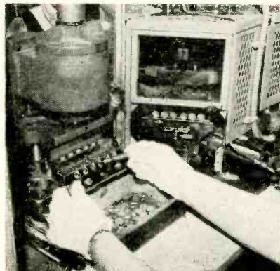
Soldering machine drops disks into clipping fixture (right) as clipper operator marks finished varistors
