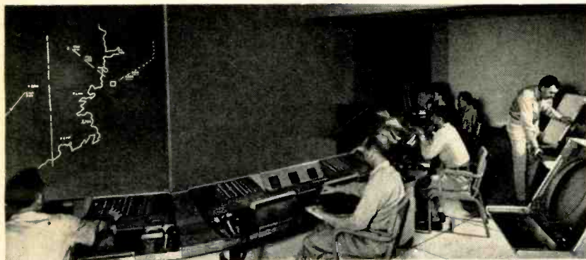
Air Defense officers at SAGE Command Post, McGuire AFB, N. J., watch the air situation over New York and Philadelphia areas. IBM computer presents an up-to-the-second visual display of air activities
