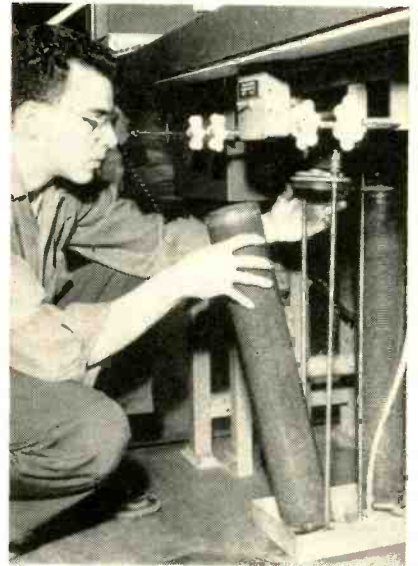
Plastic cartridge containing resin water purifiers is placed in position
