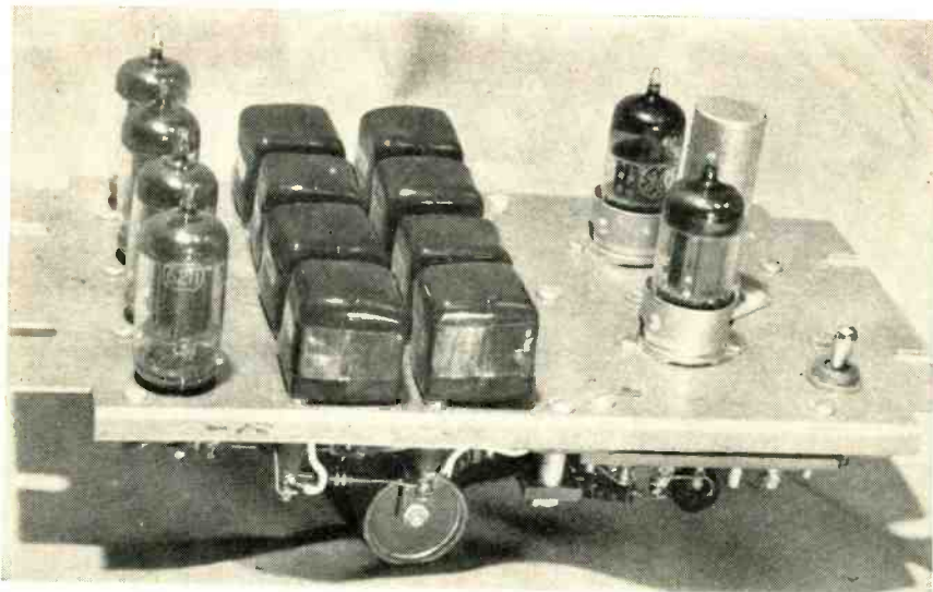
Complete 525 divider occupies space less than 4 by 5 by 2 in. on left side of chassis. Oscillator and discriminator portions of sync generator are on right side
