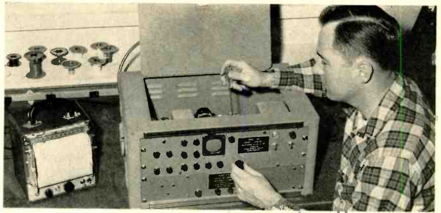
X-band klystron phase-locked with quartz-crystal oscillator provides stability of few parts in 10^8 over entire day. One use is atmospheric phase-stability research
