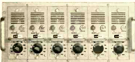
Six KIN TEL amplifiers in compact 19" rack mountable module.
