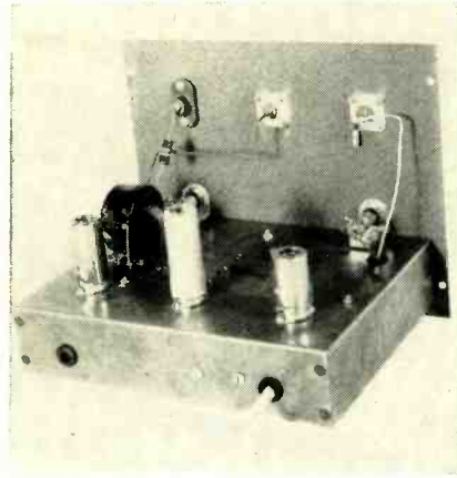
Front, rear and bottom views of the trigger generator show the physical layout of the components
