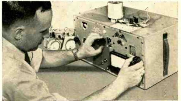
Dynamic measurement of a junction transistor under conditions of variable bias and applied RF. Similar procedures can be used with vacuum tubes.
