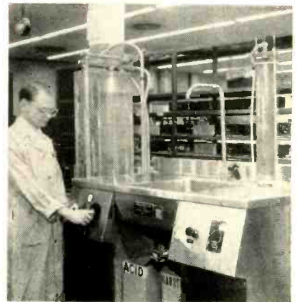
Spent cartridges are regenerated semi-automatically seven at a time on companion equipment
