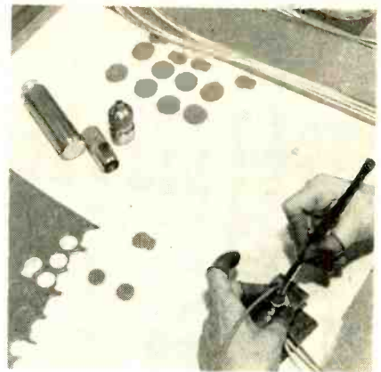
Prepacker uses cutouts stamped from rubber sheet with "cookie cutters"
