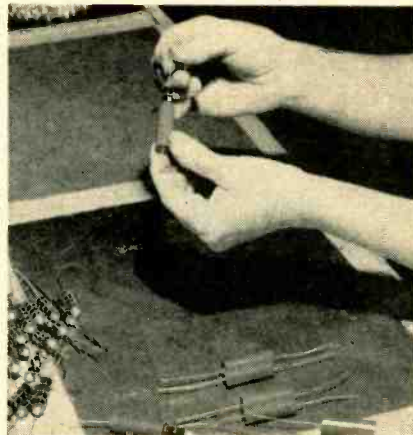
Resistors are first placed part way into shell
