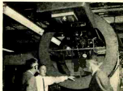
Huge deflection unit magnetically bends, focuses beams from 50-million electron volt linear accelerator
