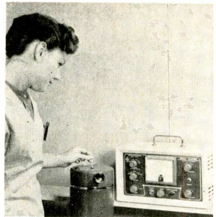
Radiation count of component is made manually, as shown, or on conveyor to determine rate at which tracer gas leaks into component
