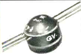
Wound core unit .01 micro-second rise time.
