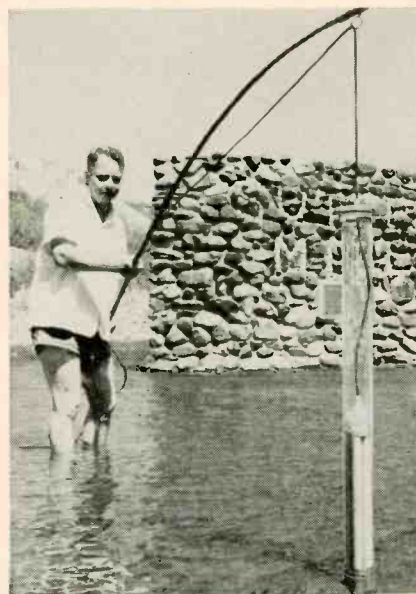
Sensing head of Geiger counter is lowered into position in river to gage flow of water containing radioactive gold
