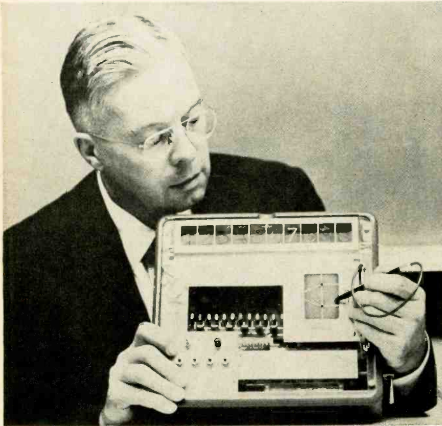
Hand written number reader can operate other data-processing gear
