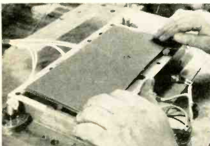
Copper sheet is placed over die first, then uncured board
