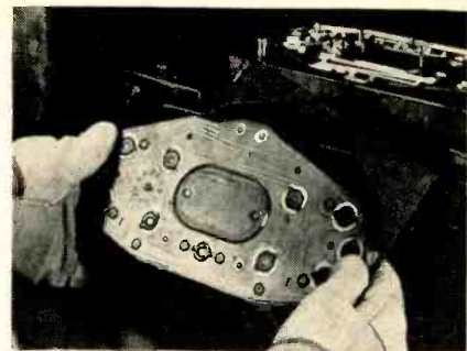
Removing punched and trimmed cured board from press, ready for use as behind-dashboard wiring for automobile. Dash lamp sockets snap into molded holes
