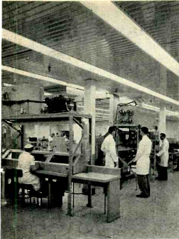
A section of the test area in G.E.'s Buffalo transistor plant. In the foreground is a humidity control box in which transistors are inspected prior to encapsulation.
