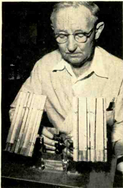
Arrangement of four lamination dispensers, with stacking jig in center
