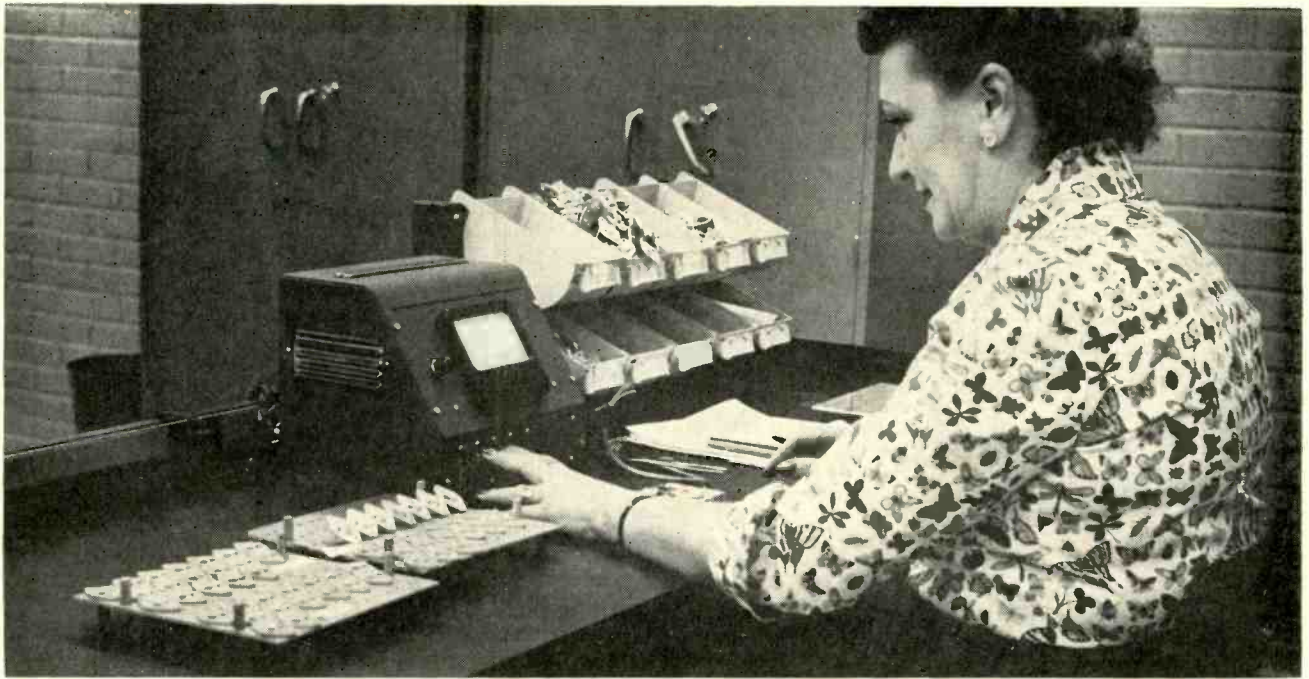
Operator uses parametrical test equipment to measure I_{c0} , I_{e0} and current gain of power transistors
