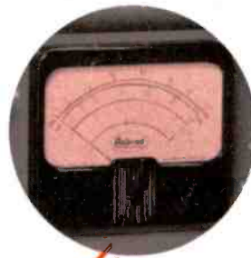
Output level reading directly in db High sensitivity
