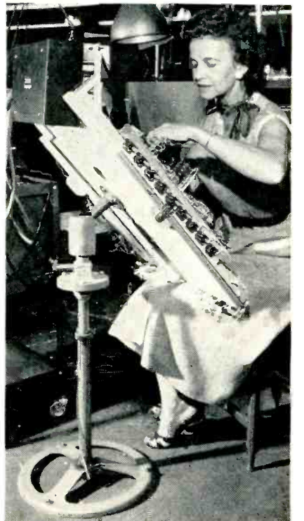
Adjustable-height harness board holder is bolted to floor. Single locking clamp permits adjusting board to most convenient angle for each phase of assembly work in business machine plant
