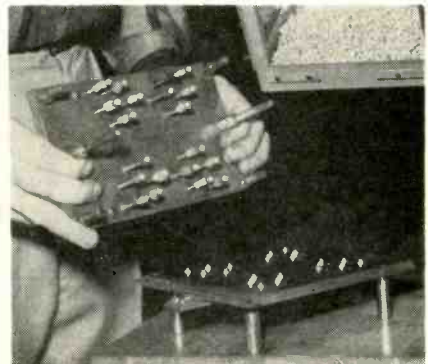
Transfer plate is placed over terminal collector plate and plates are inverted so terminals drop into transfer plate. In same way, mounting rivets are dropped into another transfer plate
