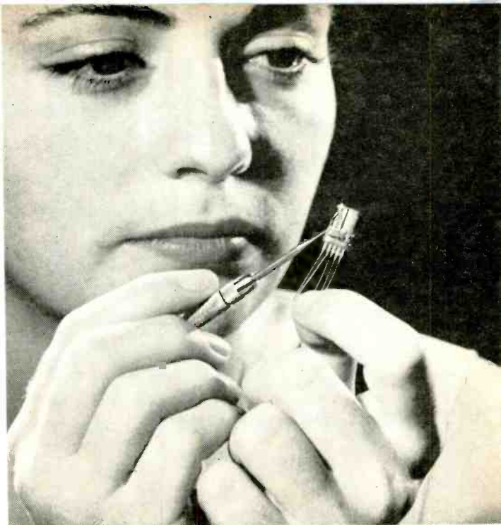
Relay by Elgin capable of handling \frac{1}{4} ampere at 28 volts has a life estimated at 1 million operations
