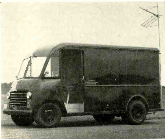
Exterior of mobile monitor shows corner reflector used for uhf reception. Interior, (right), shows rack-mounted instruments
