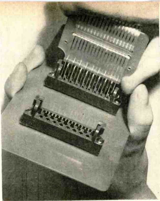
Printed-circuit cable connector by Elco attaches 17-conductor cable to circuit board. Flat cable passes through strain-relieving grip on plug
