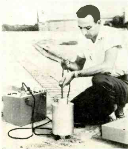
TWO MINUTES AFTER he lowers a probe through a protective shield (left) to a desired depth in the earth, the
