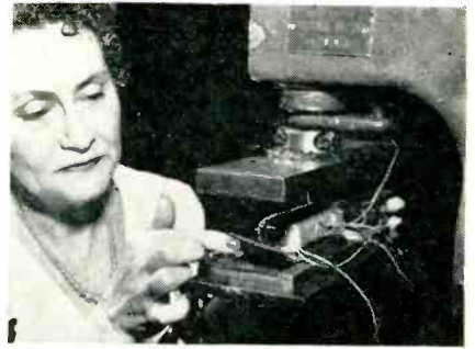
Operator lifts up rubber pad which cushions impact of press on coil assembly
