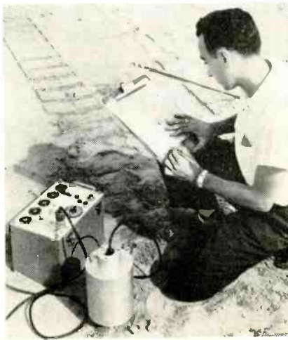
operator has accurately determined (right) the moisture content or density of the subsoil when radioactivity in . . .
