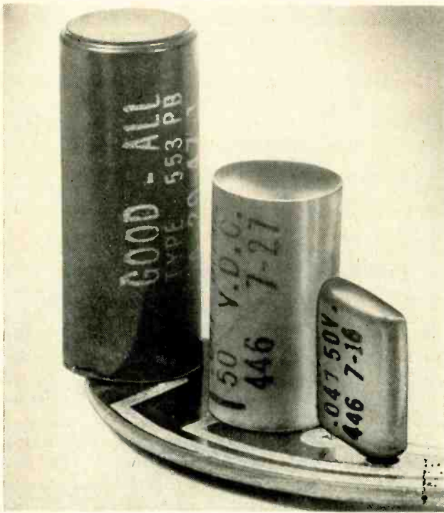
Three Good-All capacitors of same voltage and capacitance rating differ only in dielectric material and external housing
