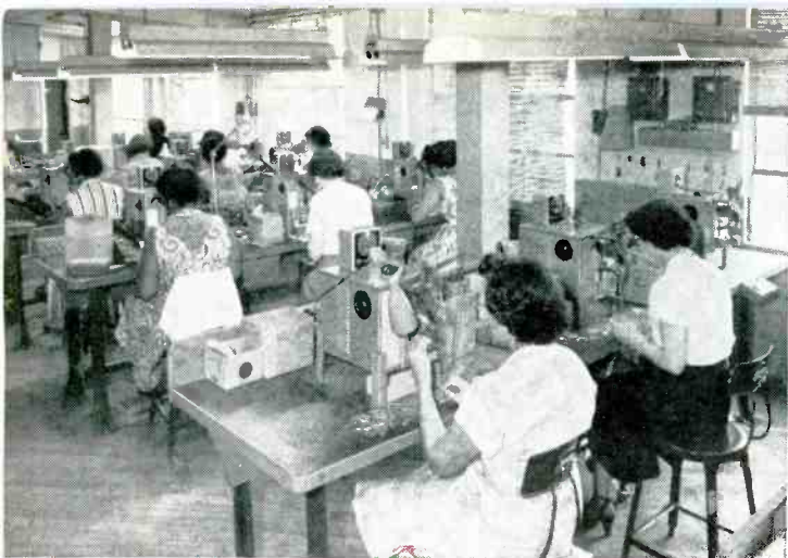
Ample Production Capacity — In this corner of the Assembly Department, spot-welding operations are performed on relay and thermostat sub-assemblies.
