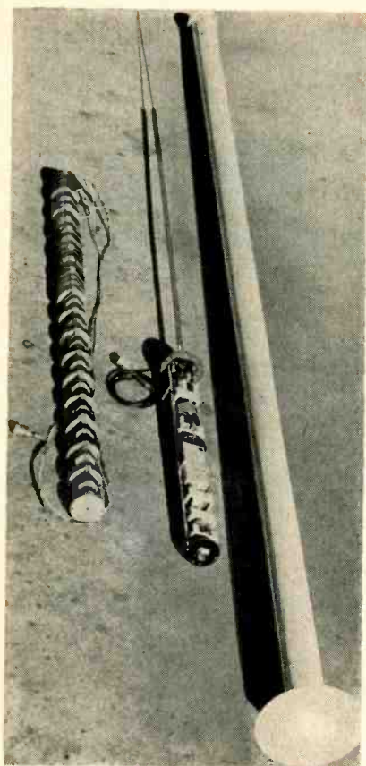
Complete assembly consists of (l to r) battery pack, electronic unit and buoy case
