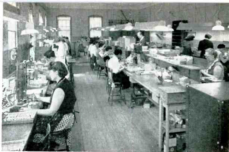
Thermal Relays are encased and hermetically sealed in this section of the Assembly Department.
