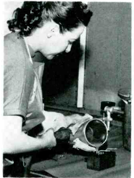
Pouring epoxy resin in mold to encapsulate toroid
