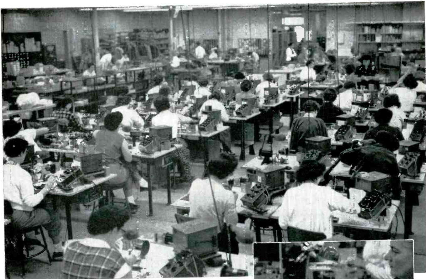
Operators in the foreground are trimming resistors down to close approximation of their final values, guided by L&N No. 4760 Bridges.
