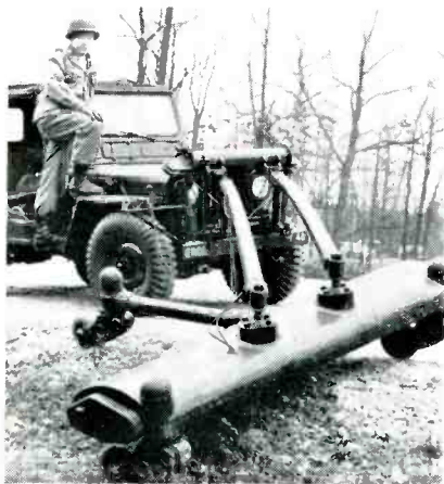
Horizontal sweeping of path ahead is provided by Army's latest mine detector. It stops jeep automatically when it discovers a buried mine
