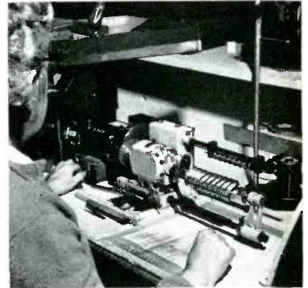
Winding a set of coils on take-apart mandrel. Wire is pulled through overhead tensioning pulley over end of spool at right rear on bench
