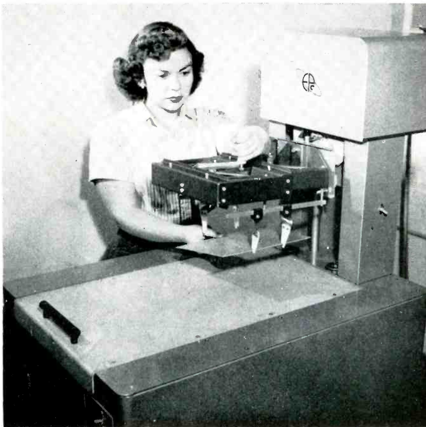
To load machine, operator pushes handle on top with left hand to spread out fingers of holding fixture so wiring board can be inserted with right hand. Fingers grip board when handle is released. Vibrator shakes board as it comes out of molten solder
