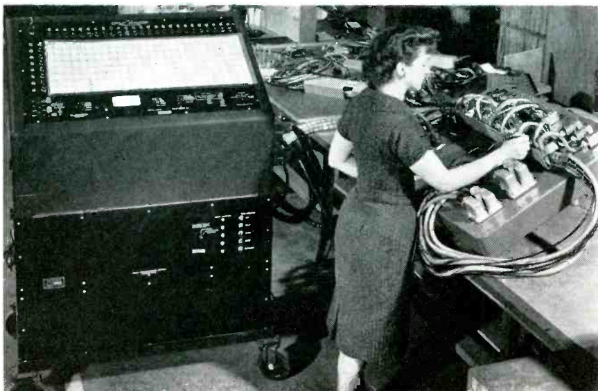
Automatic cable harness tester, mounted on dolly, is easily moved along bench for checking chassis and cable harnesses for large airborne equipment
