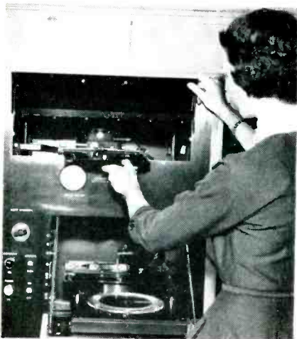
Radar Restitutor camera rephotographs original photographs of PPI radar presentations without the inherent distance distortions
