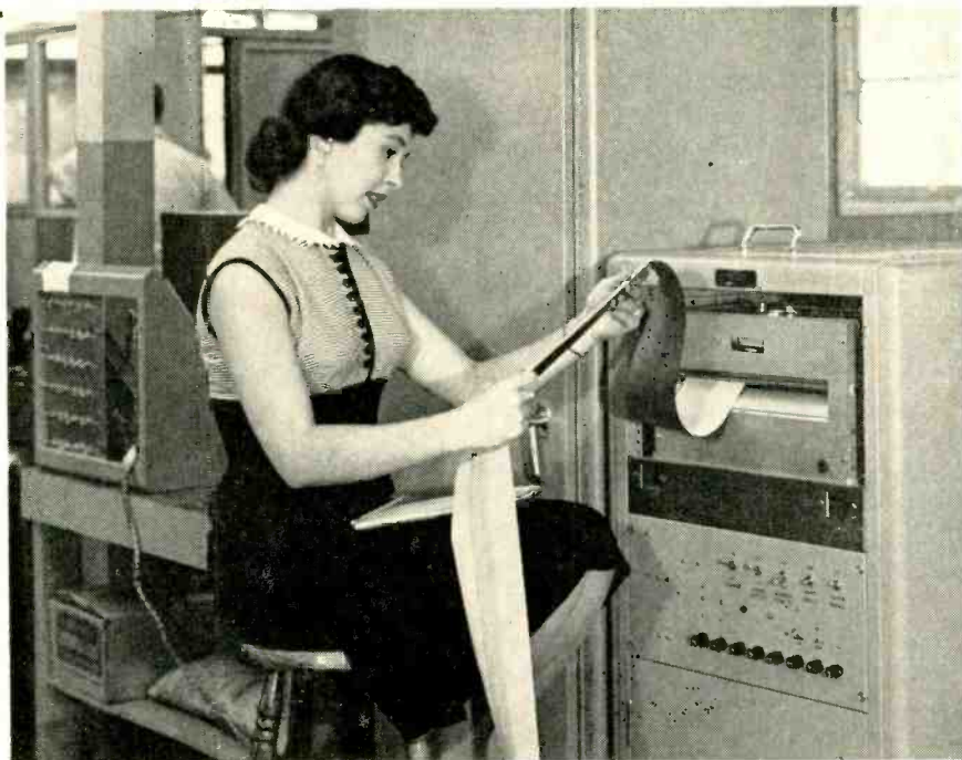
Twenty times faster than conventional printers, the recorder is shown here printing lines of twelve characters. Direct readout is accomplished by current, passing through fixed styli, which breaks down the electrosensitive paper coating. The same basic configuration will handle 102 characters per line and attain a readout speed of over a million characters a minute
