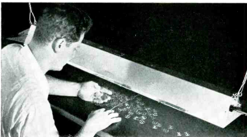
Inspecting mica spacers for tubes under overhead long-wave lamp. White fluorescence on punched edges indicates oil contamination from dies of punch press
