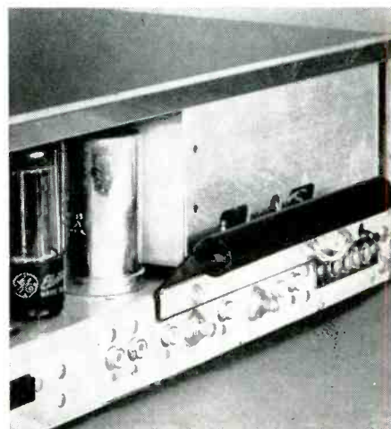
Plastic extrusion bolted to rear of high-fidelity tuner supports and protects fragile ferrite-core antenna
