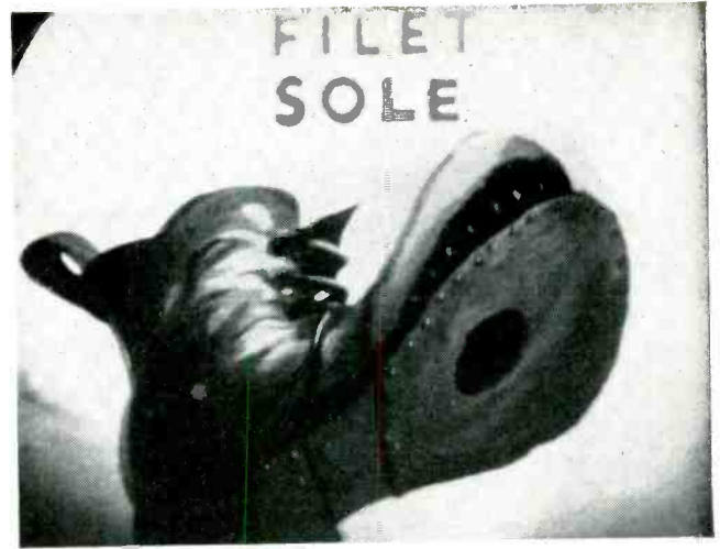
Picture of demodulated video from off-the-air signal is indicative of picture seen on home receivers. Sound beat pattern is filtered out by receiver sound trap
