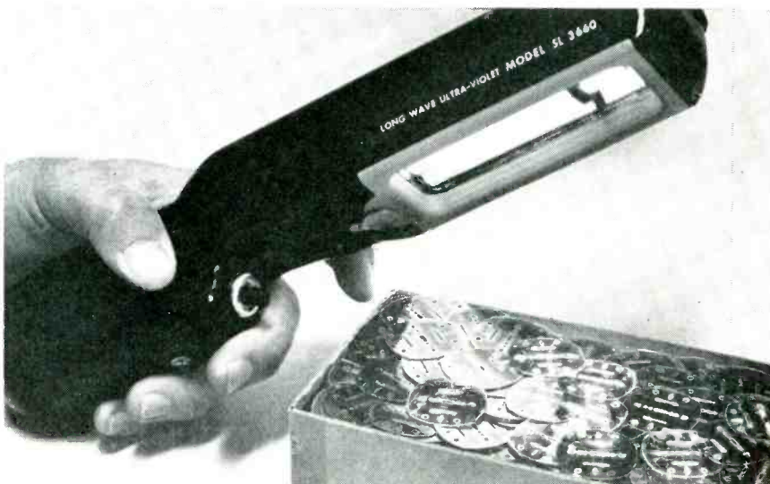
Using portable long-wave lamp to spot-check incoming mica parts for oil contamination
