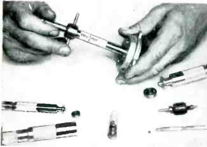
FIG. 1 Principle factors involved in fitting Micro-Bearings. Handling and fitting tools such as furnished by the Baker Co., Maplewood, Maine, enable operators to place or remove Micro-Bearings quickly, easily and help avoid damage.
