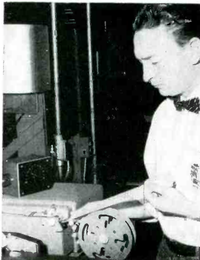
Removing punched tape. Control box on top of puncher gives choice of twelve different hole sizes, producing corresponding code markings on tape
