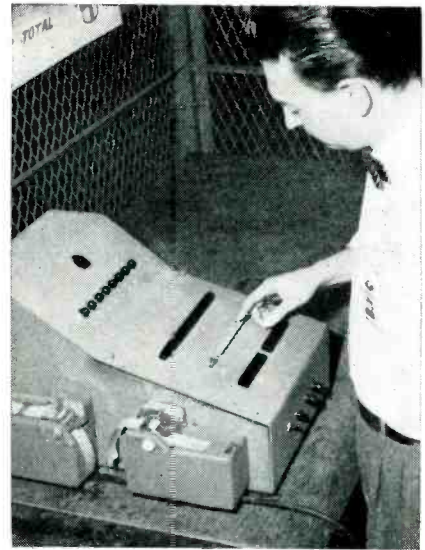
Tape proofing and correcting machine. Tape reader is at front left of machine and duplicating tape punch is at rear
