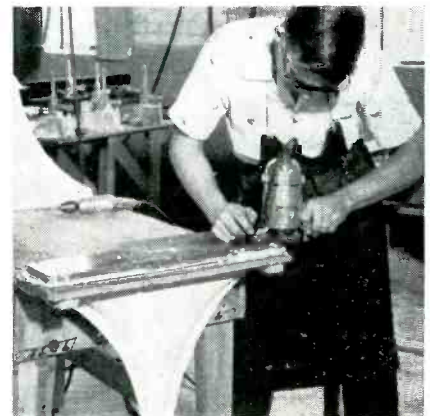
Trimming flanges of cemented horn with router running against steel template
