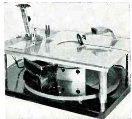
Coil-winding machine for miniature toroidal cores uses sewing action. Rotating magnet moves needle in circular path
