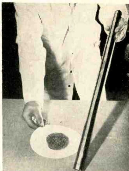
Unusually long bar of pure germanium converts to pile of 80,000 crystals shown
