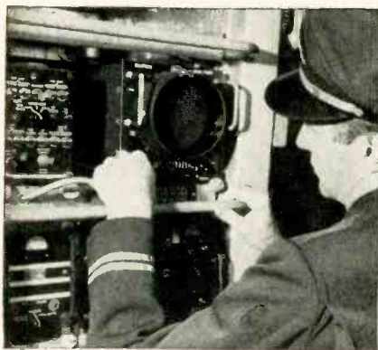
Waveforms on this Bendix analyzer enable flight engineer to check DC-7 ignition system in flight or on the ground. American Airlines has ordered 125 of the units for a total of $120,000
