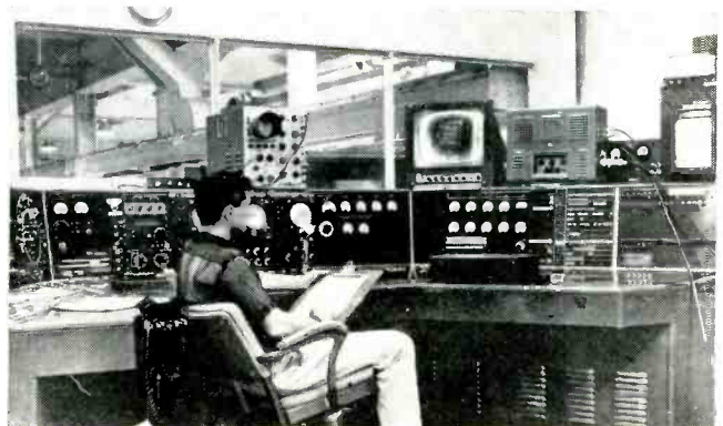
pattern produced on a sodium iodide mosaic (left) facilitates accurate adjustment of the focusing magnets. Remote control of the closed circuit tv system reduces exposure of personnel
