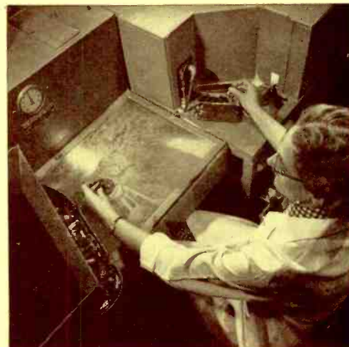
ABOVE: operator holds a 5-Star high-reliability tube while streams of abrasive emulsion scour oxidation off surfaces of pins. LEFT: pins before and after cleaning (unretouched photograph).
