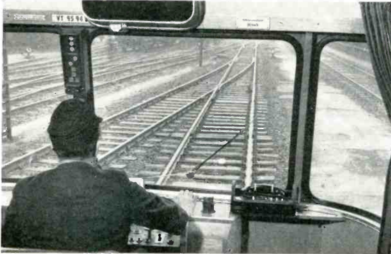
Motorman of passenger car has telephone (at right hand) and illuminated signal box (above his head). Signals from passing
