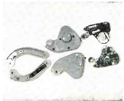
Disassembled induction receiver. Parts of receiver proper are duplicated to show obverse (right)
