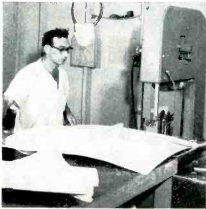
Roughing out sheet on band saw before cutting apart the two horn halves
