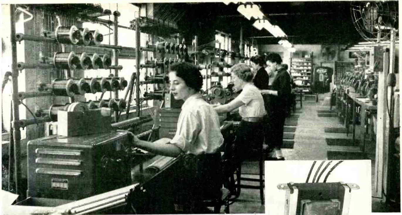
New Leeson No. 108 Coil Winders (foreground) in the plant of Ram Electronics, Inc., Irvington, N. Y., where Leeson Winders have become "standard equipment." These were added as best winders for producing short runs of stick-wound coils of varying specifications. (Inset) Ram has built an excellent reputation for winding quality coils and transformers used in radio and TV equipment.
