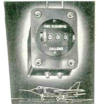
Fuel-Remaining Counter for aircraft . . . subtracts as fuel is used
