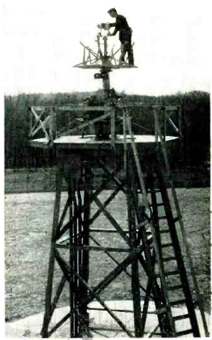
tests are being made on a transmission-reflection unit (left). The test tower (right) is 1,900 feet from the transmitter. Receiving equipment here detects effects caused by radome
