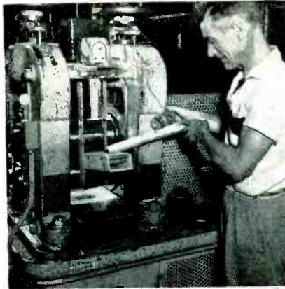
NEW magnetic core material is rolled, left, and molded to shape as . . .
