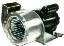
60-6 115 Volt (or 220 Volt) 60 cycle blower, 1 or 3 phase. 250 CFM at 2.5" water gauge.
