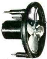
A15AD3 115 Volt 60 cycle axial blower. 35 CFM at .2" static pressure.
