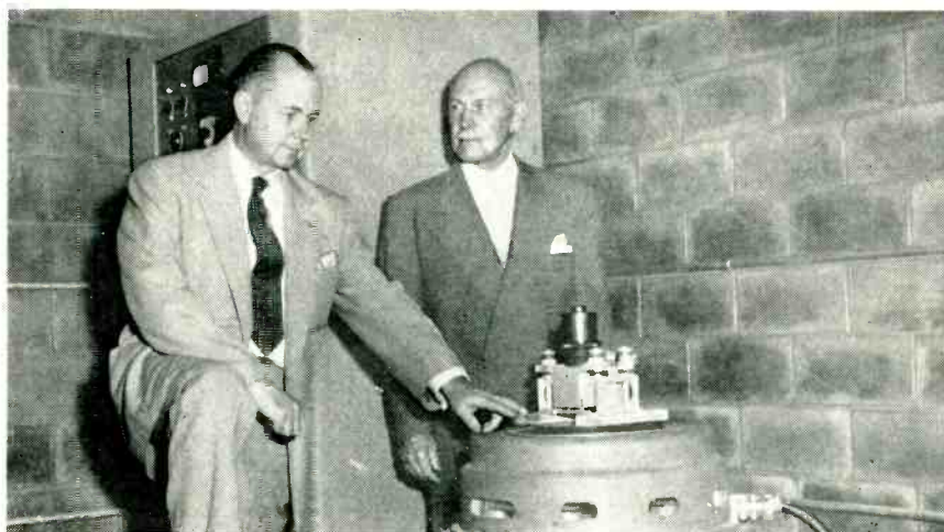
Vibration tests on electronic equipment can be made at frequencies as high as 2,000 cycles using the electromagnetic shaker shown. Primary exciter is an audio-frequency oscillator driving audio-amplifier stages to actuate the vibration device that is not unlike a huge loudspeaker. Demonstrating the effect of shock mounts in their new Teterboro, N. J. laboratory are C. S. Robinson and G. deF. Lerner of Robinson Aviation
