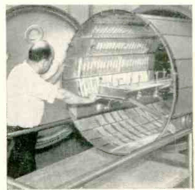
Vacuum Furnaces. Stokes melting and heat-treating furnaces permit electronic manufacturers to pre-process raw and semi-finished materials with less contamination, for increased life and performance.
