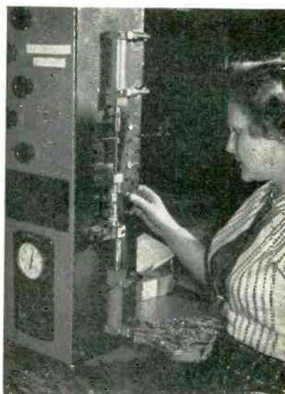
Pushing start button of robot tester after loading slide into fixture. Lower air cylinder simulates action of pushbutton, while upper air cylinder applies downward force to check holding power of cam
