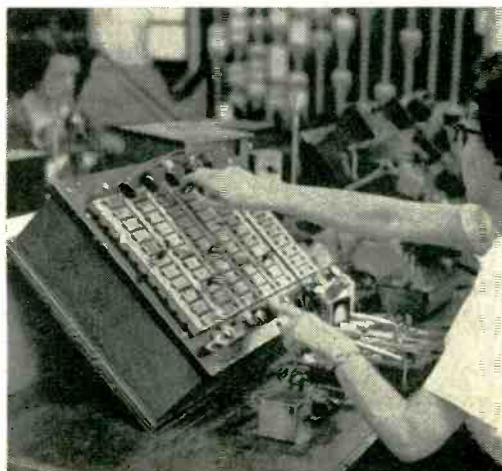
If an even higher degree of accuracy is required, the resistors are further adjusted with an L&N No. 4230 Anthony Pattern Bridge.
