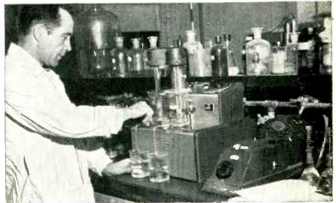
2. ANALYSIS OF EACH HEAT. Samples of each heat of the alloys are sent to Superior's metallurgical laboratory for extensive chemical and physical analysis. Metal must conform with rigid specifications before acceptance.
