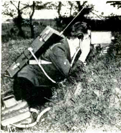
French development is one of small pickup units used by CBS. Amplifier, transmitter and battery are contained in the pack. Camera held in hand
