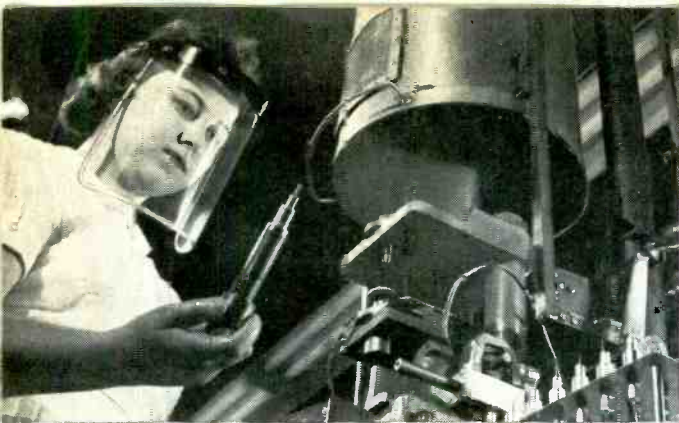
GL-6442 tubes in quantity production by General Electric are assembled by r-f brazing in a hydrogen atmosphere.
