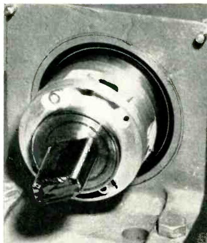
Compound headstock permits aligning proper crystallographic plane of germanium ingot to cutting plane of saw after centering ingot to face plate
