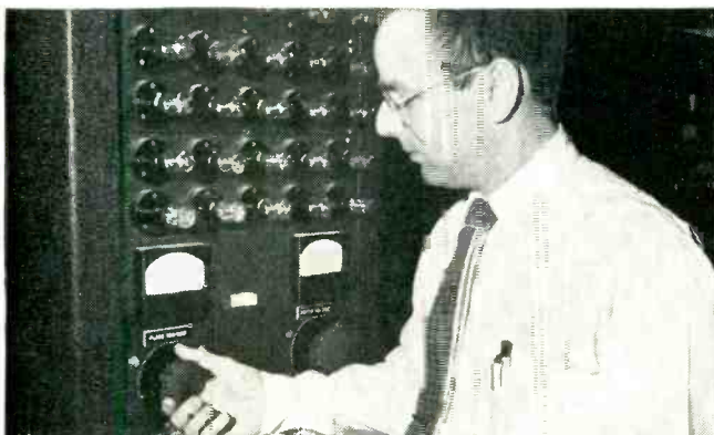
3. TESTED IN ELECTRON TUBE. Samples of each heat of Cathalloy are fabricated into cathodes and assembled into ASTM standard diodes. They are operated under controlled conditions. These tests evaluate each heat for emission and sublimation characteristics. Satisfactory results approve the heat for production.
