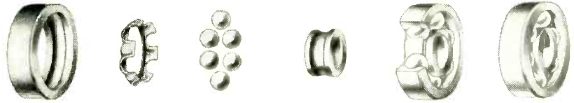
Retainer Bearing — Exploded and Assembled Views
