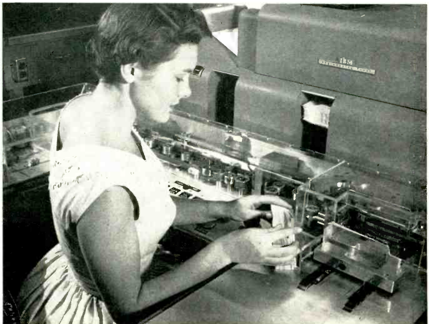
READING Operator at console feeds checks into SRI's Electronic Recording Machine Accounting (Erma) system. Models under development will read directly characters printed in magnetic ink. Present system relies on code bars
