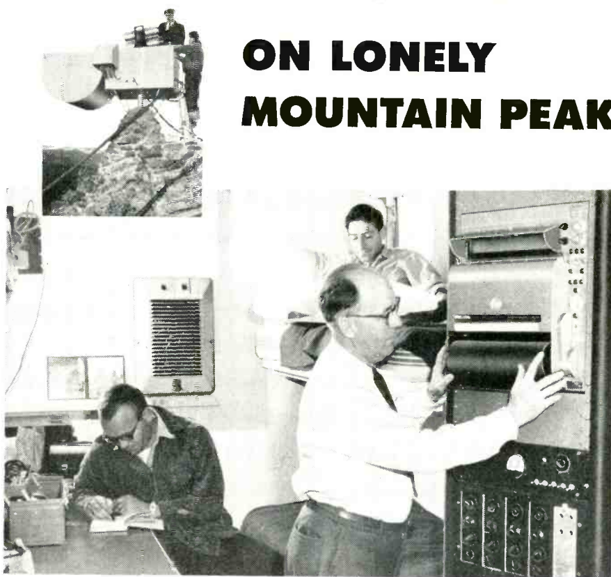
Dr. Franklin E. Roach, consulting physicist to the National Bureau of Standards, loads a record take-up drum into the Heiland oscillograph.
