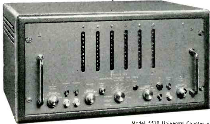
Model 5510 Universal Counter and Timer offers direct-reading digital display of count, frequency or microsecond time interval. Time bases from 1 mc. to 1 cps; gate times from .00001 to 10 sec. Accuracy \pm 1 count, \pm crystal stability (1 part in 10 9 ). Price $1,100.00 f.o.b. factory.
