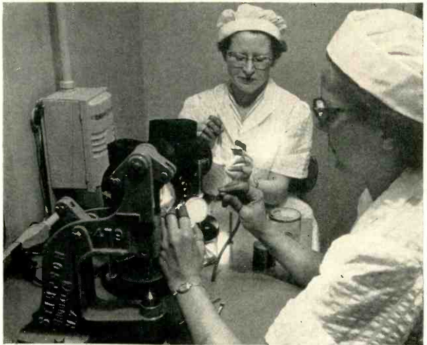
TARGET and mesh assembly of camera tube is formed under dust and lint-free conditions at GE plant while . . .
