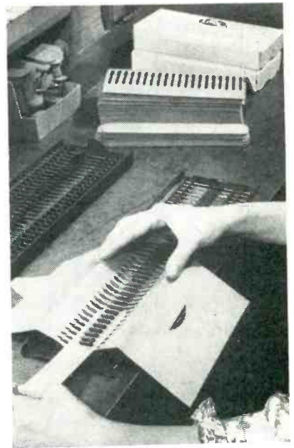
Method of inserting lacer strip to anchor precision resistors in holder of shipping carton. Each metal tray-load of resistors fills two cartons
