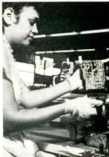
Method of holding finished wiring board, after masking its corners, for applying activated rosin flux with ordinary paint brush
