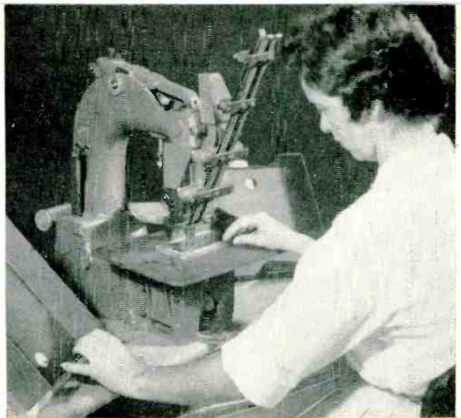
SINGLE HEAD —Basic heads from United Shoe's automatic assembly machine can be used as bench machines by adding a foot-treadle switch to actuate solenoid-operated control valve
