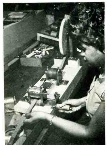
Setup for cutting cork tape into pieces 1\frac{1}{2} inches long. Metal protective shield for cutter, on bench at left, has been removed to show method of mounting blades in cylinder
