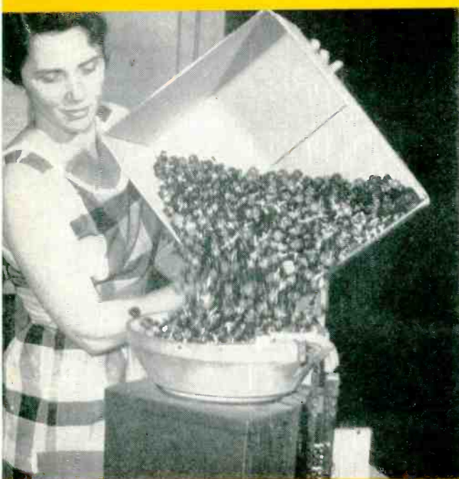
INSERTION HEADS —Dumping 7-pin sockets into hopper of Syntron feeder, for orienting by missing pin and loading into magazine that slips into position on Admiral's socket-inserting head. For same machine, body-taped capacitors in strips about 18 inches long are dropped into loading chute of capacitor head and tape is pulled off. Leads are cut and formed by head
