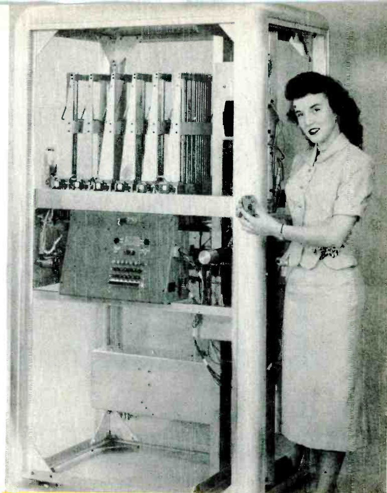
SINGLE-STATION MACHINE —Programmed system, under construction for Bureau of Ships by Melpar, will have punched-card control of magazines and air-servo positioner. Present model feeds board automatically and inserts choice of six different components at six positions on board in sequence. Clinching anvil is heated for self-soldering. Pushbuttons permit manual operation.
