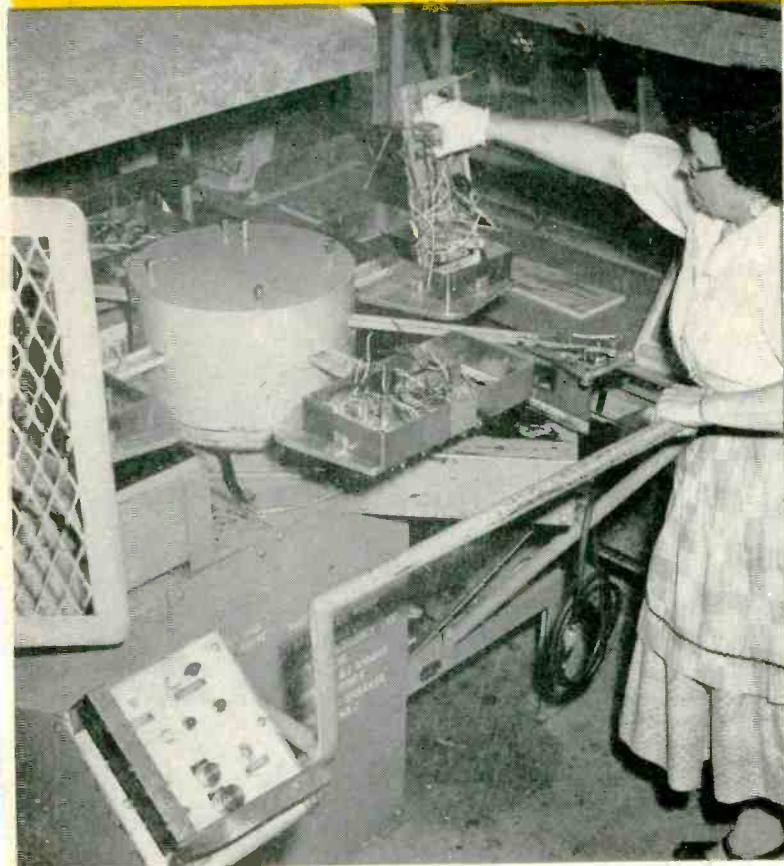
DIP SOLDERING —Machine soldering can be done in many different ways, as illustrated by these two Westinghouse designs. Flip-flop version above handles three radio boards at a time, for spray-fluxing at one end and soldering at other end after 180-degree upward swing through hot air blast. In up-and-down version below, entire central head moves up or down and rotates
