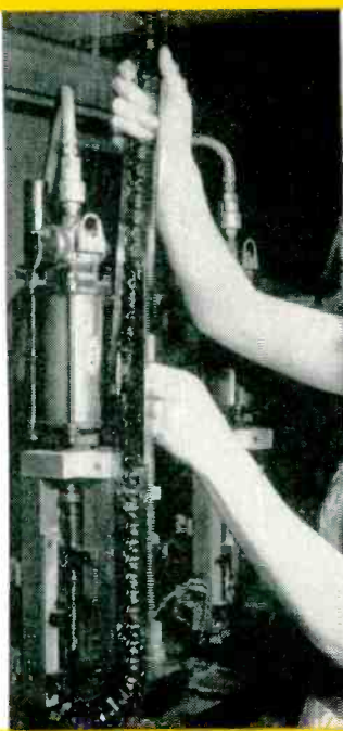
INSERTION HEADS —Dumping 7-pin sockets into hopper of Syntron feeder, for orienting by missing pin and loading into magazine that slips into position on Admiral's socket-inserting head. For same machine, body-taped capacitors in strips about 18 inches long are dropped into loading chute of capacitor head and tape is pulled off. Leads are cut and formed by head
