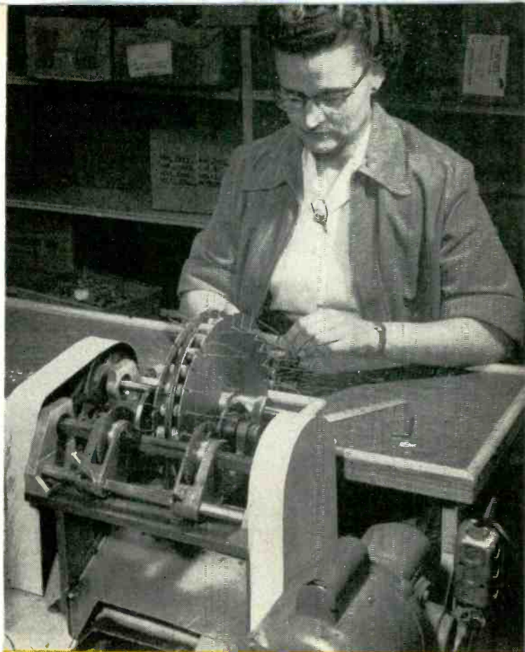
LEAD CUTTER —Motor-driven shearing blades and ferris-wheel feed on RCA machine solve problem of cutting limp, bent leads of heavily waxed tubular paper capacitors
