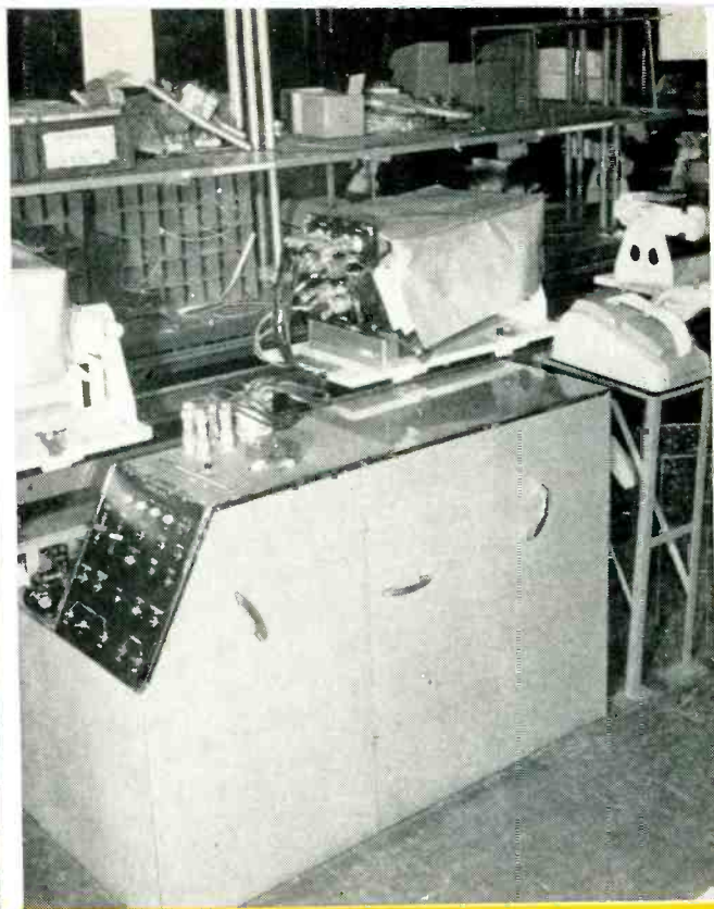
AUTOMATIC TESTING —Completely automatic GE test machine for finished military electronic equipment is programmed by punched tape. Result is recorded on tape by Clary printer
