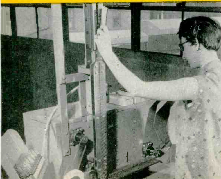
BELTING MACHINE —Resistors or capacitors in corrugated paper sleeves are fed into vertical feeder slide of Allen-Bradley machine for body taping on Minnesota Mining's filament tape at rate of over 20,000 units per hour (10 to 20 filled reels, depending on component size). Twelve-inch tape leaders facilitate loading and splicing an assembly machines. Reels are expendable
