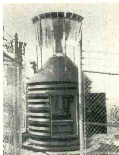
FIG. 3—Deer Creek radio reporting rain gage station showing special baffle around mouth of gage opening to cut down wind eddies and insure representative catch
