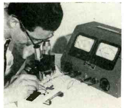
Method of using binocular microscope to aid in welding tap to single turn of resistance wire. Lamps held on microscope with rubber bands illuminate work area. Microscope base slips under wood fixture holding potentiometer
