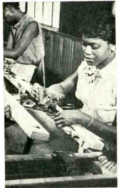
Pressing capacitor into mounting clip after leads have been inserted in punched holes. Slide-along line with grooved hardwood ways permits insertion of parts having long untrimmed leads, which are cut and clinched manually by operators at end of this line
