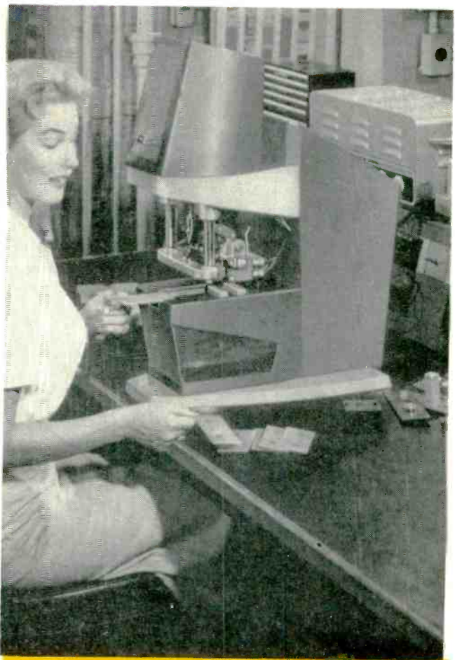
SINGLE HEAD —New General Mills unit designed for bench use, with wiring boards being fed in and positioned manually. Leads are clinched automatically after insertion
