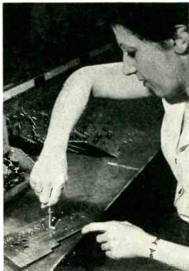
Method of holding tool while rotating wiring board, for spreading lugs
