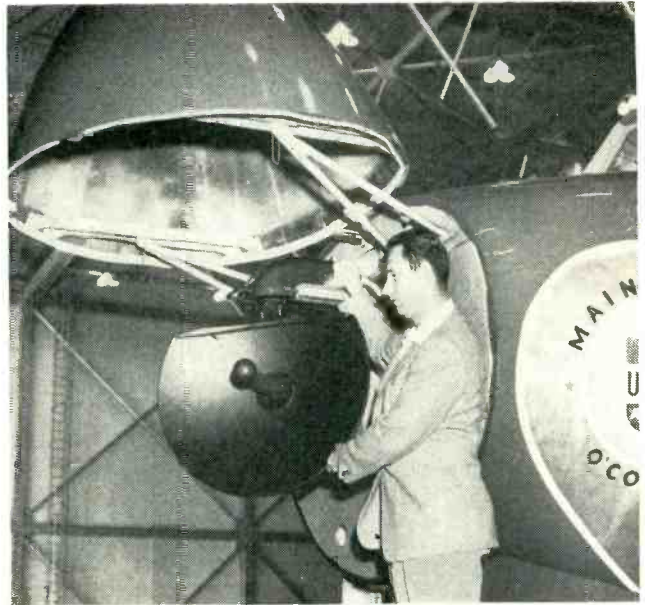
fleet uses the C-band, centered at 5.5 cm. Antenna (right) normally housed in plastic nose of aircraft is capable of 360-degree rotation but generally scans only the 240 degrees at front and sides of the aircraft nose.
