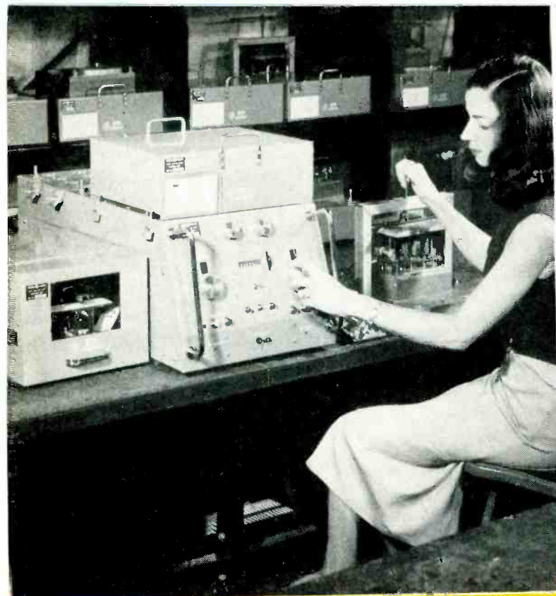
AUTOMATIC TESTING —Setup used by GE at Utica. After operator clamps board into fixture at right, CTI machine runs off electrical tests and prints results on paper tape at left
