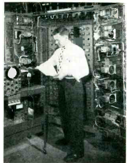
Eight analog computers simulate the four 3,500-hp aircraft engines of the C-124A Douglas Globemaster. Electronic equipment shown is a simulator used by the Electronics Division of Curtiss-Wright Corp.
