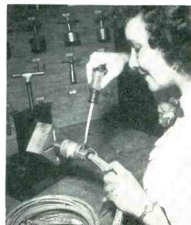
Tightening connector while wrench in block holds plug. Rack at rear holds other sizes of wrenches
