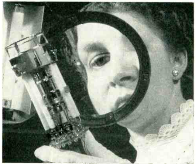
Three-gun assembly gets careful scrutiny before being sealed into color kinescope tv tube
