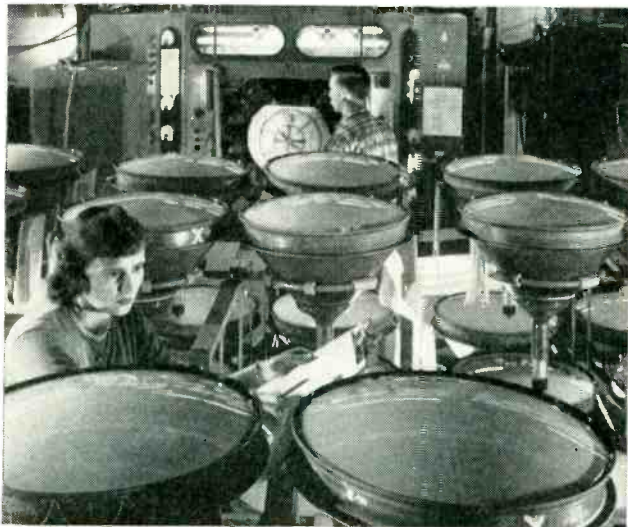
Completed color tv picture tubes undergoing final inspection at RCA plant in Lancaster, Pa.
