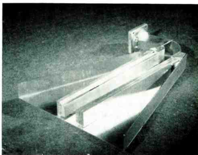
H-plane horn has 100-kw peak output. Choke arrangement and movable side walls are visible in photo at right
