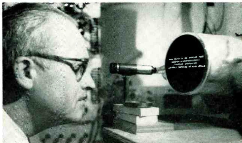
W. H. Bliss of RCA, Princeton, inspects resolution of letters on the face of an electron-image tube that translates coded information into printing
