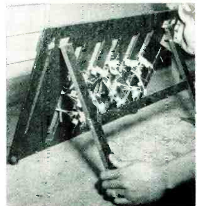
Rear view of fixture, showing method of attaching legs. Wing nut for adjusting angle of legs is near right hand of operator
