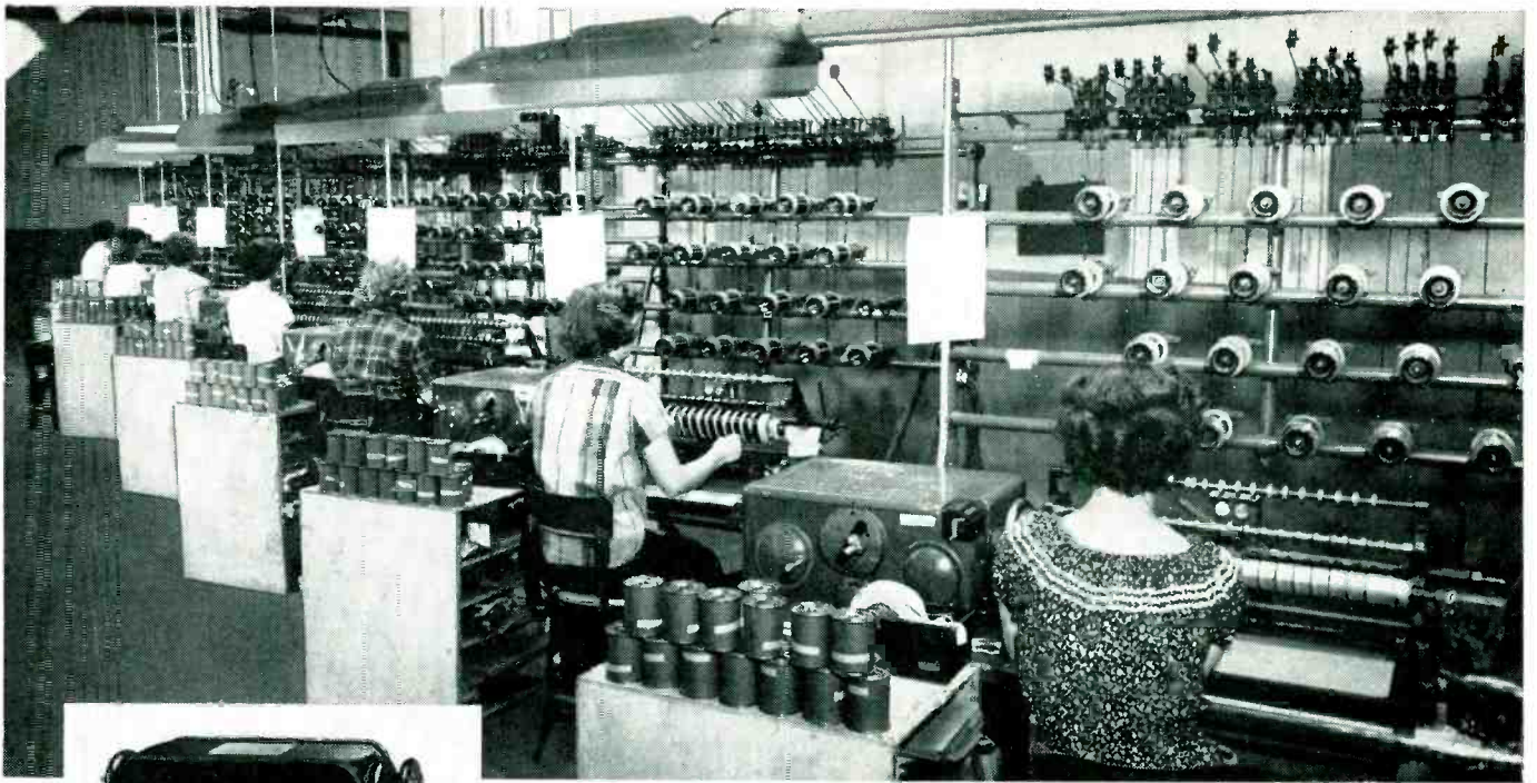
Battery Of Leesona No. 108 Coil Winders installed in the plant of Acme Electric Corporation, Cuba, N. Y. The most advanced hand-feed coil winders ever designed, Leesona No. 108's wind 4 to 30 paper insulated coils in stick form simultaneously. Note how conveniently the controls are located for quickly changing to a new coil spec — one of many advantages for speeding production on long or short runs. Inset shows an Acme Electric precision-wound luminous tube transformer which features coils that provide 18 MA 12000 volt secondary.
