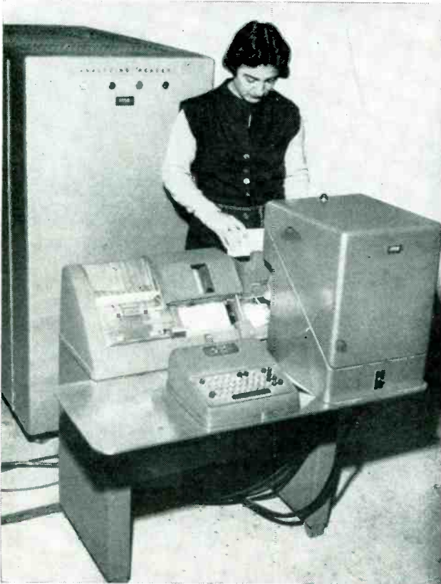
Model of analyzing reader first developed for Farrington Mfg. Co. reads a ten-digit account number from a Charge-Card sales invoice and punches the number into the same card, using a standard IBM card punch.
