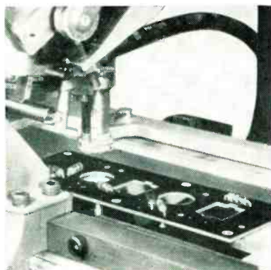
TUBE sockets and other components are automatically inserted by . . .
