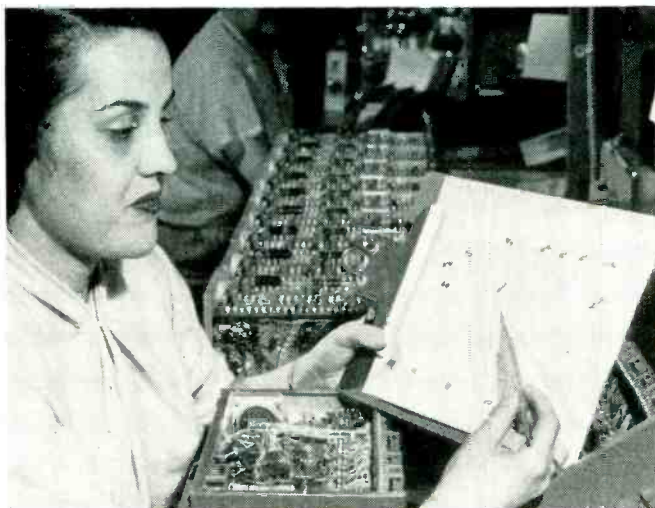
Method of marking pictorial inspection record to show defects Example of inspection record for cross-pointer omnichassis
