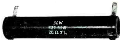
Corning Type R High-Power Resistors—Range from 25 to 1,000,000 ohms, ratings from 7 to 115 W. are non-inductive. Exceptionally good noise and frequency characteristics. Excellent moisture resistance and overload capacity recommend them for stable long-life service under adverse conditions. Meet MIL-R-11804A Specs.
