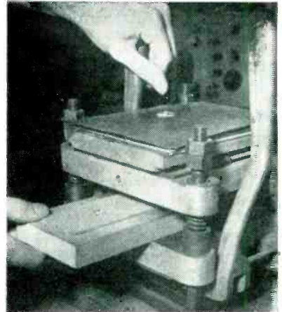
Putting engraved block and rubber sheet in hot press
