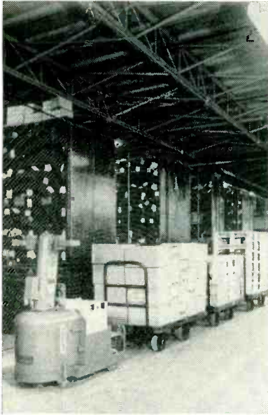
Industrial tractor is guided by radiation from control wire strung from overhead beam
