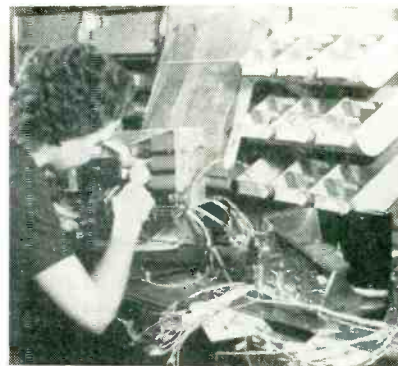
Typical assembly-line position, where timer is installed in chassis for pilotless bomber
