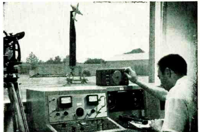
Electronics Research Engineer Irving Alne records radiation antenna patterns. Twenty-two foot plastic tower in background eliminates ground reflections, approximates free space. Tower is of Lockheed design, as are pattern integrator, high gain amplifier, square root amplifier, logarithmic amplifier.
