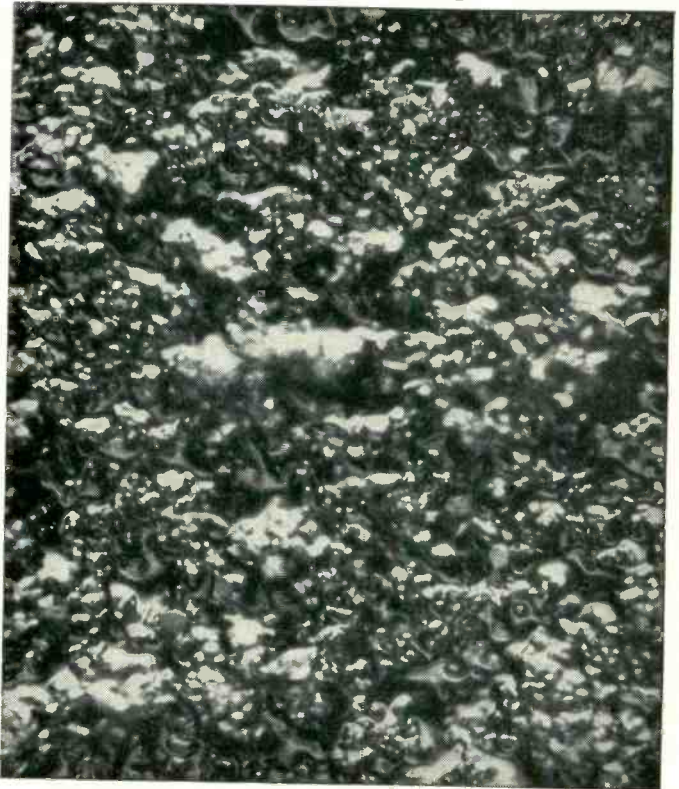
WESTINGHOUSE TUBE — Here's a photomicrograph of the Westinghouse aluminized tube manufactured with the exclusive Westinghouse "Flow-Filming" process, taken under the same conditions. Note the smoother, more even aluminum coating. It means you get maximum reflection, sharper, more detailed images.
