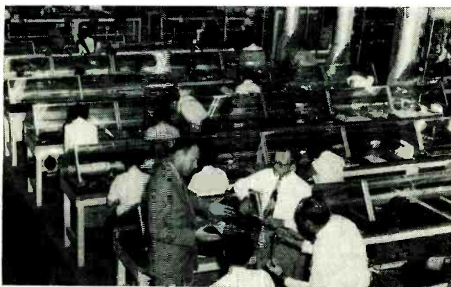
Dust-free air comes down ducts at upper right for distribution to benches. Flexibility of transparent hinged hood design permits installation of special binocular microscopes and other equipment needed for precision assembly of tubes. Diagram shows arrangement of units on ceiling and floor
