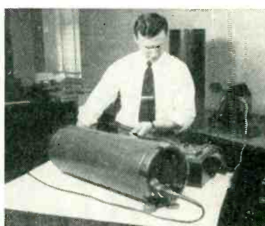
Laboratory test of unattended repeater designed for use in 12-channel carrier telephone system. Watertight unit in cylindrical aluminum casing is required every six miles to restore transmission levels. Bell Telephone Laboratories did the development work
