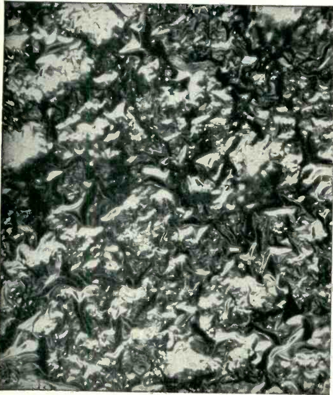
COMPETITIVE TUBE — This photomicrograph magnifies the inside reflective surface of an aluminized picture tube 200 times. You can see clearly its uneven "hill-and-valley" coating which causes some light to be lost within the tube, cuts down on brightness.
