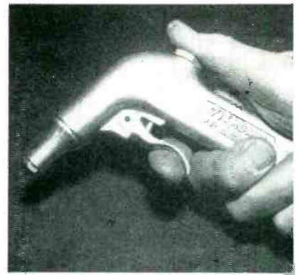
Modified air gun, with air shield outlet barely visible at base of nozzle for producing protective cone of air
