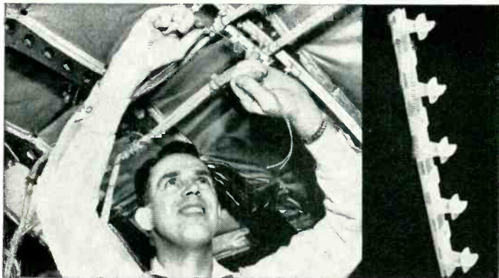
These wire supports molded of "Zytel" nylon resin (named "tombstones" because of their shape) can take any size wire bundle and eliminate the disadvantages of metal clamps. Besides saving many man-hours in installing airplane wiring, "Zytel" nylon standoff insulators are lightweight, take stress in all directions and are impervious to solvents - including gasoline and jet fuels. "Zytel" is also fungus-resistant, an excellent insulator and won't carbonize. (Stand-off insulators are manufactured by the Nylon Molding Corporation, Garwood, New Jersey, under license of Boeing Airplane Company, Seattle, Washington.)
