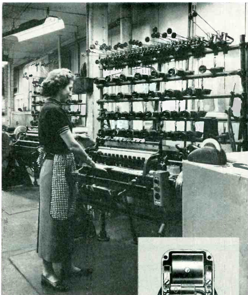
These Leesona No. 107 Automatic Coil Winders, shown in the plant of Wico Electric Company, West Springfield, Mass., were selected because of this firm's long, satisfactory experience with Leesona machines. Leesona No. 107 Winders, featuring speed and accuracy in automatic winding are enabling many plants to boost production and cut costs. Inset shows a cutaway of a Wico Model XH Magneto. Coil at top of unit is precision wound on Leesona No. 107's.
