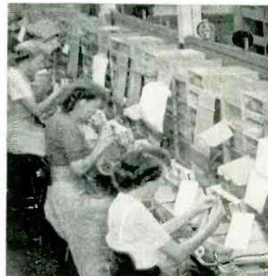
Assembly line in which rails are used on bench to aid pass-along operation
