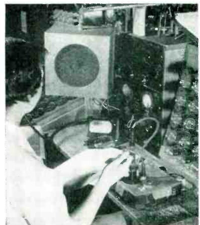
Setup for making round-robin noise tests. Slanting rack at right serves for preheating tubes before test. Noise is heard from loudspeaker and indicated by flickering of pointer of wattmeter on bench
