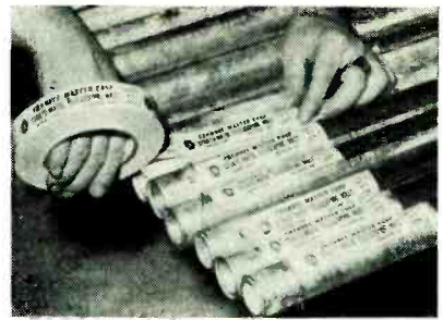
Applying tape for later guidance of customer in assembling antenna. Other printed lengths hold hardware together
