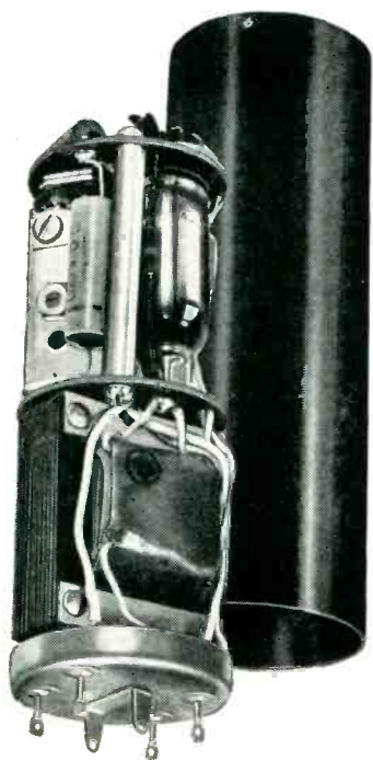
JAMES MODEL C-867 INPUT 6.3 VOLTS OUTPUT 750 VOLTS D.C.
