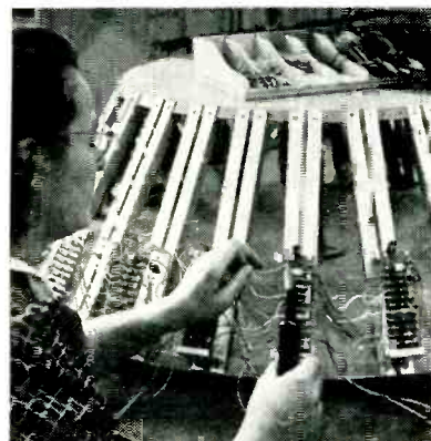
Lazy Susan jig holds resistor cards for soldering and assembly. Use of this setup cut by 40 percent the time required when individual jigs were used. Operator spins the jig to do the same operation on each card in turn, then repeats for the next operation
