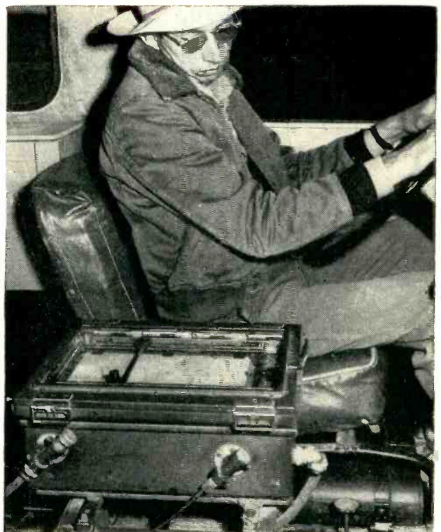
Gravity method of geophysical exploration. Operator, left, is using a portable gravity meter, while jeep driver, right, keeps track of crew's location with odometer
