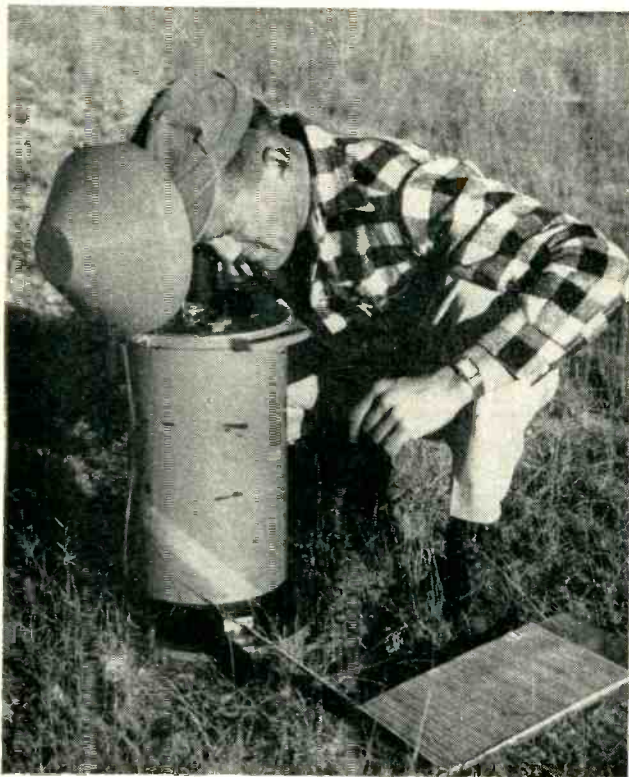
Gravity method of geophysical exploration. Operator, left, is using a portable gravity meter, while jeep driver, right, keeps track of crew's location with odometer
