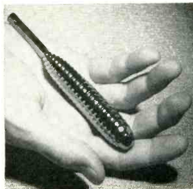
Quarter-pound germanium ingot, rate-grown by GE step technique in two hours, gives 2,000 transistors.
