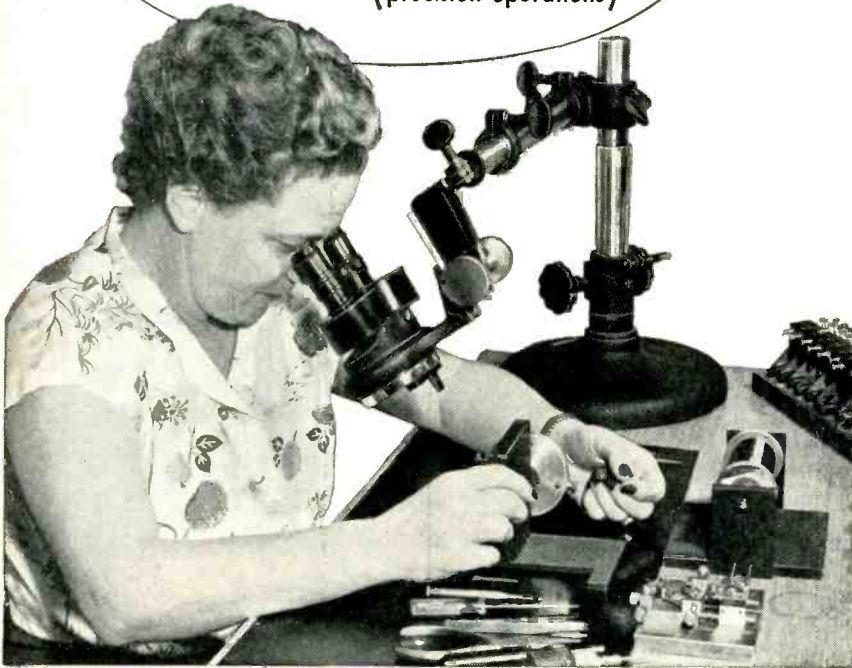
At the Hathaway Instrument Company, tiny galvanometer coils are wound with wire so fine that it is almost invisible to the unaided eye. Ingenious tooling and use of an AO Stereoscopic Microscope assure fast, precise workmanship.
