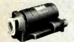
Gearhead DC motor. Continuous duty, air-over-totally-enclosed type with single stage reduction spur gearing and built-in filter. Typical application: aircraft fuel pump.
