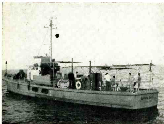
Seismographic operations in the Gulf of Mexico. Radar ship, left, keeps track of other ships in fleet. Target antennas mounted on ships anchored, right, provide positive radar identification
