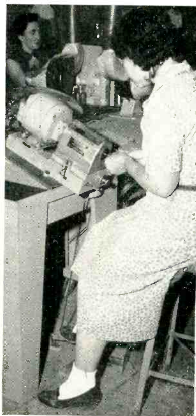
Mounting wire stripper at forward angle as shown greatly reduced worker fatigue. Ruler mounted behind twisting head makes length setup easier
