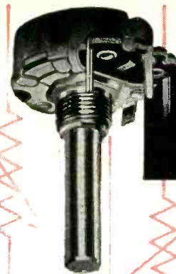
Cutaway view of CTS 252 Series, 1\frac{1}{4} " diameter 2 watt wirewound variable resistor. The total resistance can be varied from 3 ohms to 15,000 ohms, depending upon the size and type of resistance wire used.
