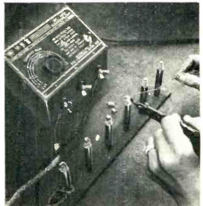
This jig lines up coils and terminations to be soldered together before plastic molding. A Wyse arc-melt soldering unit (Wyse Labs. Dayton, Ohio) is used, with one graphite electrode and one clip attached to the metal jig
