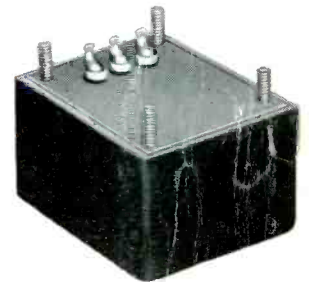
This 600 ohm miniaturized low pass filter is housed in a case only 1" x 1 3/4" x 2 1/2".
