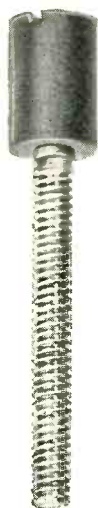
PYROFERRIC INSERT CORES Diam: .245 to .250 • Insert: 4-40 x 1" Extending Slot in Core: 1/32 x 1/32
