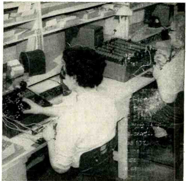
Production-line testing at Daven plant selects resistors within specified tolerance range. Improved fabrication methods have narrowed range of quality variations, producing more accurate resistors at lower cost
