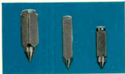
Pre-drawn shapes, such as triangles and squares, are naturals for carburetor needle valves.
