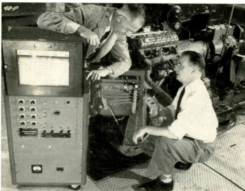
Continuous loop of 35-mm film perforated at intervals plays electronic circuits that control test engines at California Research Corp.
