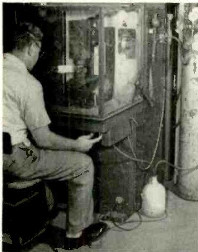
Resistance brazing setup for magnetrons
