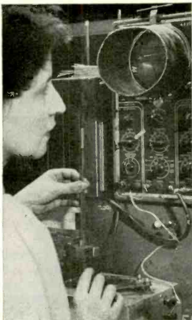
Setup for rough adjustment of printed i-f transformer
