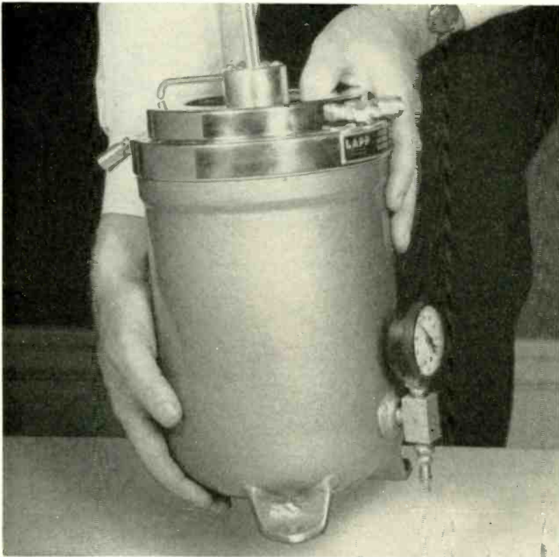
Example of unit using gas pressurizing technique to boost voltage rating. Unit shown here, made by Lapp Insulator Co., is variable water-cooled capacitor rated to carry 70 amperes at 1 mc. Gas inlet is below gage near bottom, and water inlet and outlet fittings are at top. Tuning rod projects upward at top center
