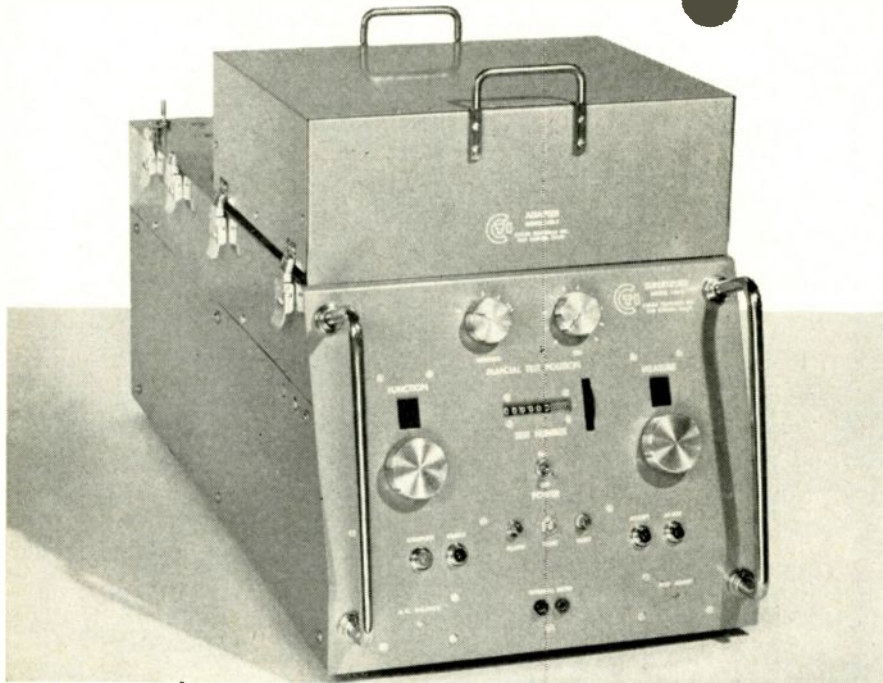
FIG. 1—Frequency-deviation indicator uses two R-C filters. Meter balance is adjusted with 200-ohm potentiometer
