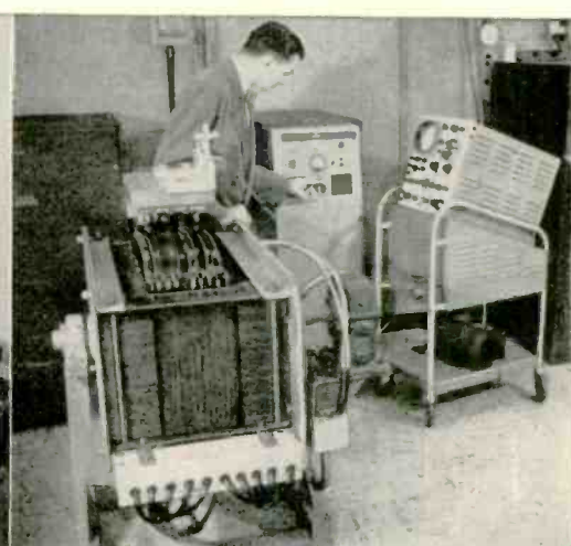
Condenser Discharge Magnetizer. Produces very large current impulse for magnetizing magnet configurations that can best be accomplished with special field shapes.
