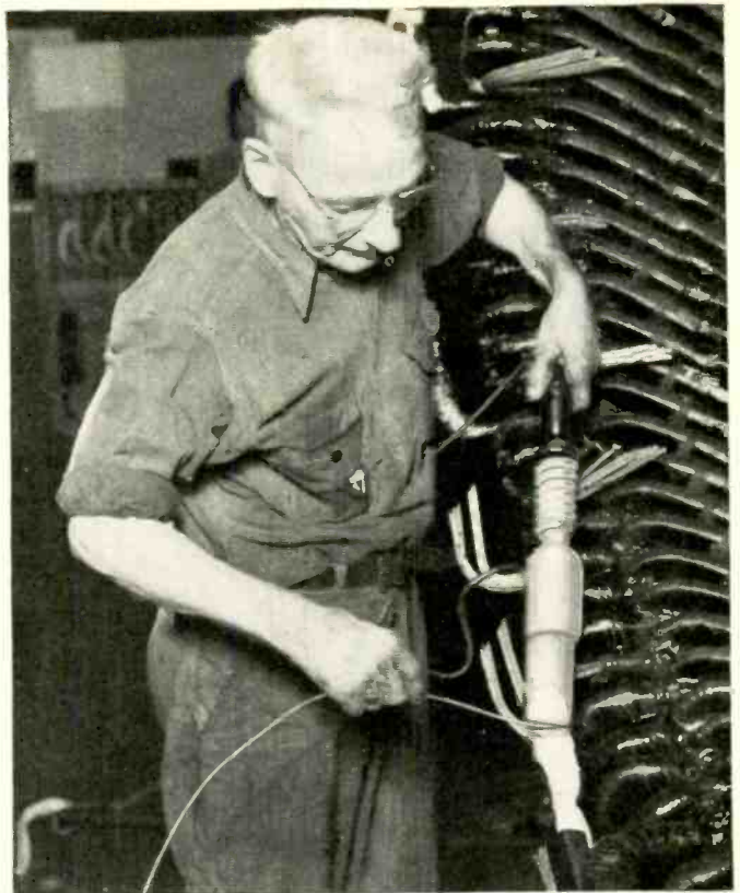
EXTRA-HEAVY-DUTY G-E IRON with long-life calorized copper tip is ideal for soldering heavy-gage cans and armature windings.
