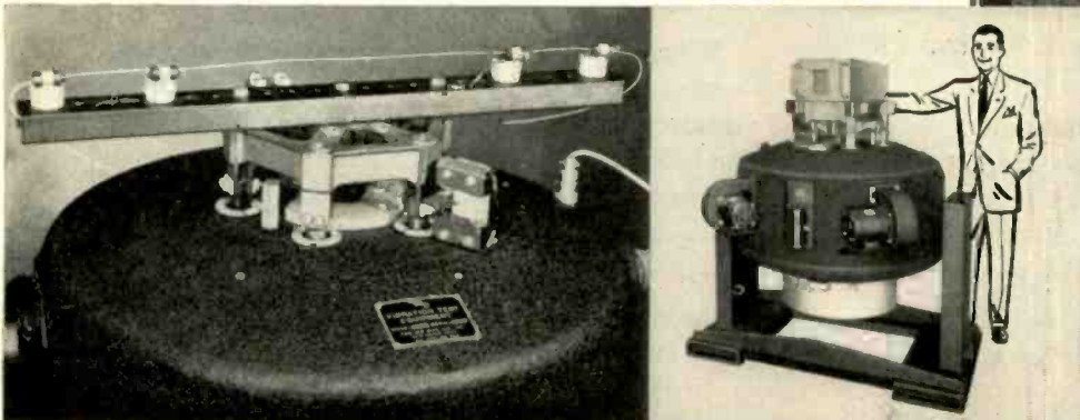
MB MODEL T-25 MC CONTROL CABINET with automatic cycling system developed to control the action of vibration exciters to a specified cycle of events, and with little or no supervision.
