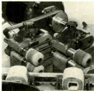
Tandem-driven wheel-type strippers with wheel guards and dust-collector covers removed. Special fiberglass wheels develop sufficient frictional heat to melt insulation, which is then wiped off by brushes. The double pass insures complete removal of insulation from stripped area. Entire width of wheels is used for stripping, so no low spots are worn in the wheels
