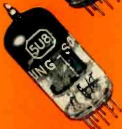
5U8 (Prototype—6U8) Heater Volts 4.7 Heater Current 0.6 A
