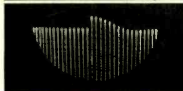
Oscillograms illustrate high-speed response of typical G-R Automatic Voltage Regulator. Illustrated at top, is sudden 1% change in 60-cycle voltage input to Regulator. Bottom oscillogram shows instrument correcting for this change in 8 cycles (0.13 seconds)
