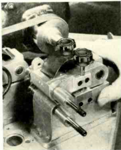
Stripper head, without wheels, being placed into position. Black knob in foreground is space regulator screw which maintains proper minimum spacing between wheels so that wire cannot be reduced in diameter or otherwise damaged. Knob at back is pressure regulator, which permits wheels to open up to receive wire and maintains proper amount of frictional heat. Antifriction plates under the arched spring allow free movement of upper spindle. Round part in base is part of dust-collecting system
