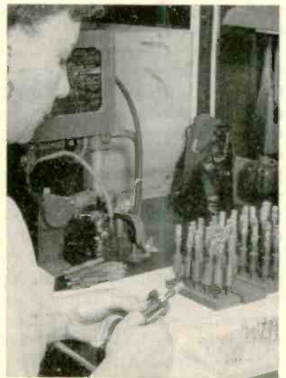
Using stretching tool on completed grid. End bands and center ring are welded to grid wires before tension is released. Completed grids are placed on plastic studs on plastic sheets in foreground. Grids in background, on wood trays, have been completed but not yet removed from mandrels
