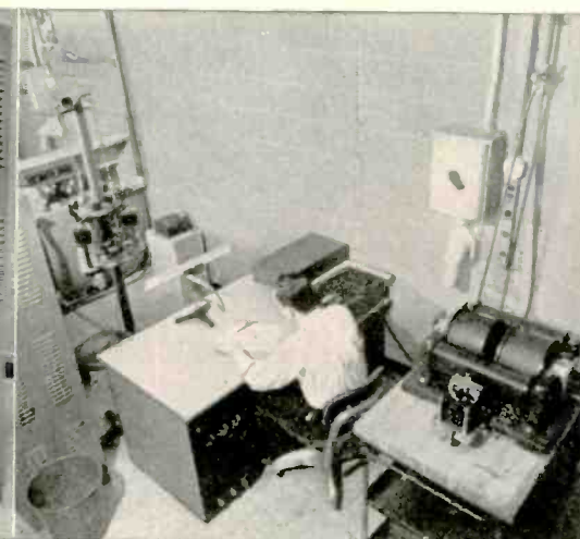
High H-Permeameter. Provides point-by-point readings of magnetizing force and induction. Control table and Ballistic Galvanometer also used for general flux measurements.
