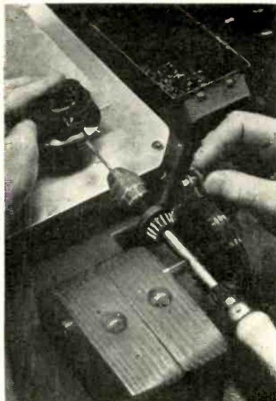
Hand drill setup for inserting setscrews in dial knobs
