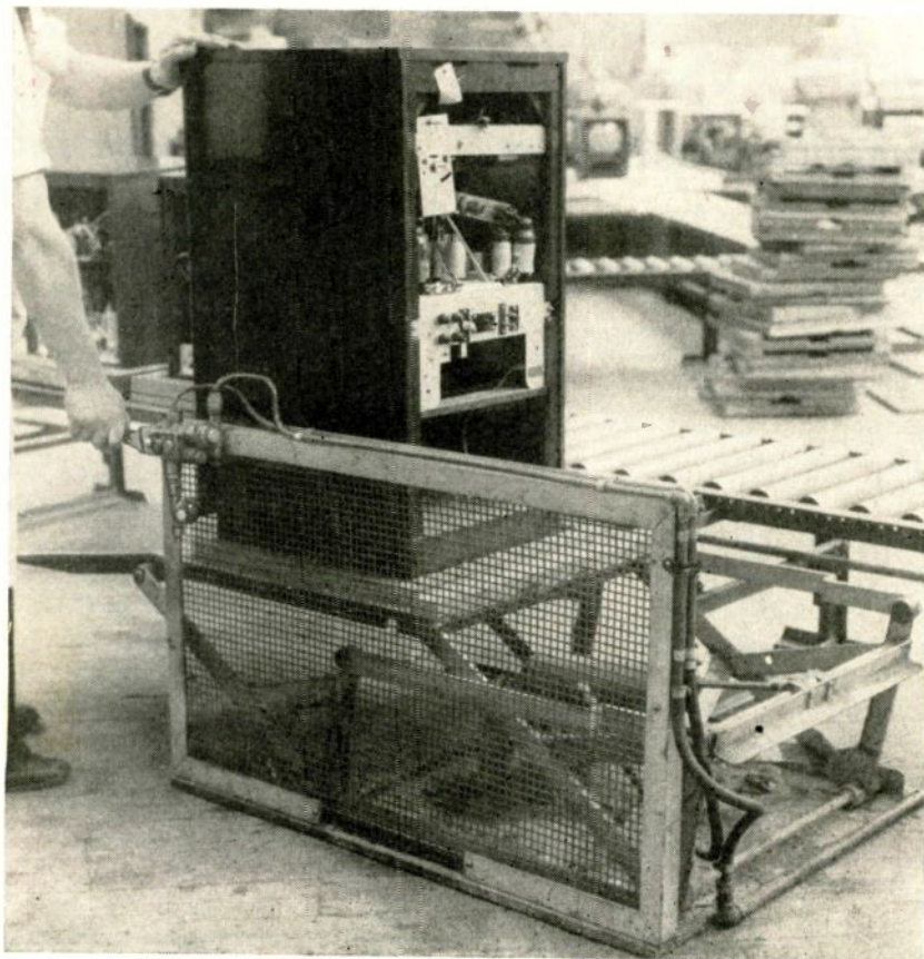
Operating lever of air valve for lift table, to lower console to floor
