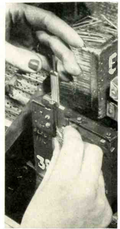
Stretched position of tool, with wedge projecting up between the two halves of the mandrel
