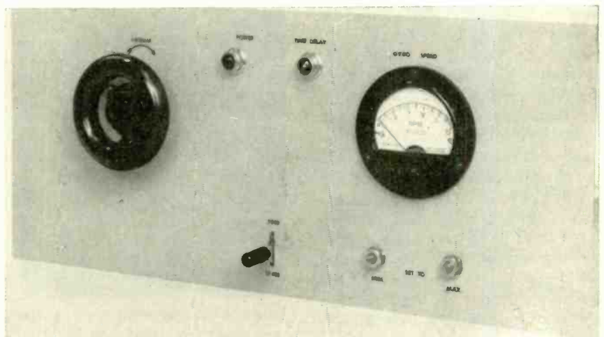
Front panel of tachometer has speed control at left. Switch at lower center injects calibration signal for setting upper and lower dial points
