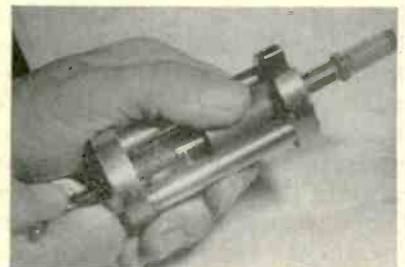
Tool used for stretching grid wires
