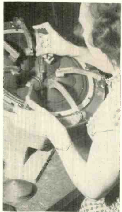
Applying cement around domes with hypodermic syringe while weighted tools hold the seven domes in position. Entire fixture rotates to bring domes into working position
