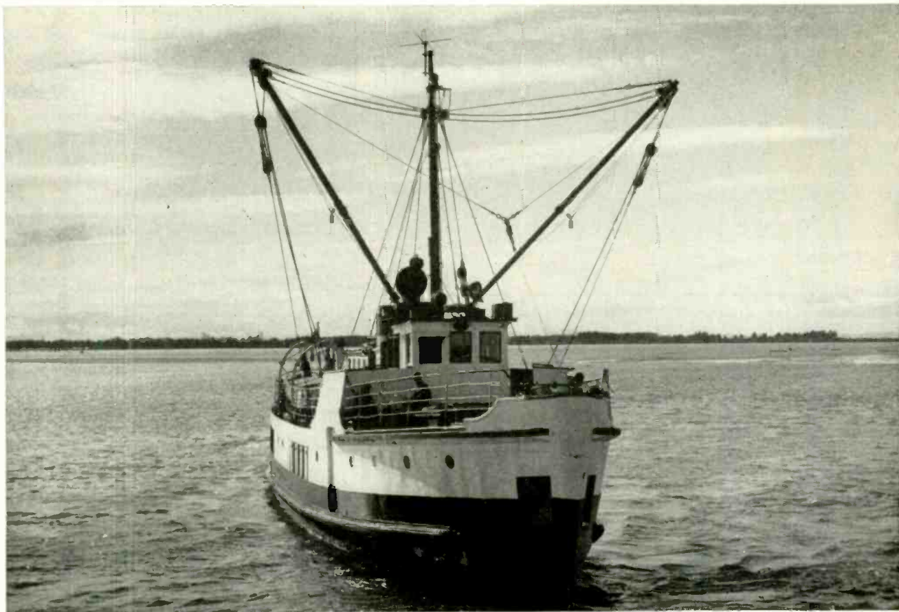
Small vessel typical of Great Lakes and Canadian west coast maritime activities requires only small antenna atop mast
