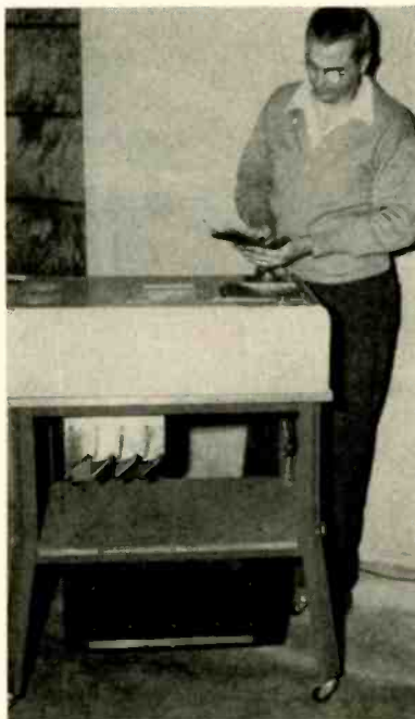
Loading pencil crayons into machine for sorting into four different diameter categories
