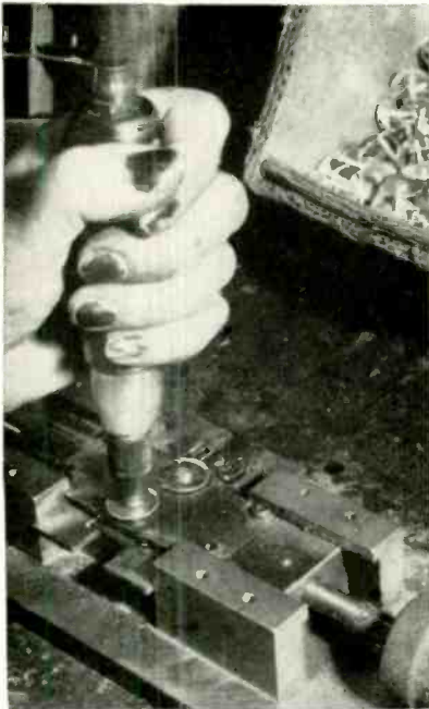
Using air driver and depth-controlling vise jaws to speed assembly of etched i-f coil strips
