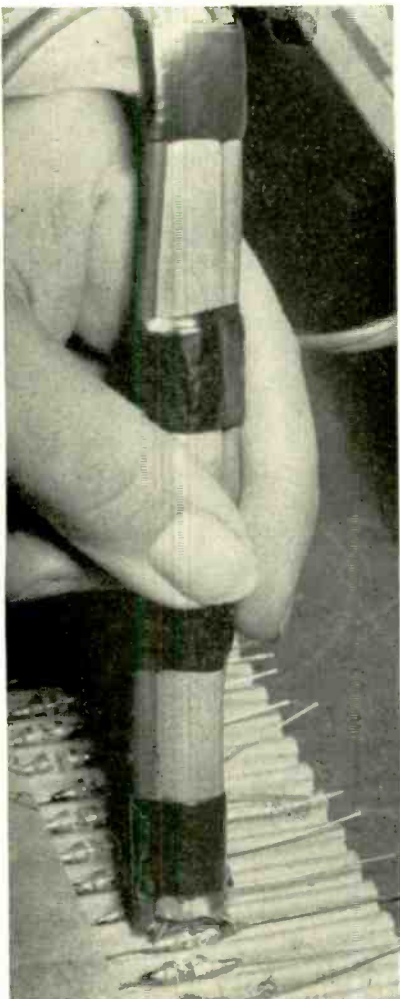
Details of improvised two-contact test prod for diodes
