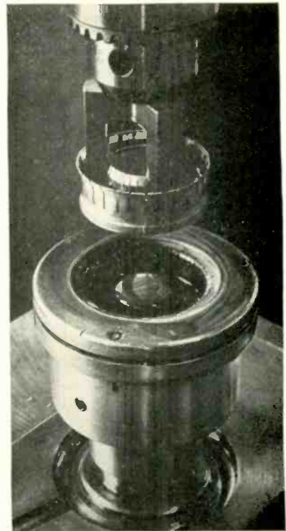
Lapping operation takes about 10 minutes on modified drill press
