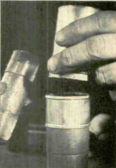
Brass ring is knocked out with series of short, sharp blows. This is a critical operation: the annealed copper crumples if hit too hard
