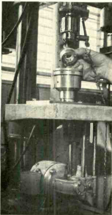
A conventional Delta drill press was adapted to lap inner and outer surfaces of contact fingers with simultaneous rotary and up-and-down motion. Reciprocating unit below table gives oscillatory up-and-down motion to specially fabricated carborundum wheel
