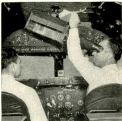
Lightweight radar for commercial airlines permits crew to see weather and obstructions 150 miles ahead
