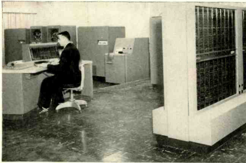
Unitized computer is made up of arithmetic and logical units, input and output equipment and memory units as required by specific application
