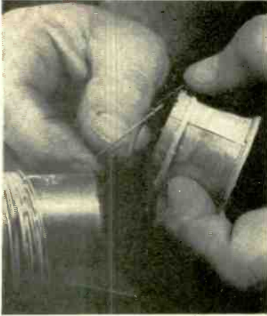
Cylinders are coated with flux and silver rings and silver solder wire positioned on either end
