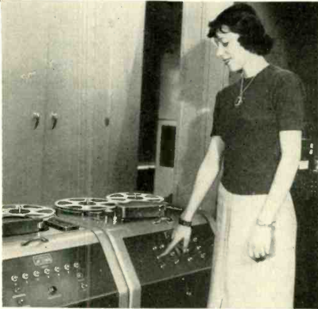
Output recorder and tape-to-punch reader shown from left-to-right. Pulses are recorded in six parallel tracks
