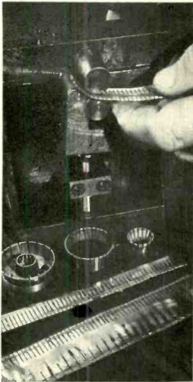
Each strip is cut longitudinally, then trimmed to size and put through another roller to shape it for assembly into a simple brass ring. Various types of contacts are made from the basic strips after this cutting operation
