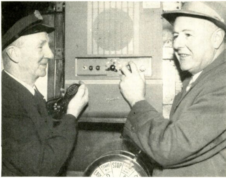
Equipment designed for nontechnical personnel (left) swings out on hinges for quick servicing in port (right)
