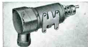
#4440 a continuous service solenoid, 24v, D.C.—3.6 amp. (starting) .42 amp. (holding)—stroke 3/8" weight 16 oz.
