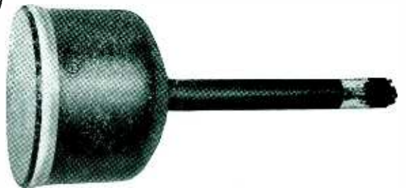
TYPE K1080P — 7-inch magnetically focused and deflected tube operating at accelerating potentials up to 30,000 volts, providing high light output with excellent resolution. Face-plate manufactured to conform to uniform standard of curvature and thickness.
