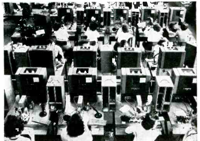
4. ORDERLY BANK OF WHISKER MACHINES is typical of modern production facilities in the new G-E plant. Quantities up to 12 million units a year can be produced here.
