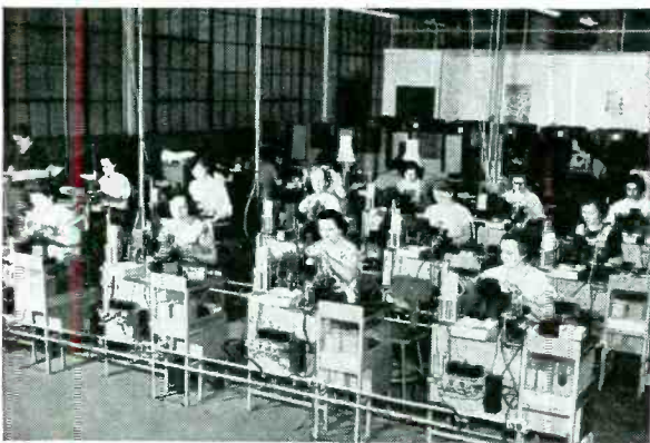
7. ASSEMBLY MACHINES turn out diodes of 12 different varieties. This process represents unusual advancement over former "hand-made" methods.
