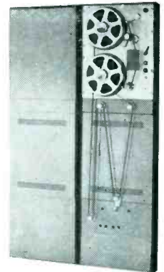
Multi-channel continuous loop reproducer. Custom construction by AMPEX.
