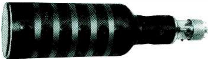
TYPE K1101P — 5-inch flat-faced tube designed for ultra-high-speed oscillography. Will provide spot writing speeds as high as 1000 in./ \mu sec. Overall maximum accelerating potential of 37,000 volts, with good deflection sensitivity.
