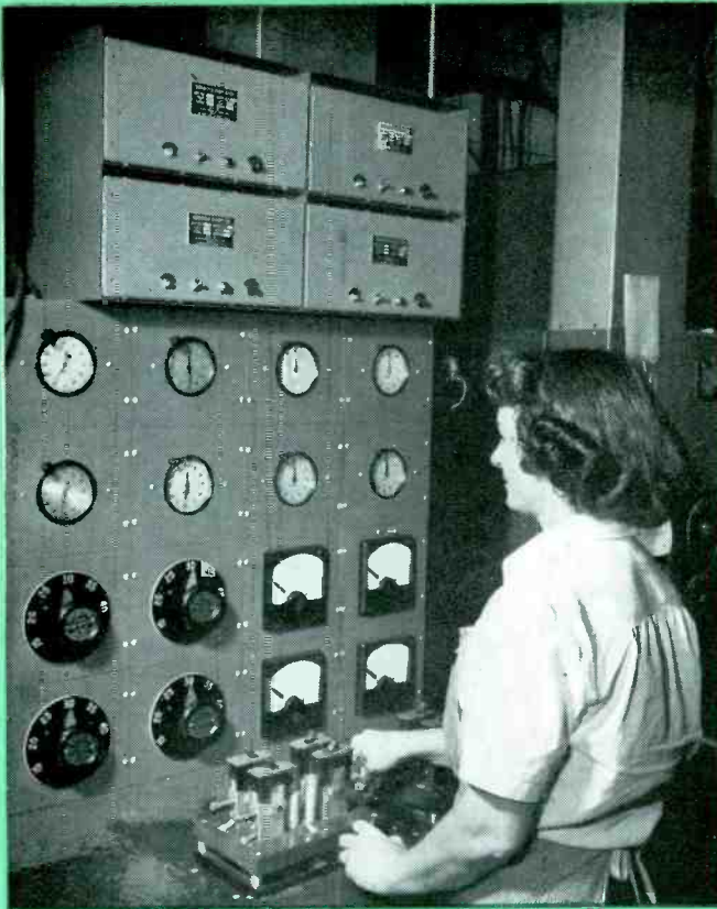
Calibration setup at Square D. Four Sorensen AC Line Regulators allow operator to concentrate on calibration procedures with assurance that line supply is a precise constant.
