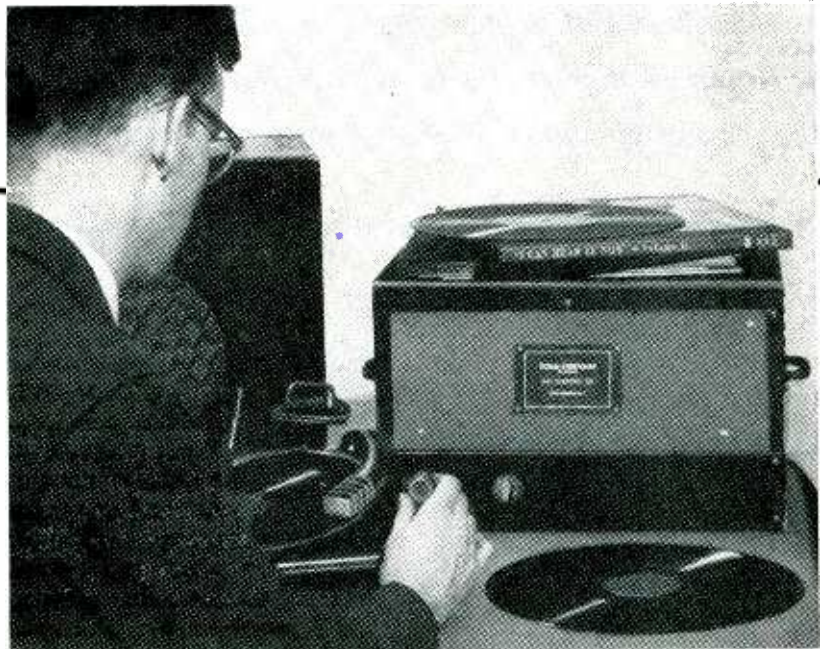
Sona-Stretcher unit, on table at right, accentuates speech mannerisms and habits. Untrained listeners using it hear more than skilled phoneticians hear in normal-tempo speech, because time available for reflection is greater than twice that with normal speech
