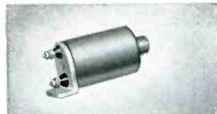
#1154 an intermittent service solenoid, 12v, D.C.—10.5 amps.—stroke 9/32", weight 13 oz.
