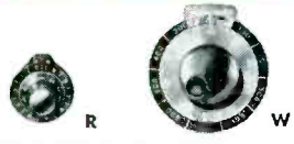
MODELS R AND W DUODIALS Each model available in standard turns-ratios of 10, 15, 25 and 40 to 1. Inner scale indicates angular position of HELIPOT sliding contact, and outer scale the helical turn on which it is located. Can be driven from knob or shaft end. R—2" diameter, exclusive of index. W—4-3/4" diameter, exclusive of index. Features finger hole in knob to speed rotation.
