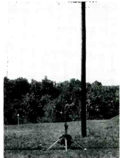
FIG. 2—After the station lands, explosive charges disengage the parachute, raise the station to an upright position, and erect a telescoping antenna
