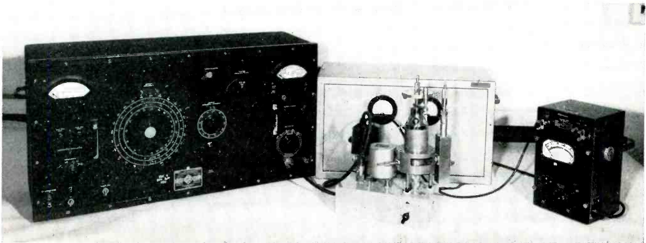
Equipment used at National Bureau of Standards for making power factor measurements on low-loss dielectrics. Measurements as low as 10^{-4} may be made to three significant figures from 1 kc to 300 mc. In the center is the micrometer electrode and coil mounted on negative resistance circuit. Power supplies and measuring instruments are shown in background. (For complete details and circuitry, see p 224)
