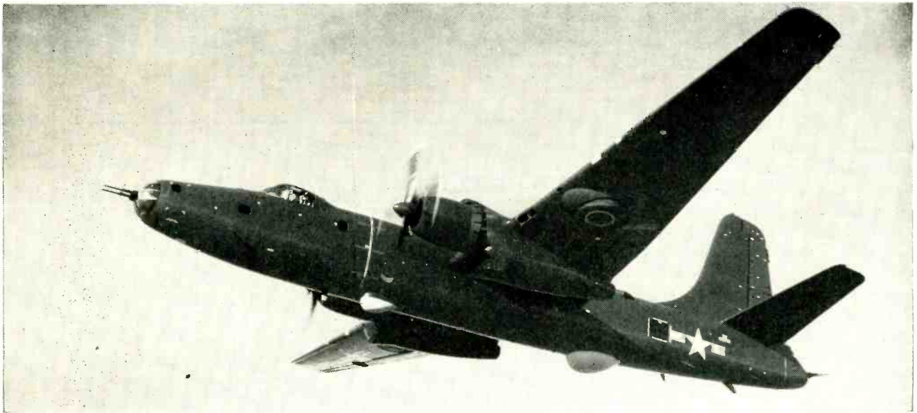
New U.S. Navy long-range patrol plane for photo reconnaissance, mine-laying and antisubmarine duties. Known as the Martin P4M-1 Mercator, the plane carries jet engines in the same nacelles with the piston engines, to provide additional power and speed for take-off and when over the target area. Both radomes face downward
