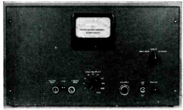
Front panel of amplifier, showing zero-center meter having 25-micromicroampere and 25-microvolt basic ranges
