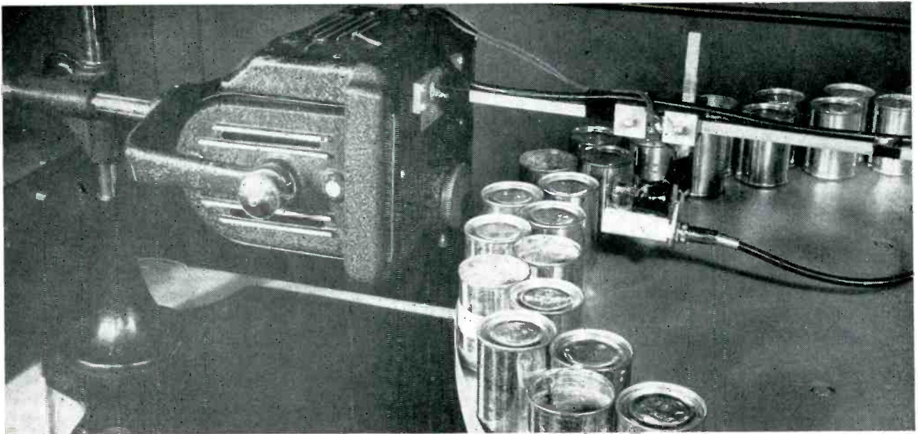
Use of cadmium-sulfide crystal in a detector for inspecting cans of baby food. Partially filled can has paper band around it as does nozzle holding crystal. Light above nozzle is illuminated briefly as low-content can passes between x-ray source at left and nozzle.
