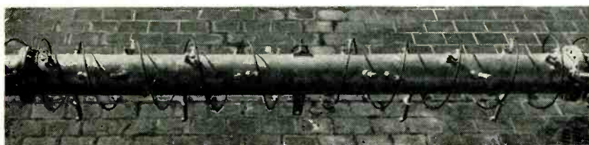
Closeup view of one bay of 500-mc sidefire helical antenna. Each turn of the helix is two wavelengths long at the velocity of propagation along the helix
