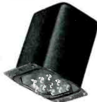
FIG. 2—After the station lands, explosive charges disengage the parachute, raise the station to an upright position, and erect a telescoping antenna
