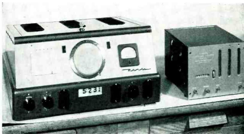
Receiving equipment used at central recording station to handle the audio sub-carriers of remote repeater stations
