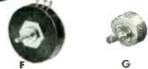
MODELS F AND G PRECISION SINGLE-TURN POTENTIOMETERS Feature both continuous and limited mechanical rotation, with maximum effective electrical rotation. Versatility of designs permit a wide variety of special features. F—3-5/16" dia., 5 watts, electrical rotation 359°—resistances 10 to 100,000 ohms. G—1-5/16" dia., 2 watts, electrical rotation 356°—resistances 5 to 20,000 ohms.
