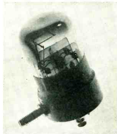
Improved vacuum-tube pickup contains stops that limit plate excursions
