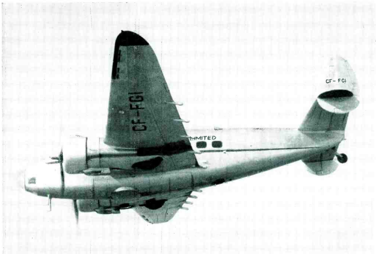
Lockheed Hudson equipped for elevation-profile surveying, with 4-foot parabolic reflector for radar altimeter mounted in bomb bay. New datum stabilizer circuit corrects for vertical excursions of plane in turbulent air, giving elevations accurate to within 10 feet
