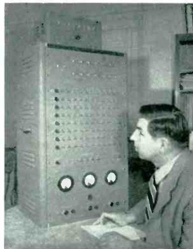
One of the authors, D. L. Gerlough, records data from the vehicle speed-distribution recorder
