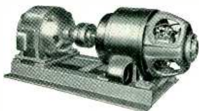
◀ 3-kw Amplidyne motor-generator set
