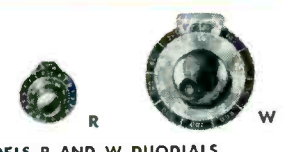
MODELS R AND W DUODIALS Each model available in standard turns-ratios of 10, 15, 25 and 40 to 1. Inner scale indicates angular position of HELIPOT sliding contact, and outer scale the helical turn on which it is located. Can be driven from knob or shaft end. R—2" diameter, exclusive of index. W—4-3/4" diameter, exclusive of index. Features finger hole in knob to speed rotation.
