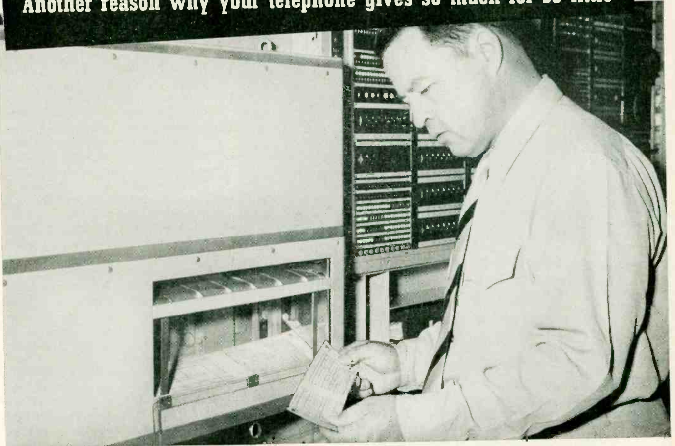
Studying punched card record of dial system operation. Each card (top) can report 1080 items
