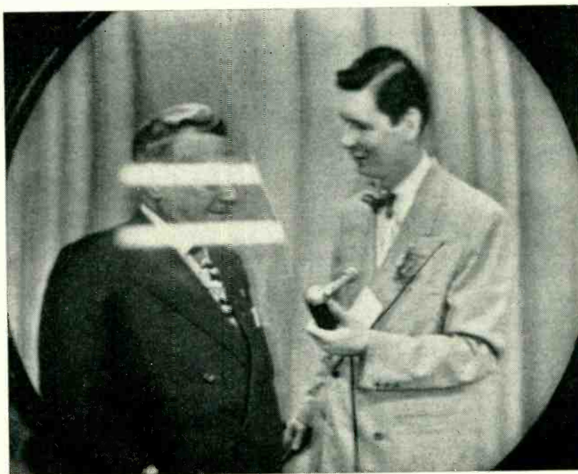
Television picture taken from 12-inch metal tube. Reflected image of fluorescent lights from untreated portion of face plate shows advantage of process
