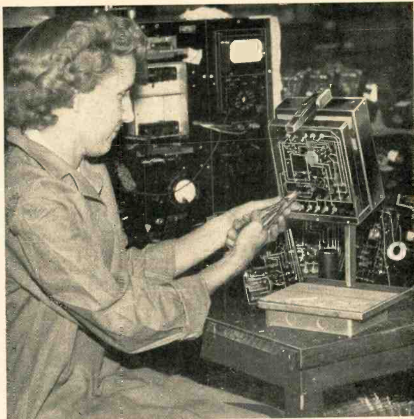
Snipping out shorting segments from stamped wiring of electronic home heating control after soldering all joints
