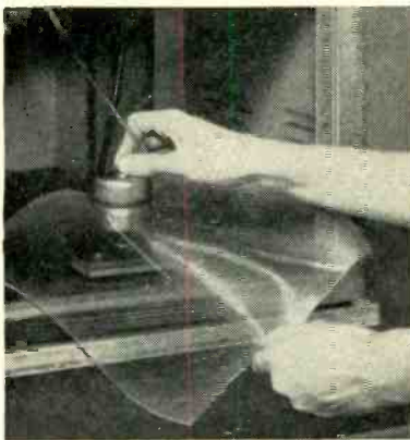
Inserting sample preparatory to voltage breakdown test on Kodapak I Sheet.
