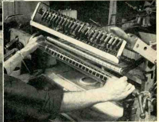
Feeding in .005-inch Kodapak I Sheet for coil-layer insulation.
