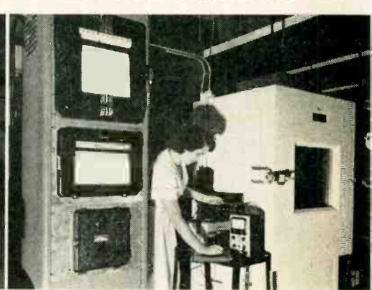
Resistance of switch insulation to atmospheric change is tested in controlled temperature and humidity chamber. Test helps avoid breakdown or leakage.
