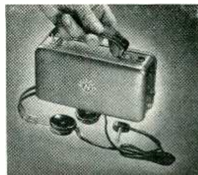
Low-cost Geiger counter weighs only two pounds
