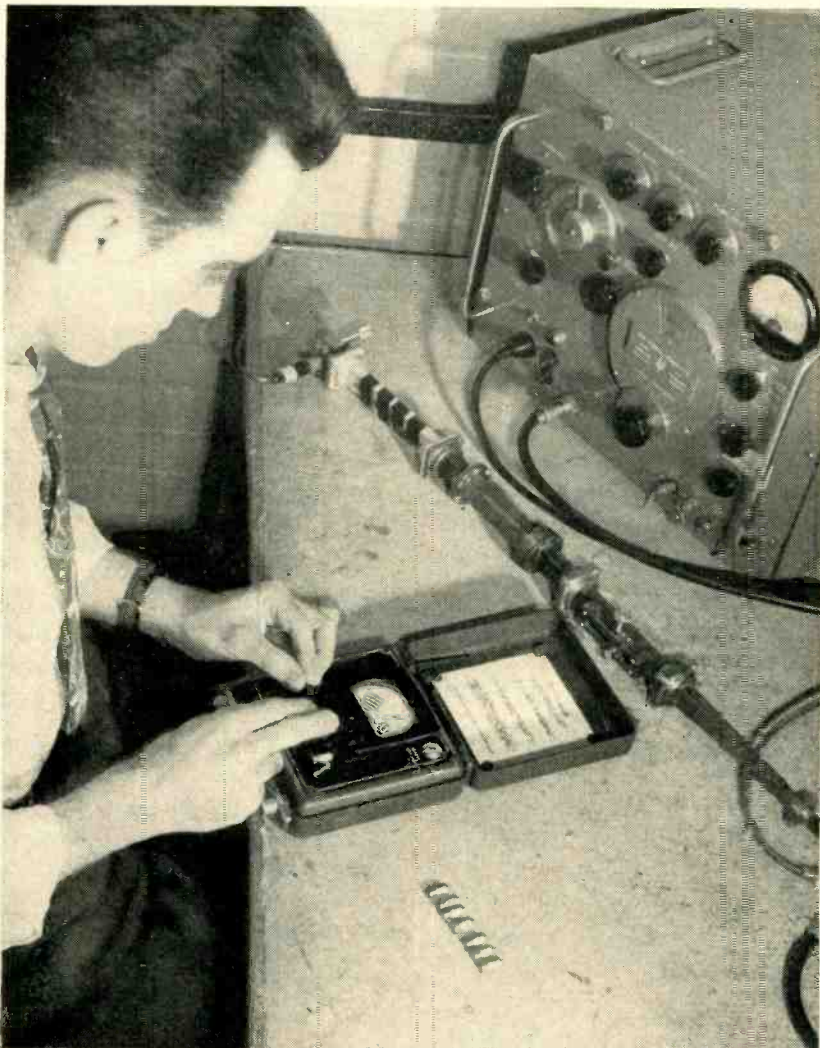
Using new d-c crystal checker to choose crystals for use in microwave measuring equipment in background
