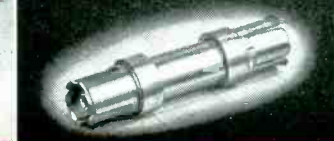
874-K COUPLING CAPACITOR — $12.00 Short coaxial line with 0.005 microfarad capacitor in series with inner conductor — transmits h.f., blocks d.c.
