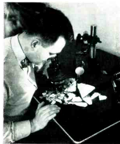
Flakes of synthetic mica are examined under a binocular microscope for structural defects, such as impurities, gas bubbles, faulty orientation and incomplete crystallization
