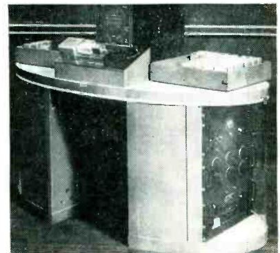
Unified test position, with electronic circuitry and electrical matching networks for filters located under console. Operator's test jig clamps to front of scope, masking all scope controls except centering, focusing and intensity
