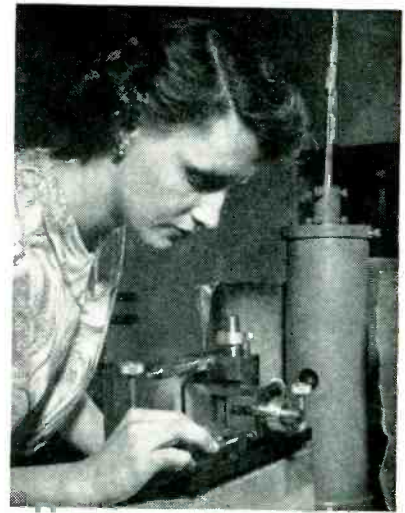
Cylinder at far right houses x-ray source for x-ray microscope capable of magnifications up to 100 diameters
