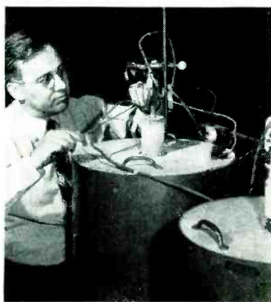
Ingredients for synthetic mica are melted in a special electric furnace at 1,400 C. Crystals form at bottom of platinum-lined crucible on cooling
