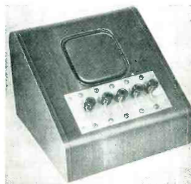
Station for automatic call selection by means of three-position switches. Extreme right switch controls talk, listen and release
