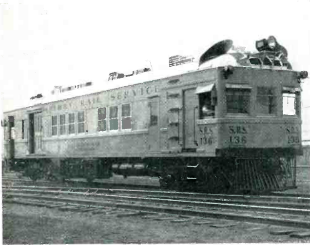
Rail flaw detector car inspects track at a rate of about 12 mph. Detector coils and current-carrying brushes are mounted on rear carriage
