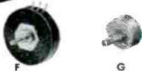
MODELS F AND G PRECISION SINGLE-TURN POTENTIOMETERS Feature both continuous and limited mechanical rotation, with maximum effective electrical rotation. Versatility of designs permit a wide variety of special features. F—3-5/16" dia., 5 watts, electrical rotation 359°—resistances 10 to 100,000 ohms. G—1-5/16" dia., 2 watts, electrical rotation 356°—resistances 5 to 20,000 ohms. — Ask for Bulletin 105 —
