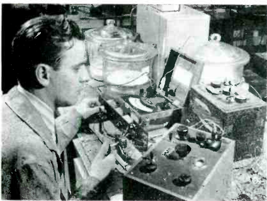
Constant checking makes sure CRL switches give you desirable uniform low contact resistance. Here an engineer tests resistance by running 1 ampere through contacts.
