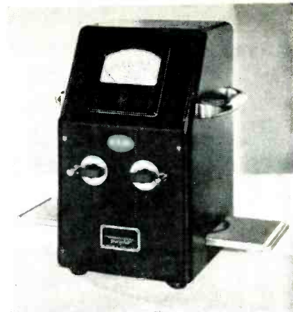
Radioactive thickness gage as designed for single measurements in laboratories
