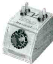
MODELS A, B, & C HELIPOTS A—10 turns, 46" coil, 1-13/16" dia., 5 watts—resistances from 10 to 300,000 ohms. B—15 turns, 140" coil, 3-5/16" dia., 10 watts—resistances from 50 to 500,000 ohms. C—3 turns, 13-1/2" coil, 1-13/16" dia., 3 watts—resistances from 5 to 50,000 ohms. — Ask for Bulletin 104 —
