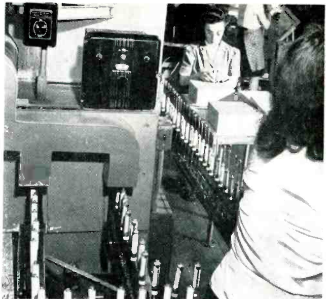
DRUG INDUSTRY Oven temperature of machine for applying and baking decoration onto collapsible metal tubes is controlled electronically by unit in center. Blank tubes enter on conveyor at lower left
