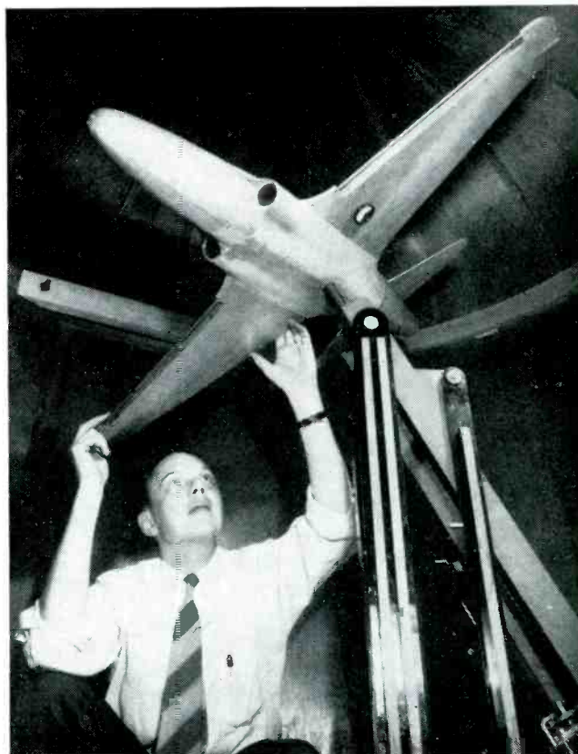
Jet aircraft model used at Cruft in connection with aircraft antenna research project
