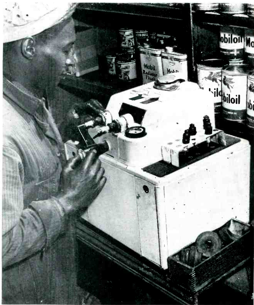
Typical spark-plug testing machine employing a compression chamber in which the plugs are fired
