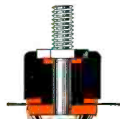
Silicone gaskets and plastic stand-offs used with capacitors rated 2000-v d-c and lower.
