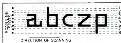
FIG. 1—Eight scanning spots are used in the letter reader
