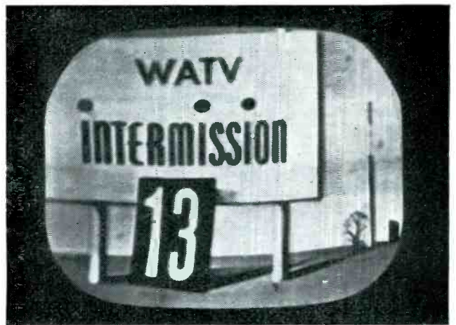
Improvement in channel 13 reception after adding two-stage booster and erecting a good high-band antenna
