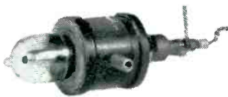
Raytheon magnetron used in the "Rad-range" for swift cooking by microwaves.
