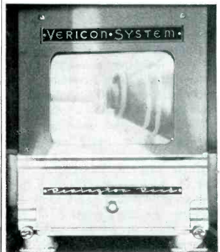
Safe in a protective shelter, the viewer sees this picture of the defusing operation on the screen of the c-r tube
