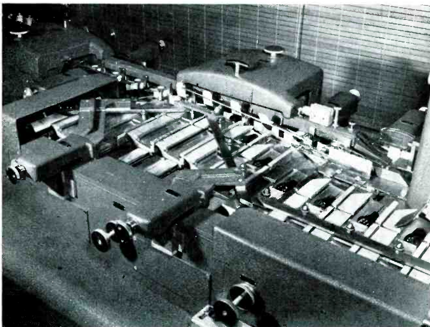
This GE automatic tube cartoner feeds flat folding cartons from a magazine, makes up the carton, inserts a tube, closes the top and bottom tuck-in flaps, and imprints the tube type designation on the top panel of each carton in one continuous automatic operation at the rate of 160 cartons a minute
