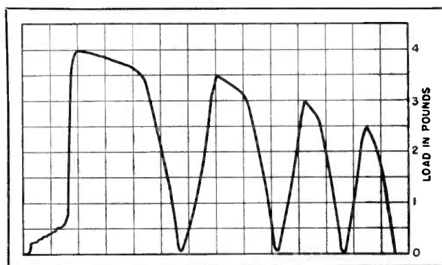
FIG. 6—Record for repeated loading of paper, illustrating magnification ratio of 50 to 1 as applied to inextensible material
