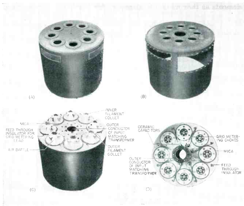
FIG. 3—Plate cylinder (A), grid cylinder (B), filament cylinder (C), and underside of filament cylinder top plate (D) used in the amplifier
