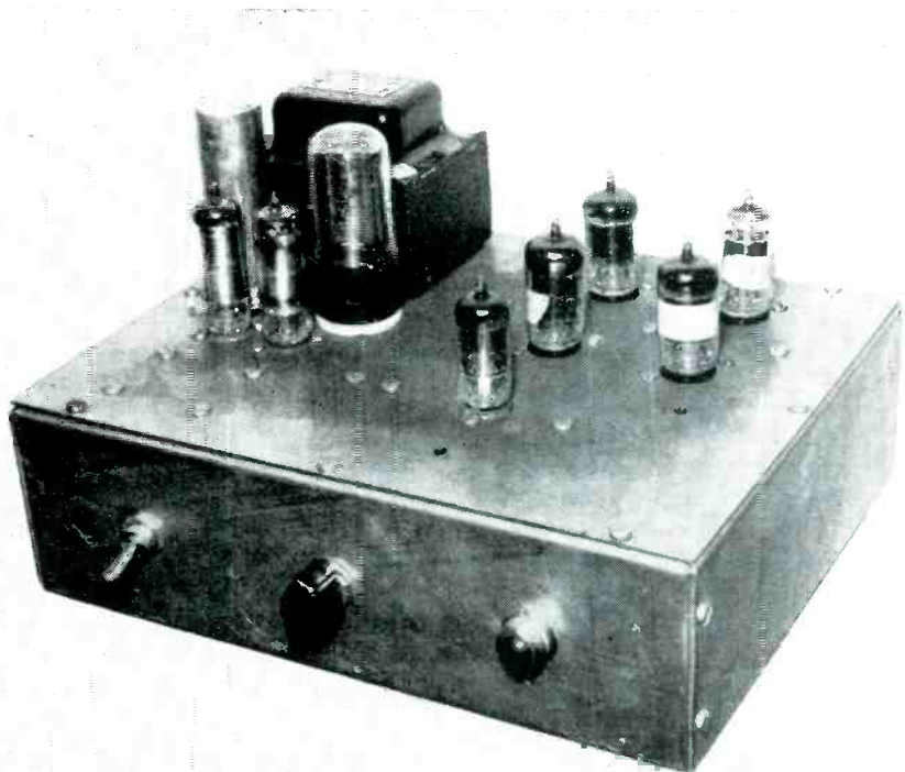
Top view of wide-range audio-frequency generator. Useful frequency range is 150 cps to 15,000 cps
