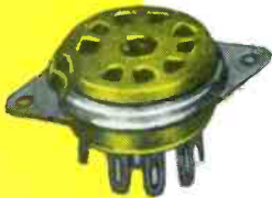
Cinch Noval Nine Prong No. 53F12617 Saddle Type—Mica Filled Molded with .093 mtg. hole 1 1/8" mtg. center
