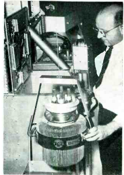
Hoist and sling hold the 5592 tube ready for lowering into the tube well in the background. Two of these tubes form the 50-kw final amplifier
