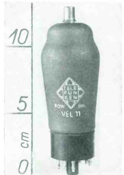
The VEL11 encloses two pentodes, one for grid detection and one for power amplification, in one envelope. Dark sprayed shield improves tube's heat radiation
