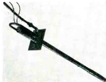
Seven-foot air-purged sighting tube is immersed in molten metal for temperature measurements
