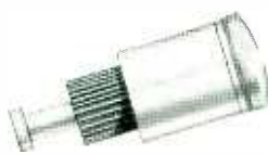
Combination lug. Screw on top . . . solder terminal below. Designed as a rugged swaged terminal for top & bottom wiring applications.
