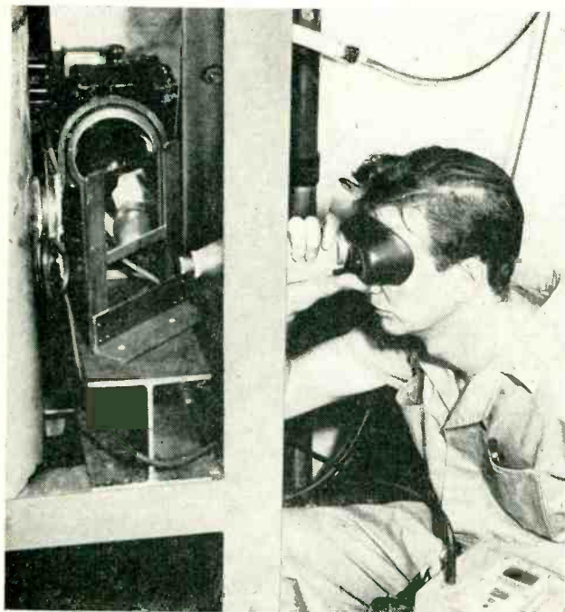
Photoelectric sensing unit on 15-kw electric furnace. Operator is checking temperature with optical pyrometer through peephole. Phototube views flame in 45-degree mirror
