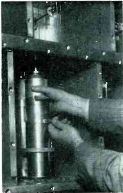
FIG. 6—One of the class-B stages of the G-E transmitter, showing method of removing air-cooled tube from anode tank. The circuit is tuned by an L-shaped flipper
