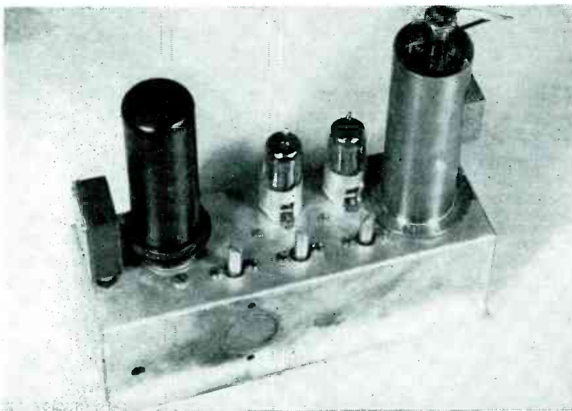
FIG. 7—Frequency multiplication of 48 is accomplished in four-tube transmitter
