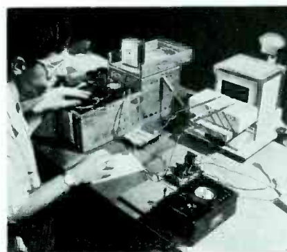
Research students measure and tabulate the temperature-resistance characteristics and resistivities of the samples
