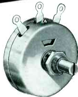
TYPE M potentiometers and rheostats have a normal rating of 4 watts, are insulated for 1,000 volt DC breakdown to ground, and are also available in a complete line of T and L Pad Attenuators. Diameter 1 \frac{1}{2} ".
