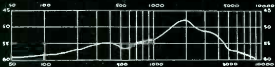
TYPICAL FREQUENCY RESPONSE AT HIGH IMPEDANCE
