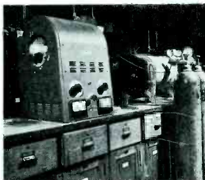
The test bars are fired at high temperature for several hours in a hydrogen atmosphere to complete the processing
