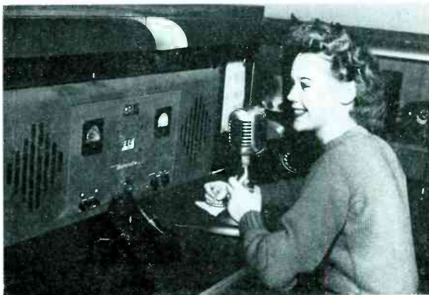
Telephone Exchange, Inc. dispatcher with remote control unit and loudspeaker. Incoming and outgoing calls are channeled through her land wires
