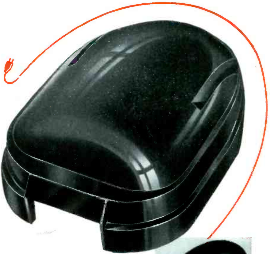
Above, top side view of motor dome as molded for Miracle Electric Company, Chicago 3, Illinois. The miniature reproduction to the right shows the dome's intricately designed wall separations. Item was compression molded of phenolic. Color—maroon.
