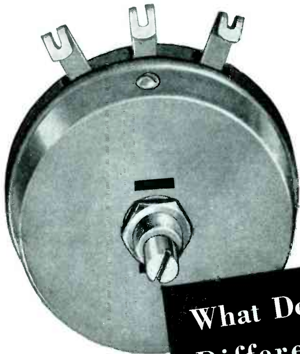
The TYPE E potentiometer is rated at 7 watts. Widely used in precision instruments, resistance bridges and other circuits requiring accurate settings. Diameter 2 \frac{1}{2} ".
