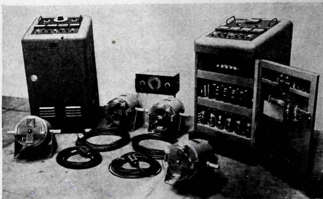
Complete vibration exciter equipment for driving the two pairs of electromagnetic shaker on the floor. Power amplifier cabinet at left contains plug-in a-f oscillator for controlling exciting frequency of shakers, while cabinet at right contains plug-in phase shifter for varying phase relationship of signals fed from a-f oscillator to the two power amplifiers. Extra a-f oscillator on box between cabinets is plugged into cabinet at right in place of phase shifter when it is desired to use the two amplifiers independently, each with its own controllable a-f oscillator and pair of shakers
