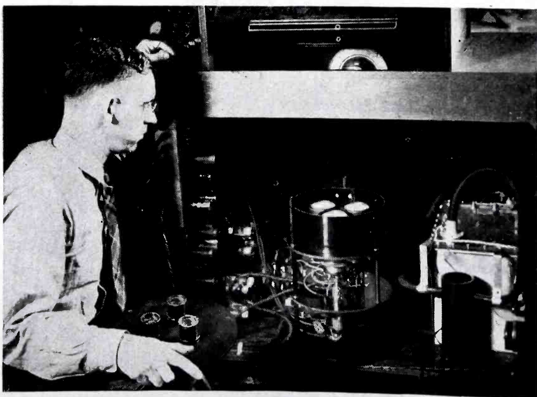
The Trinoscope consists of three cathode-ray tubes that project the colors upward to the screen in the top of the cabinet. Karl Wendt, research engineer, holds the triple lens assembly used to focus the beams
