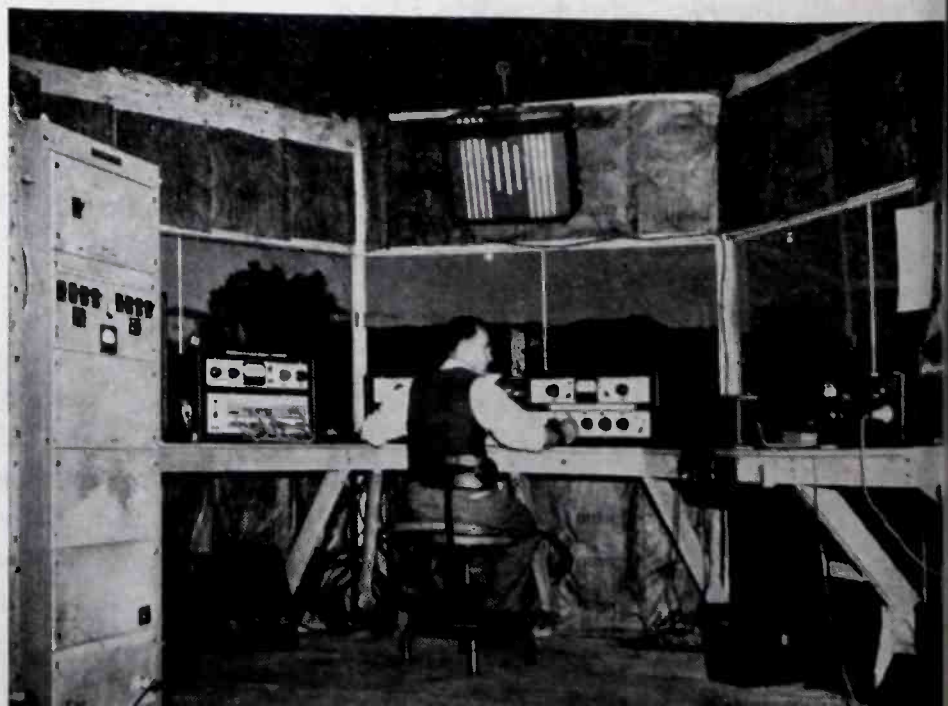
FIG. 3—(Left) Exterior of the Vancouver Diamond Jubilee show control tower. The far windows enclose the director's room, the near windows are those of the sound control room, and the cubicle between the two rooms was used by a commentator. The speaker (not part of the main sound system) was used to convey directions to the stage. (Right) Interior of the sound control room showing left to right, one corner of the power amplifier bays, master control unit, the two mixers, and the two turntables
