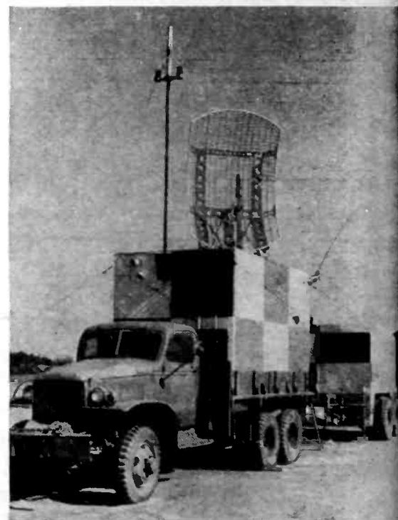
Bendix airport surveillance system, employing high-definition search radar as an auxiliary to GCA and an aid to traffic control. Center frequency is 2,880 mc, and antenna rotation rate is 30 rpm. This equipment was demonstrated to PICAO delegates at Indianapolis
