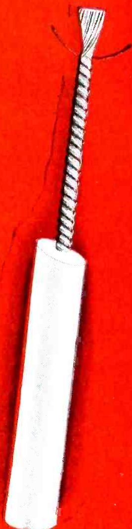
A section of the heating element used in Simmons Electronic Blanket, showing water-proof insulation and rayon core. Light wire is D-H 99 Alloy, dark wire copper.
