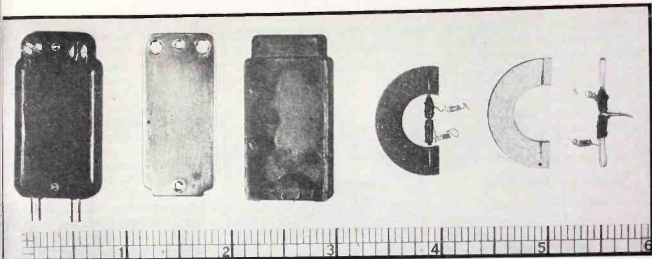
Parts of torsional magnetostriction pickup fit into small cartridge shown at the left
