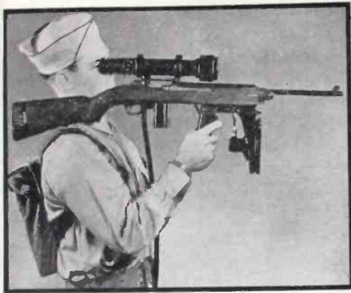
The night sight mounted on a 30-calibre carbine, showing the sighting and aiming telescope (receiver) above the barrel, the "near infrared" lightsource (transmitter) below it, and the powerpack on the marksman's back
