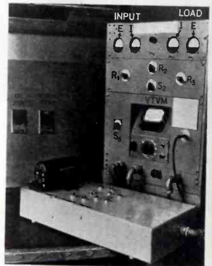
Fig. 2—Panel meters and controls of the dynamotor tester
