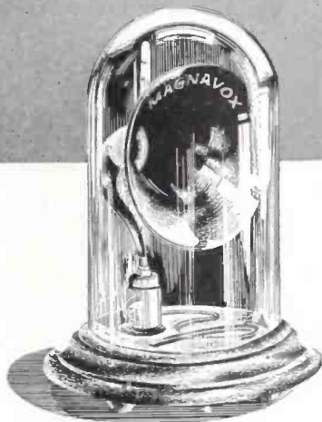
The Electrodynamic Speaker —the first voice of all modern sound reproduction.
