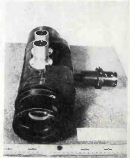
The infrared receiver for tanks viewed from the sighting position. High-voltage terminals are at top
