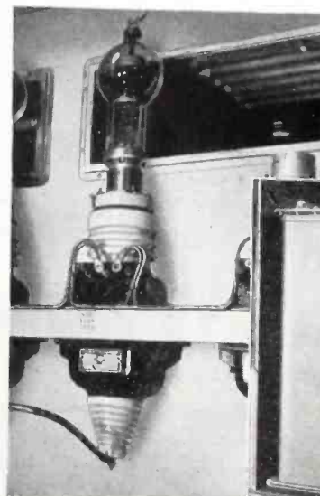
↑ Front panel view, rectifier section, showing AmerTran Filament Transformers.
