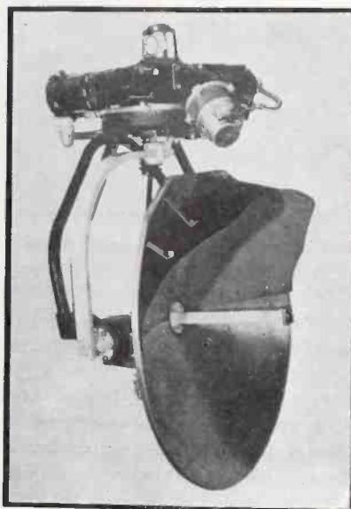
Antenna system of Western Electric APQ-13 version of H2X bombing radar. Azimuth selsyn is at top right, azimuth motor at left
