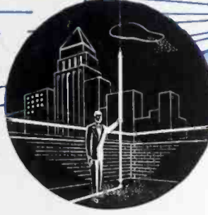
1938 Coaxial antenna for ultra high frequency communications, designed by Bell Laboratories, gave increased signal strength. Widely used in police radio systems.
