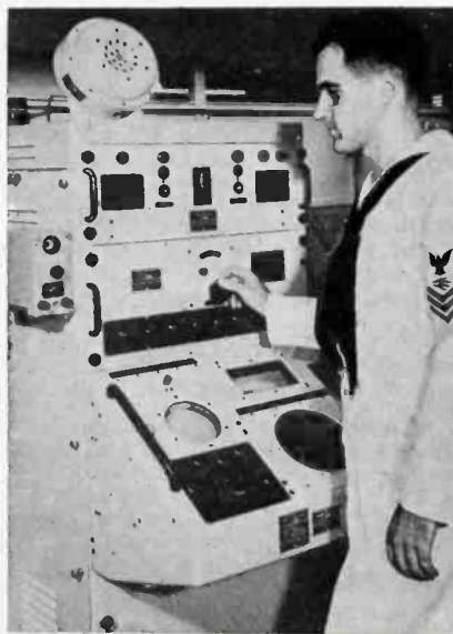
Indicator console of modern echo ranging sonar having built-in bearing deviation indicator to help operator keep the projector trained on a moving submarine
