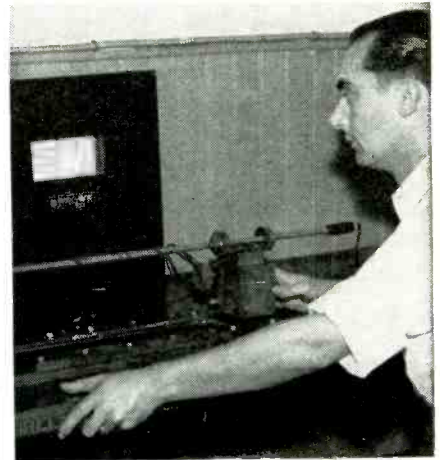
The electronic bore gage utilizes direct contact to measure cylindrical interiors with an accuracy of 0.00005 inch
