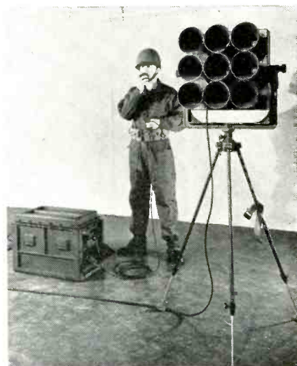
Amplifier and loudspeaker unit of the beachmaster announcing system. Made by Western Electric, it was used by the Navy during the invasions of Iwo Jima and Okinawa
