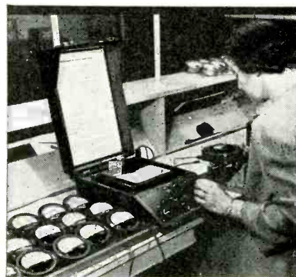
The meter tester in use on production line. Instructions for use are lithographed on brass plate inside the cover for permanence and convenience
