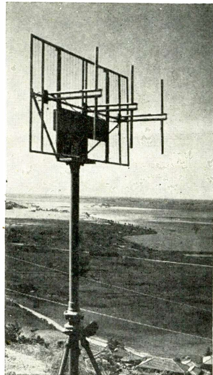
Antenna of an IFF, Identification Friend or Foe, set as installed on Okinawa for part of the radar warning system
