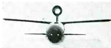
Model of gorgon II-C, a guided missile that carries 1,000 pounds of explosive to its target at 400 miles per hour. The ring at the top is the jet-propulsion engine
