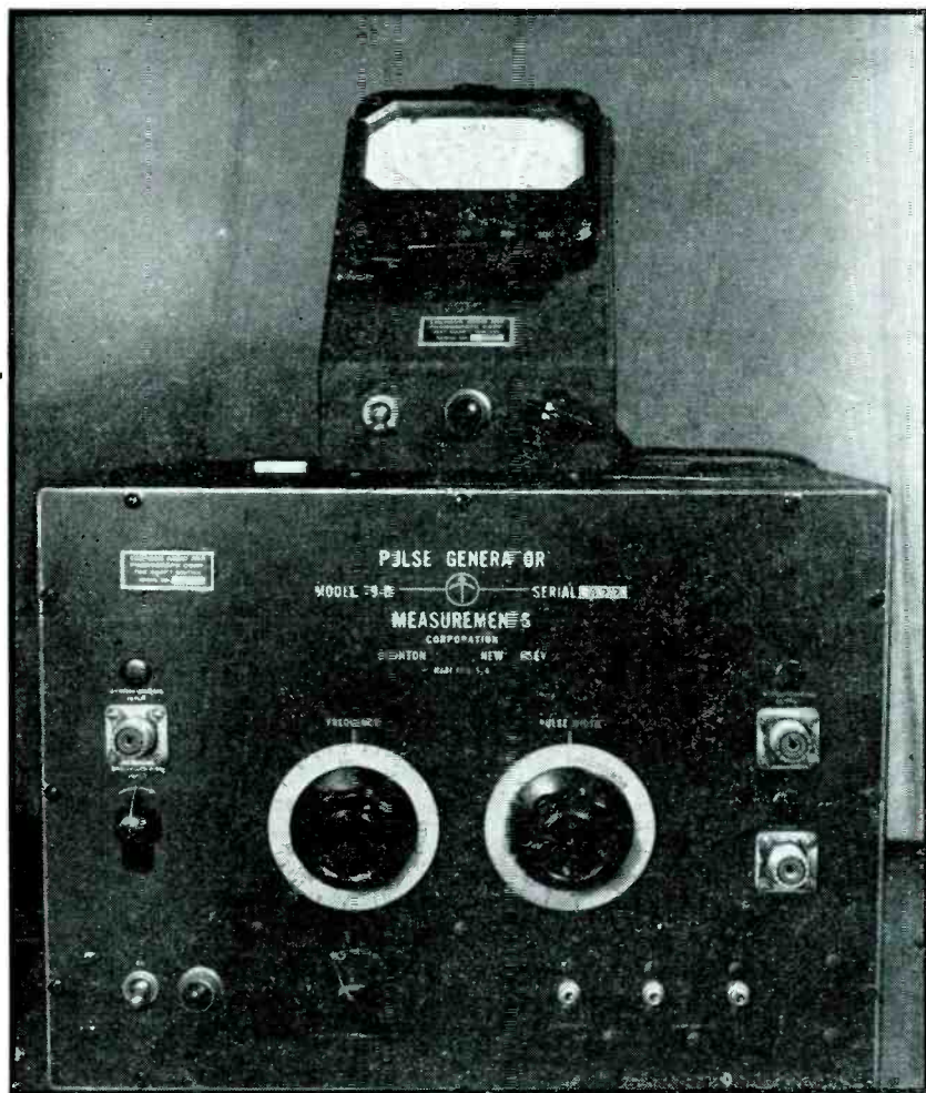
On top of the pulse generator used to check theoretical conclusions is a peak vacuum-tube voltmeter of the type analyzed in this article
