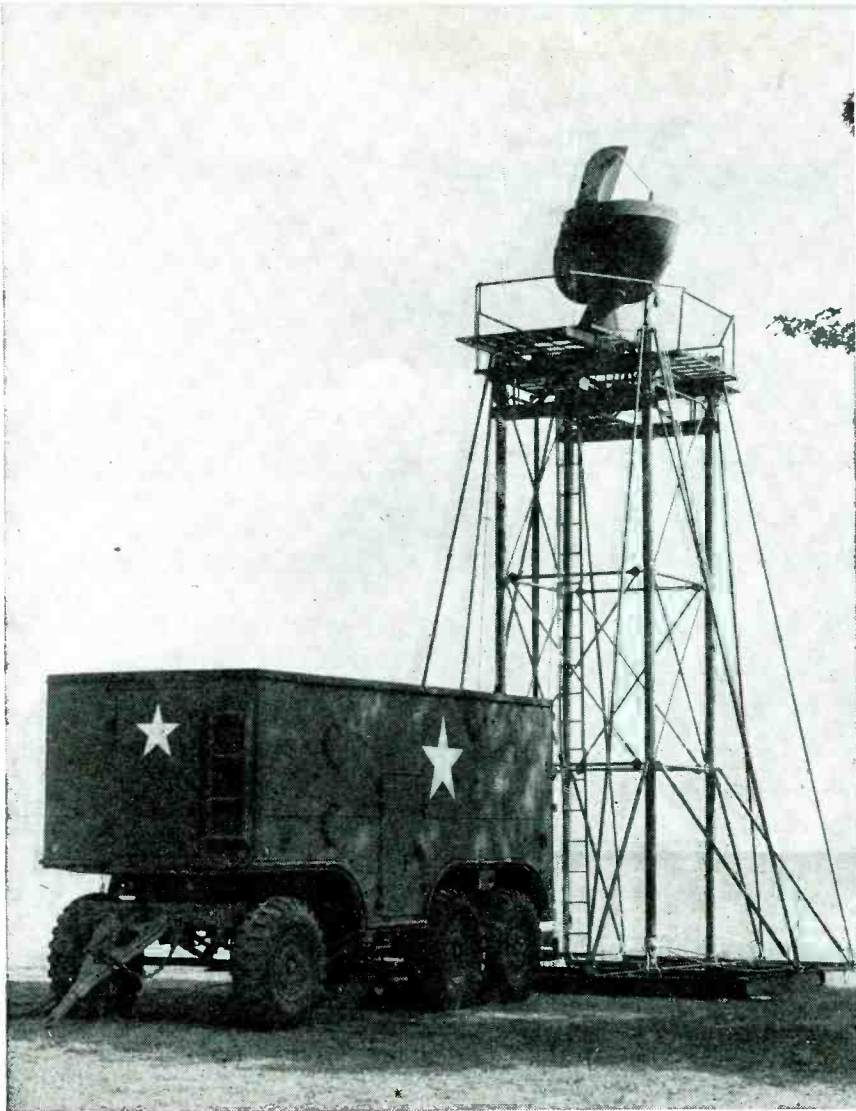
AN/MPG-1 trailer, tower and radiator. The "bath-tub" radiator is elevated within the tower to raise it to operating position
