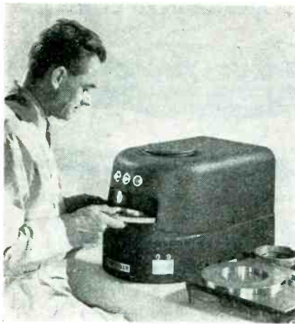
Piston rings are inserted in a master ring and rotated under a light beam for electronic checking of true and width of gap
