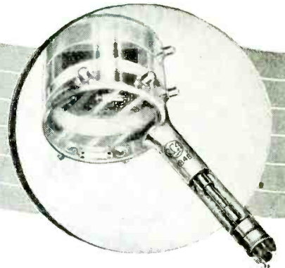
1. THE ICONOSCOPE — The "electric eye" of the television camera. Developed by Dr. V. K. Zworykin, RCA scientist, and brought to a high degree of perfection by RCA engineers.
