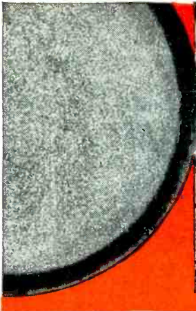
Fig. 1. Macrostructure—Dark circumferential area is the hardened portion of the steel.
