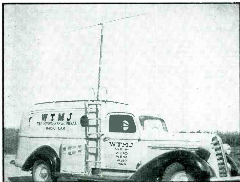
FIG. 3—View of the field car with the telescopic antenna raised. The antenna pivots on a bearing inside, permitting orientation for maximum signal
