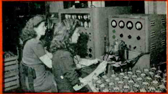
QST-2 —A unique test is applied to every United tube to assure noise-free operation.
