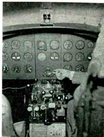
API installed on a typical aircraft instrument panel to provide continuous readings of latitude and longitude
