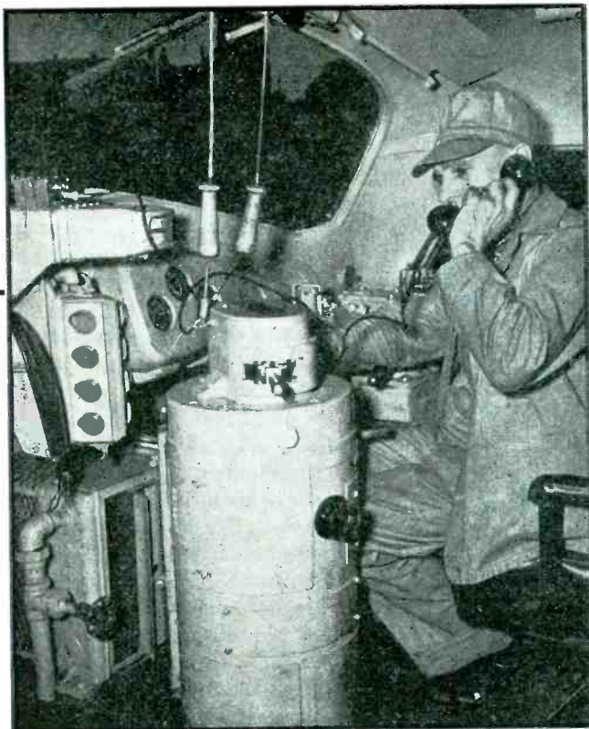
Freight engineer using a radiophone in the cab of a diesel locomotive
