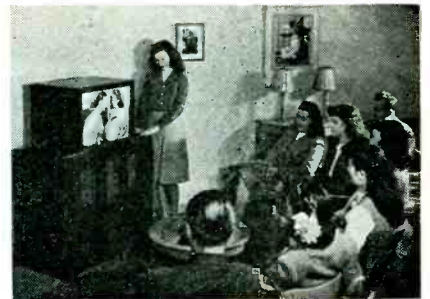
Large-screen television receiver of advance development type demonstrated in New York recently. Picture is 16 x 21¼ in., and appears on a treated plastic viewing screen
