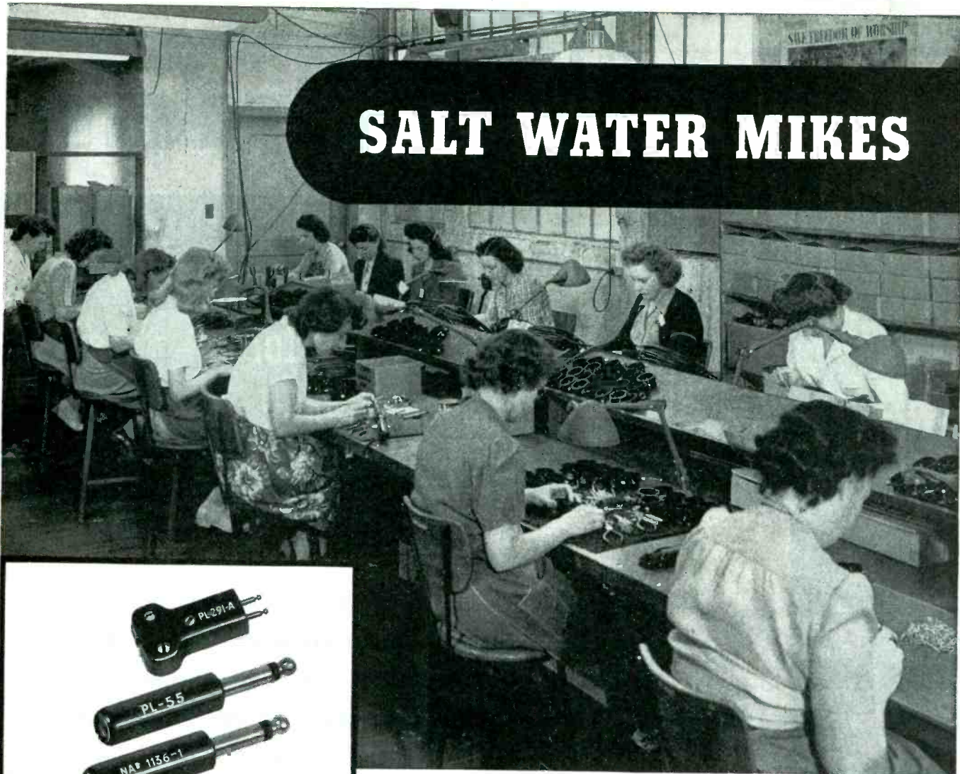
Marine microphone assembly. Plastic and metal parts designed, made and assembled by Remler to meet Navy and Merchant Marine specifications.
