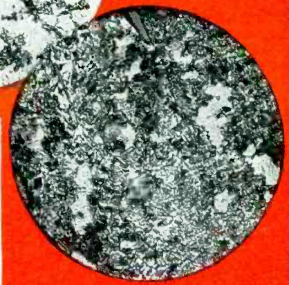
Fig. 4. .112" Below Surface—structure is troostite-sorbite with patches of martensite. This area is in zone close to core structure.
