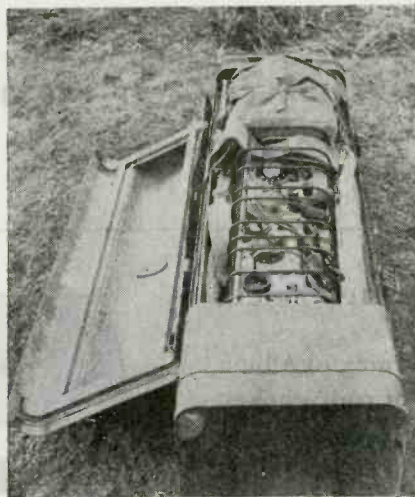
A Number 22 Wireless set tucked in its container and ready for service with British airborne troops
