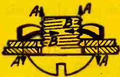
A Self-locking PALNUT Type WT replaced more expensive jam nut and lockwasher on this volume control, saving in cost of material and labor.
