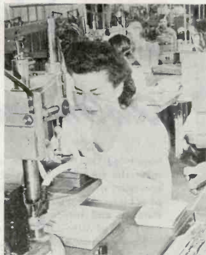
Vertical-bar-type grid elements are wound on a mandrel and spot welded by girl operators in the Eimac tube plant
