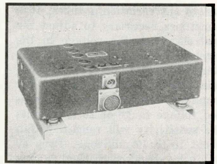
Power unit assembly, operating directly from plane's storage battery
