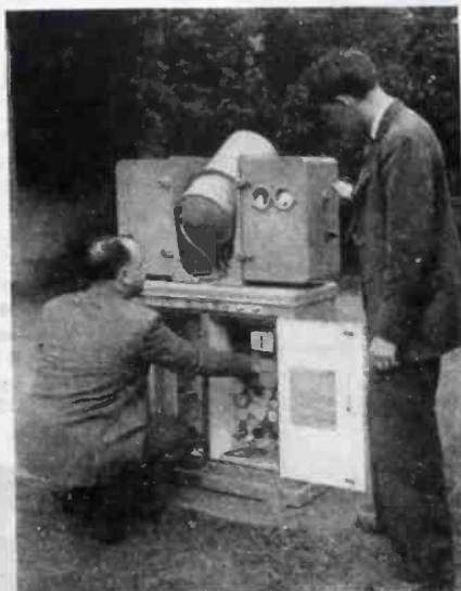
Electronic equipment of the Novalux ceilometer. The scanning drum may be operated by a hand crank at the side
