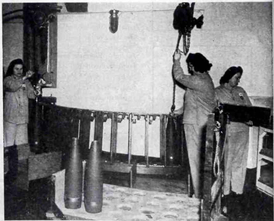
View of the motorized ring that carries 155-mm shells into the adjoining room for x-raying of TNT cast. The girl at the left is loading shells onto the ring and the girl at right is removing them as they emerge from an aperture in the concrete wall of the exposure room
