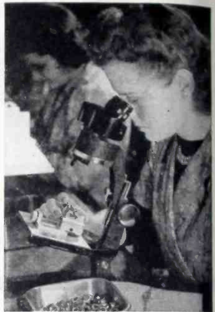
Vital bearings for a Mark XIV Gyro Compass being inspected with a Spencer Stereoscopic Microscope.
