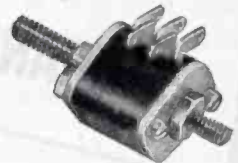
"Coprox" Model CX-4D4F23, a full wave rectifier with high conversion efficiency, for electronic control work. Rated at 5 volts A.C., 40 milliamperes D.C. continuous. Fully enclosed. Mounts on a single screw.
