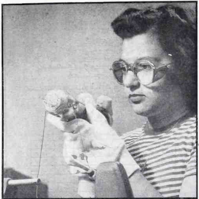
Shrinkage analyst uses a hot-wire glass cutter to open a defective cathode-ray tube for investigation
