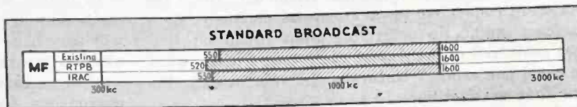
FIG. 1—Standard broadcasting would get three new channels on the low-frequency end, if the industry-sponsored RTPB had its way. The IRAC proposal representing the viewpoint of government departments would provide only two, keeping clearer of the SOS frequency
