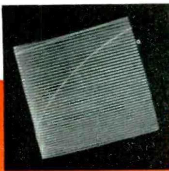
Pattern used for measuring light output by means of photoelectric cell. Frequency—60 x 2940 cycles.
