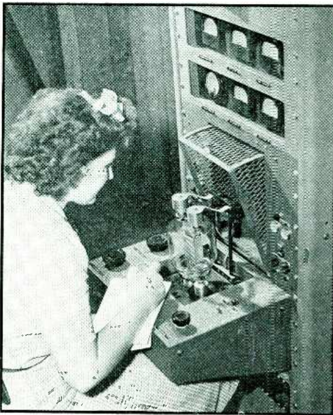
Operator preparing to apply a static quality test to a type 833A transmitting tube
