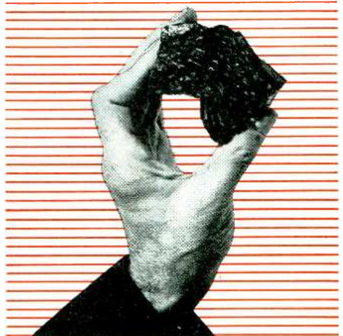
THIS 4-OZ. PIECE of plastic was thoroughly softened for molding in about 15 seconds by an RCA 2000-watt electronic generator.
