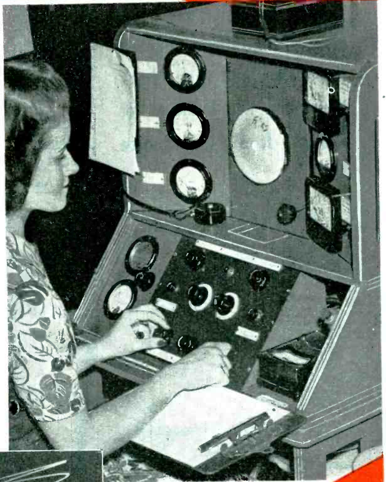
Uniformly bright spot on screen of 15-CPI cathode ray tube in test set indicates perfectly formed cathode.
