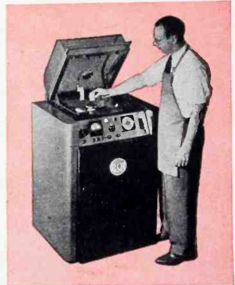
• This is the new RCA 2000-watt electronic generator especially designed for the plastics industry and other applications requiring power at frequencies up to 27 megacycles.
