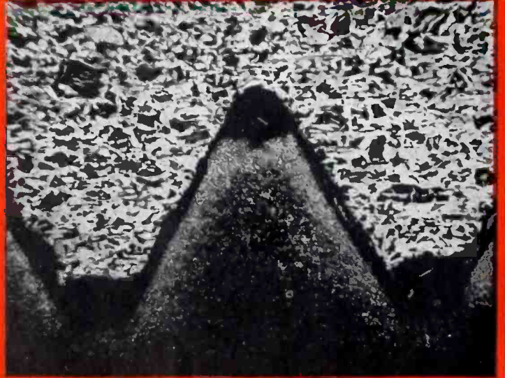
Decarburization of bolt satisfactory. Thread form good. Heat treatment slightly deficient. Nut satisfactory.
