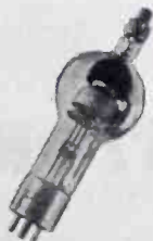
PHANOTRON — for high-frequency electronic heating
