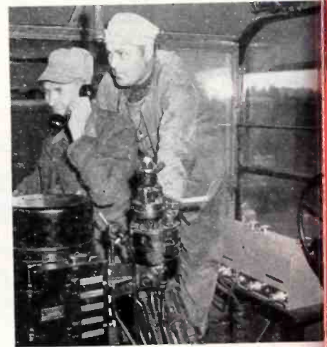
On approaching the railroad yards, train crews can now receive instructions from the train dispatcher via Motorola f-m equipment mounted behind the engineer
