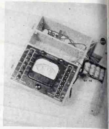
In this push-button test kit, standard battery types BA-42 and BA-59 are shown in relation to their means of connection. This unit is part of test set IE-10
