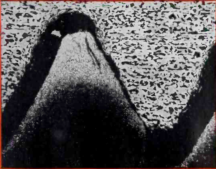
This photograph shows somewhat excessive decarburization in the bolt, and a lap in the thread. Nut is satisfactory. Heat treatment O.K.
