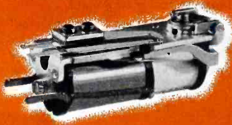
ABOVE—Type 107—Time delay relay of the slug type. Pure copper slug on heel end of core provides maximum of 300 milliseconds delay in contact opening after circuit is broken.
