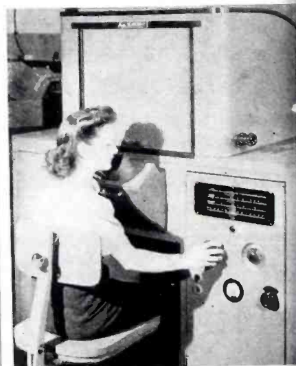
Rayproof and shockproof. A girl operator adjusts the controls of the Norelec Searchray model 150. Made by North American Philips Co., the unit has a built-in indirect fluoroscope and a potential limit of 150 kvp
