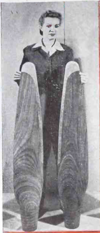
PANELYTE Compreg Propeller Blades — rotary cut veneer impregnated with phenol-formaldehyde. It possesses extremely high tensile, compressive and flexural strength. Carving is done by Engineering Research, Riverdale, Md.
