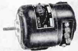
Type "B" A.C. Generator Permanent Magnet Field wound for one, two or three phase A.C. Ball-bearing equipped; flange or base mounted. 2 1/4" outside diameter . . . weighs 16 ounces.
