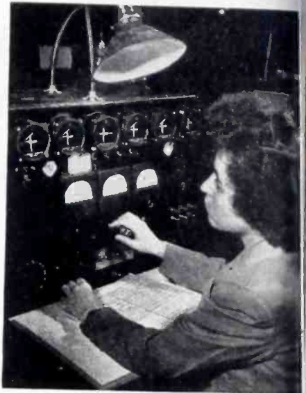
Cross pointer indicators for blind landing of aircraft are checked in the Westinghouse Meter Division at Newark, N. J. The instruments operate on a current change as small as 12 microamperes.
