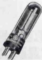
PHOTOTUBE — for counting, sorting, grading
