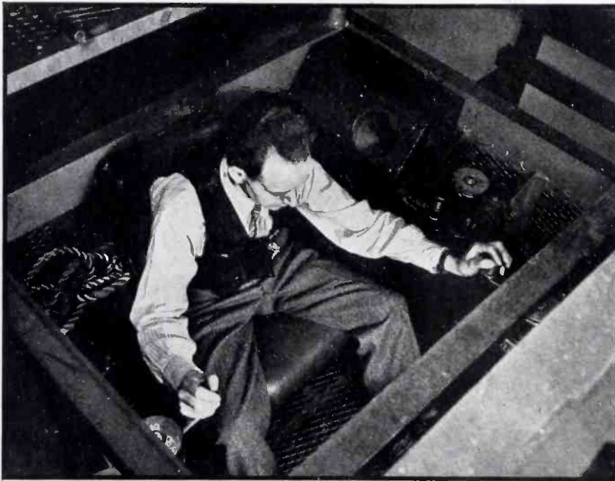
Experimental model of special-design receiver for carrier-current signal reception fits into the corner of a crane cab at plant No. 2 of GM's Fisher Cleveland Aircraft Div. At the controls is R. B. Jones, who had charge of construction and testing on the installation
