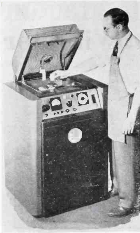
In the photo above, the operator is shown placing a preform on the lower electrode. When the mesh cover is lowered, the upper electrode makes contact with the plastic material. The cover pops open and power is shut off at the end of a predetermined heating interval
