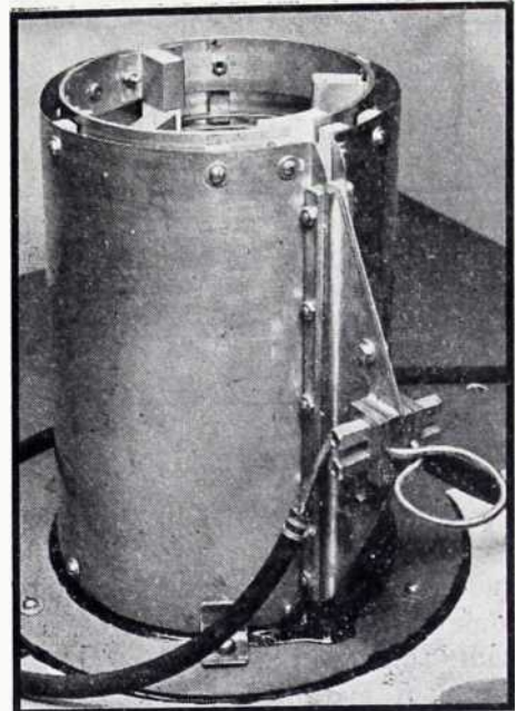
FIG. 17—A current transformer which is useful for inductive heating
