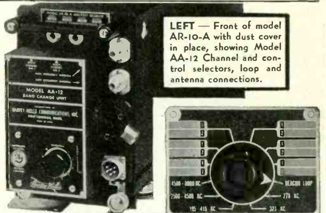
RIGHT — Close-up view of model AA-15 Electric control unit for remotely controlling all-functions of the AR-10-A Receiver. A separate manual timing unit is also provided.
