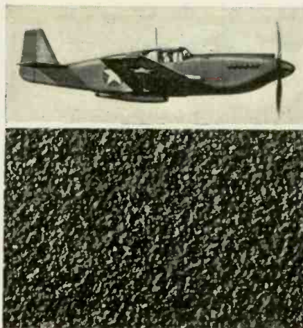
On the steps, catwalks, and cockpit floors of military aircraft, a covering that will withstand wear, yet be skid-proof, is absolutely essential. Rubber is slippery when wet. Other materials wouldn't stand the abuse. The Western States Lacquer Company developed an abrasive coating, particles of hard aggregate suspended in a rubber-like BAKELITE Plastic base. Sprayed or troweled on, this new coating gives a resilient, sandpaper-like surface to the flooring of some of America's leading bombing and fighter planes.
