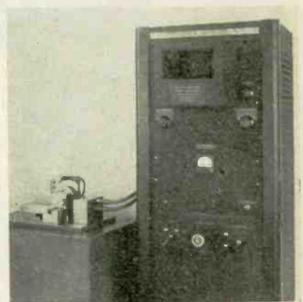
Test jig and control cabinet of the Electrodynamicoscope, a machine for dynamic balancing of gyro rotors by electronic measurement of centrifugal forces
