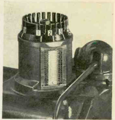
The preselector dial drum that automatically figures the gear ratios and speeds in the use of a No. 5 Warner & Swasey turret lathe was formerly made of metal. It is now molded of a BAKELITE General Purpose Phenolic Plastic eliminating several machining operations. The conversion has meant an important savings of metal and a reduction in production costs of approximately 80 percent.
