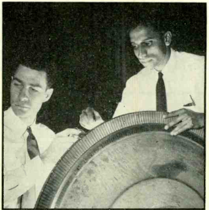
FIG. 5—The crystal vibration detector is moved along the wheel while the operator watches a nearby oscilloscope. Points of peak vibration are marked on the wheel
