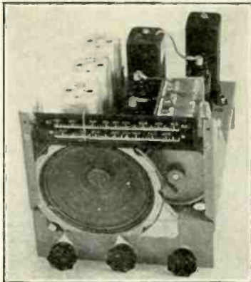
Series 6 tunable receiver. 2 band model illustrated, range 550-4000 K.C.
