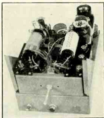
Series 20, 4 channel 1600-6000 KC, 20 watt transmitter.
