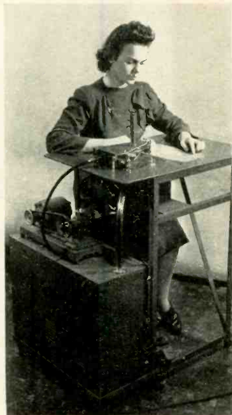
This induction heating machine, developed by RCA for use by the plastics industry, is popularly known as a radio sewing machine. The diagram shows how the two wheels act as electrodes
