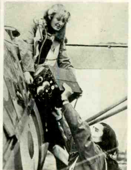
The personnel of the Women's Royal Naval Service are expert radio mechanics. This photo, taken at a Royal Naval Air Station in south England, shows a transmitting instrument being fitted into a plane. The girls are taught to tune in radio instruments
