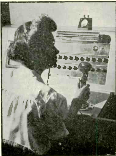
CONTROL PANEL—Director of Broadcasting Marie Kabrynez, seated at radio station type console containing a tuner, two turntables, necessary volume controls and channel switches
