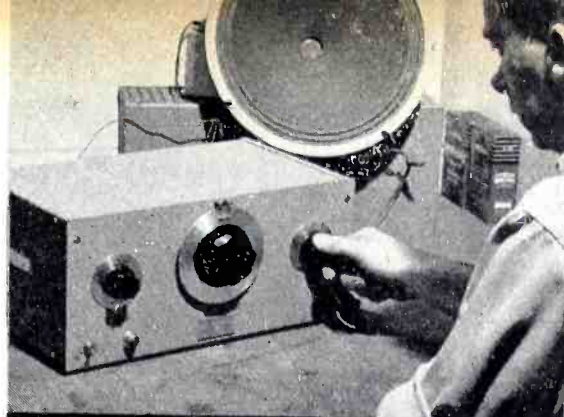
Audio frequency oscillators of the resistance-tuned type. Excellent frequency stability and freedom from wave form distortion. Model 2008 Resistance-Tuned Oscillator above
