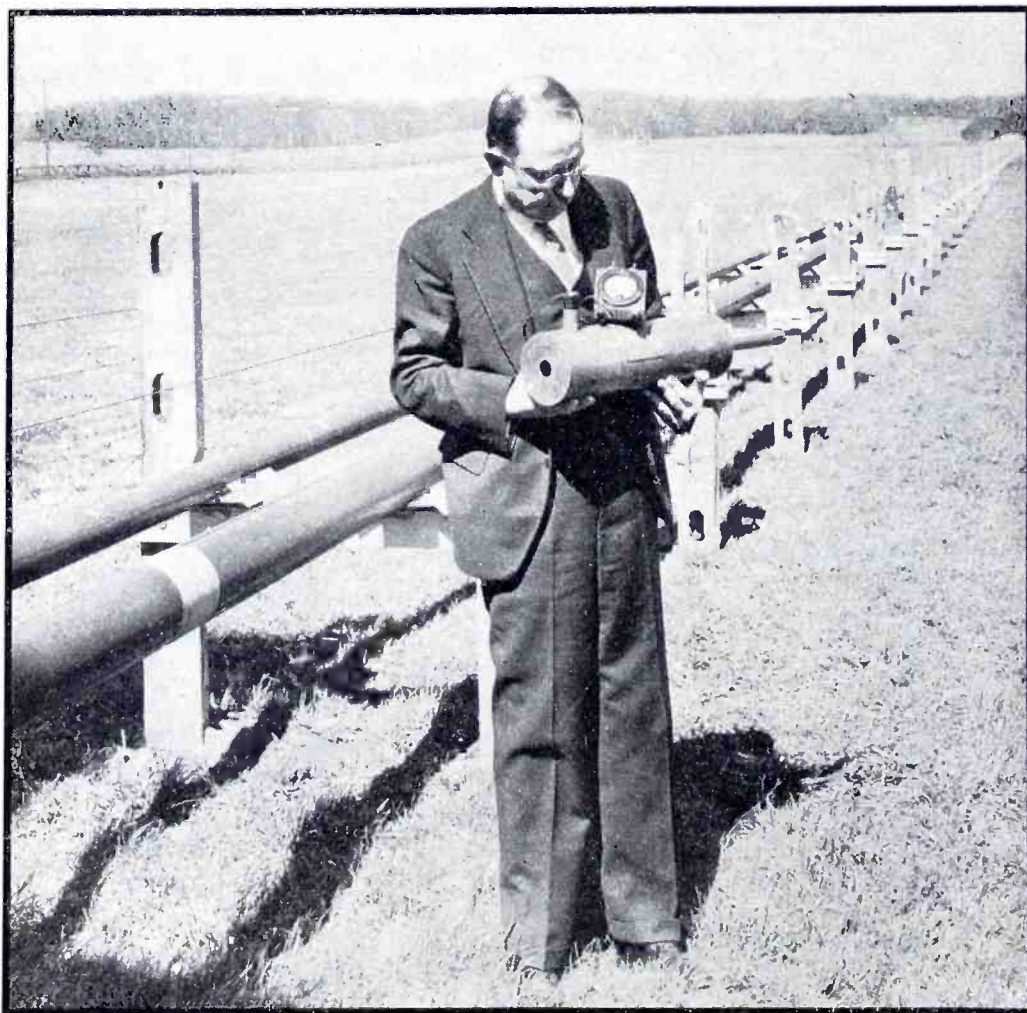
WAVE GUIDE —G. C. Southworth, holding one of the resonant chambers used for tests of wave guide transmission. Behind him are two experimental wave guide transmission lines at the Holmdel Station of Bell Telephone Laboratories
