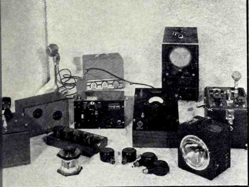
INSTRUMENTS —Typical commercially available devices in use at ETL. Sound level meter, stroboscopic tachometer, cathode-ray oscilloscope, vacuum tube voltmeter, amplifier for power frequencies, susceptance-variation circuit, bridge and wavemeters
