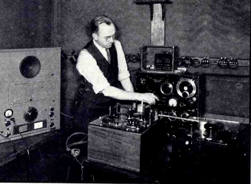
UHF—Measuring equipment in double-shielded room at the Electrical Testing Laboratories. Left—radio receiver; center foreground—Schering bridge; center at rear—radio frequency signal generator; right—quartz-insulated standard air capacitor
