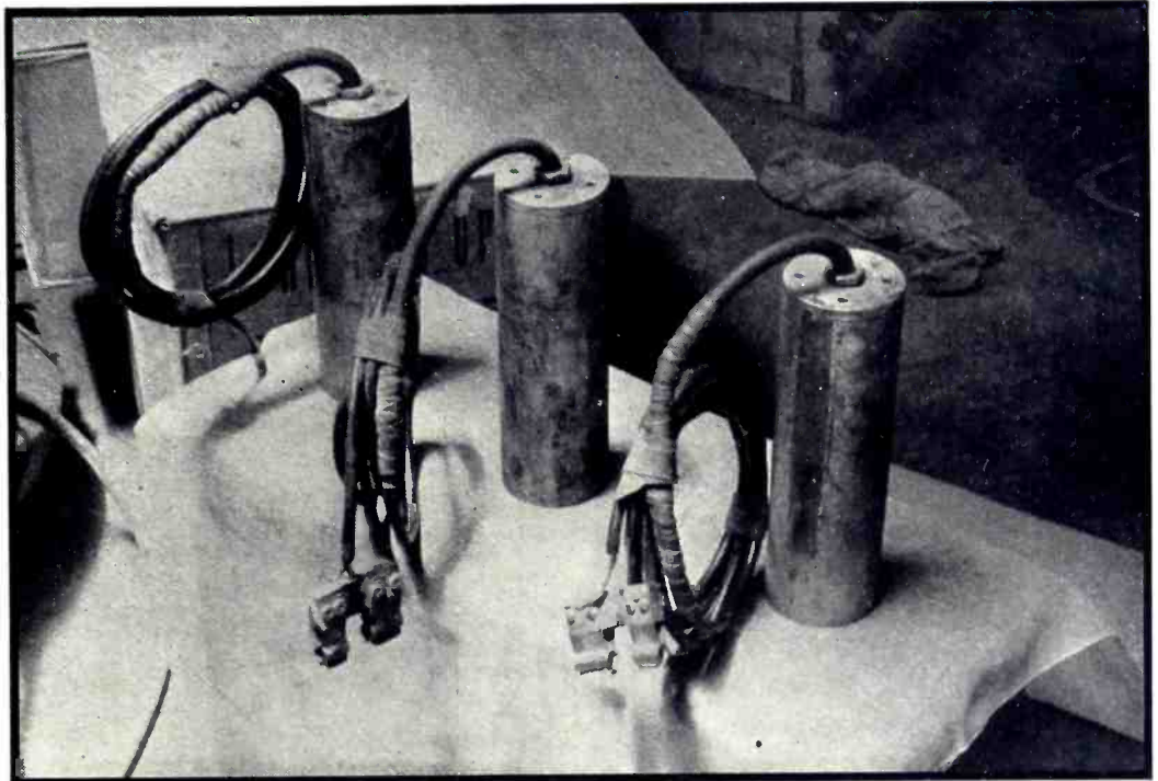
PICKUP —Seismic pickup of the variable-reluctance type. At a frequency of 45 cps and a ground movement amplitude of one millionth inch, this device will deliver approximately one-half millivolt to the grid of the first amplifier, through the appropriate transformer
