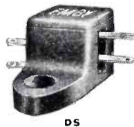
Input 10 volts. Full wave Bridge. Continuous dc 10 ma. Unbreakable plastic case with mounting extension.
