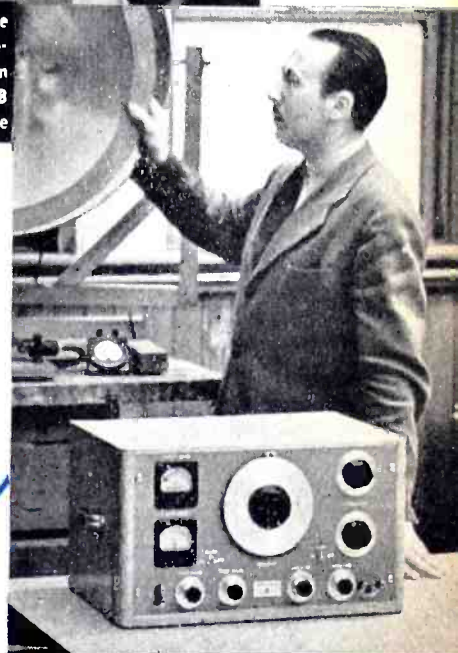
Audio signal generators providing standardized voltage throughout the audio frequency range. Model 205AG Audio Signal Generator above
