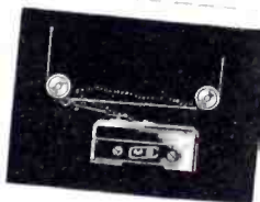
This illustration shows a Micro Switch enclosed in a die cast housing with a synthetic rubber seal, and is being used as a lathe carriage stop.
