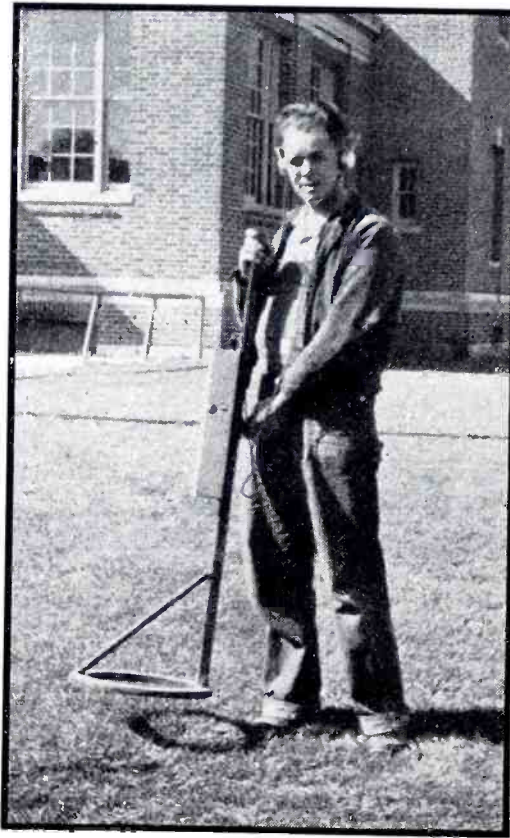
DETECTION—Metal locator, equipped with an electronic amplifier. It facilitates the finding of buried pipe lines and valves
